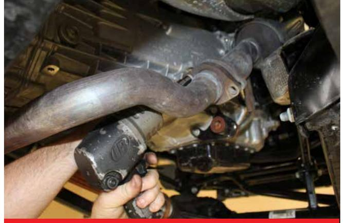
**B.** Remove fasteners from right and left sides.
