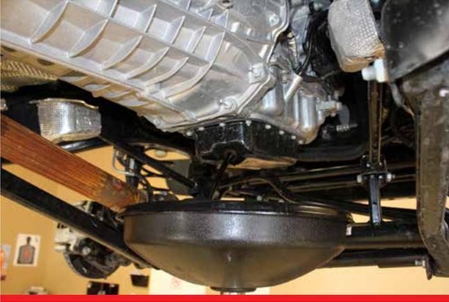
**A.** Drain the engine oil from the vehicle and tighten the drain plug.
