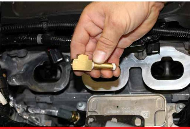
**C.** Apply Teflon tape to extension on both sides and insert into T-fitting as shown.
