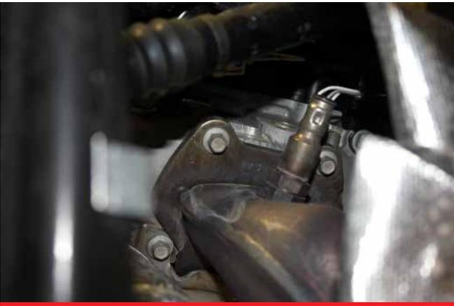
**D.** The cat equipped pipes are a wedged flange design. Remove the top 2 bolts and just loosen the lower 2.
