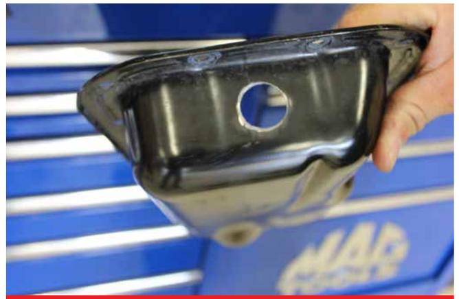
**E.** Using a hole saw, drill a 7/8" hole as shown. Clean any burrs so surface is flat.
