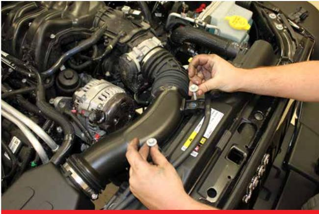
**A.** Remove entire factory air intake system including lower box portion under air filter.
