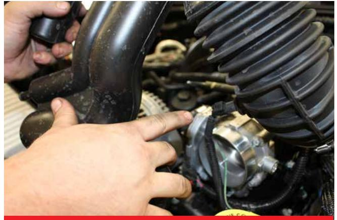
**B.** Remove intake air temperature sensor for later use.
