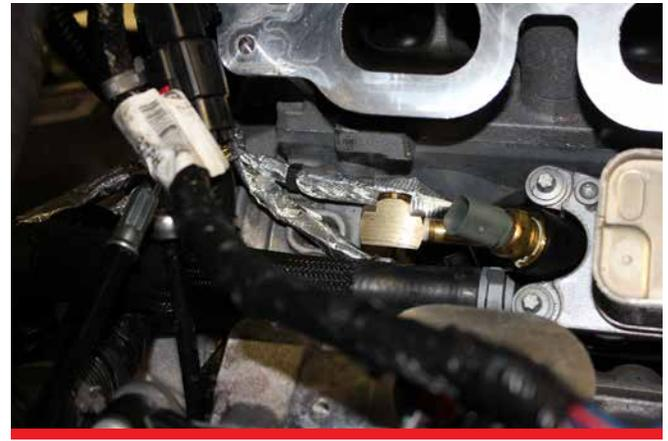
**D.** Install extension and T-fitting where oil pressure switch was removed and tighten.
