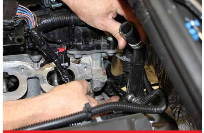
**B.** Disconnect 2 electrical connectors and remove oil pressure sensor.
