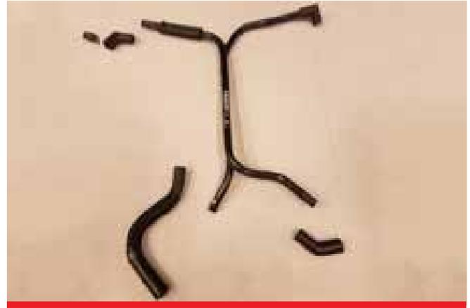
**B.** B. Remove the 3 hose ends as shown here.
