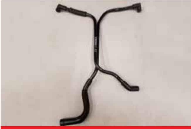
**A.** A. Remove the factory PCV lines shown .
