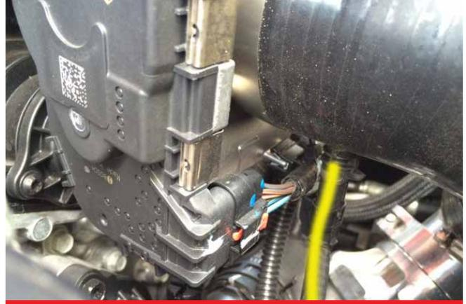
**A.** Install throttle body silicone and intake air temperature sensor in pre-punched hole on underside of hose going to throttle body
