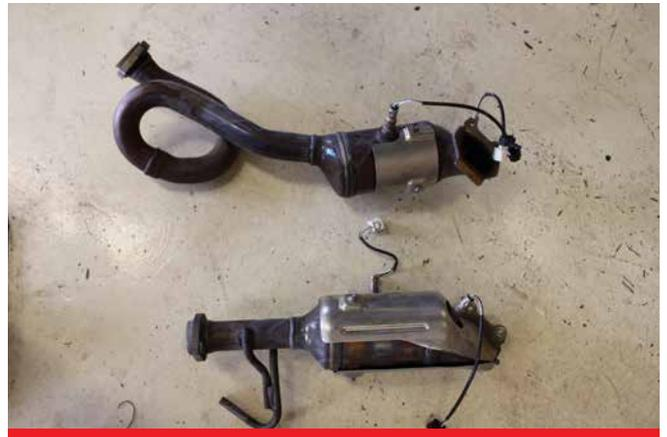
**E.** Remove left and right cat equipped pipes.
