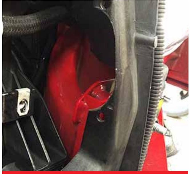
**D.** Clearance core support on both passenger and driver side for silicone hoses as shown.
