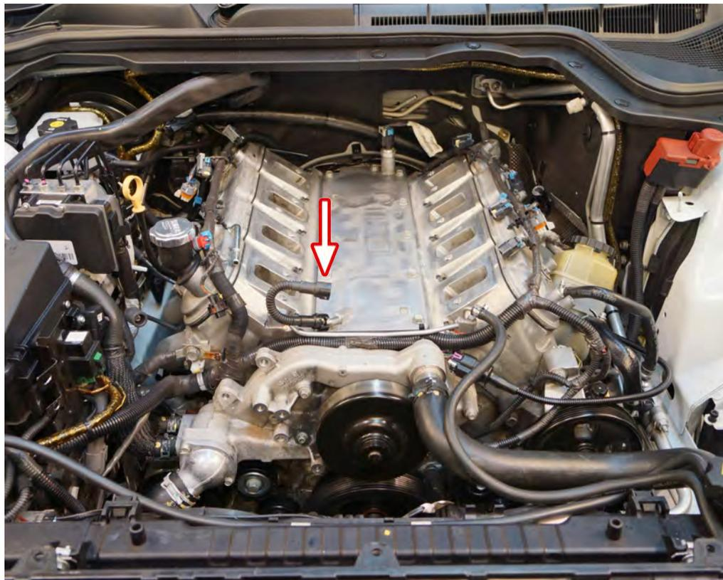
62 With assistance lower the supercharger manifold on to the engine.
