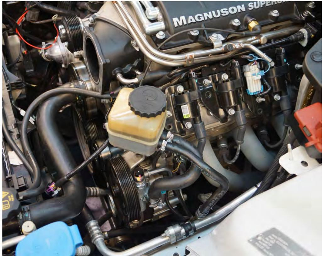
92 Fit the throttle body to the adaptor using the factory throttle body bolts kept from step 24. Plug in the throttle body extension harness.
