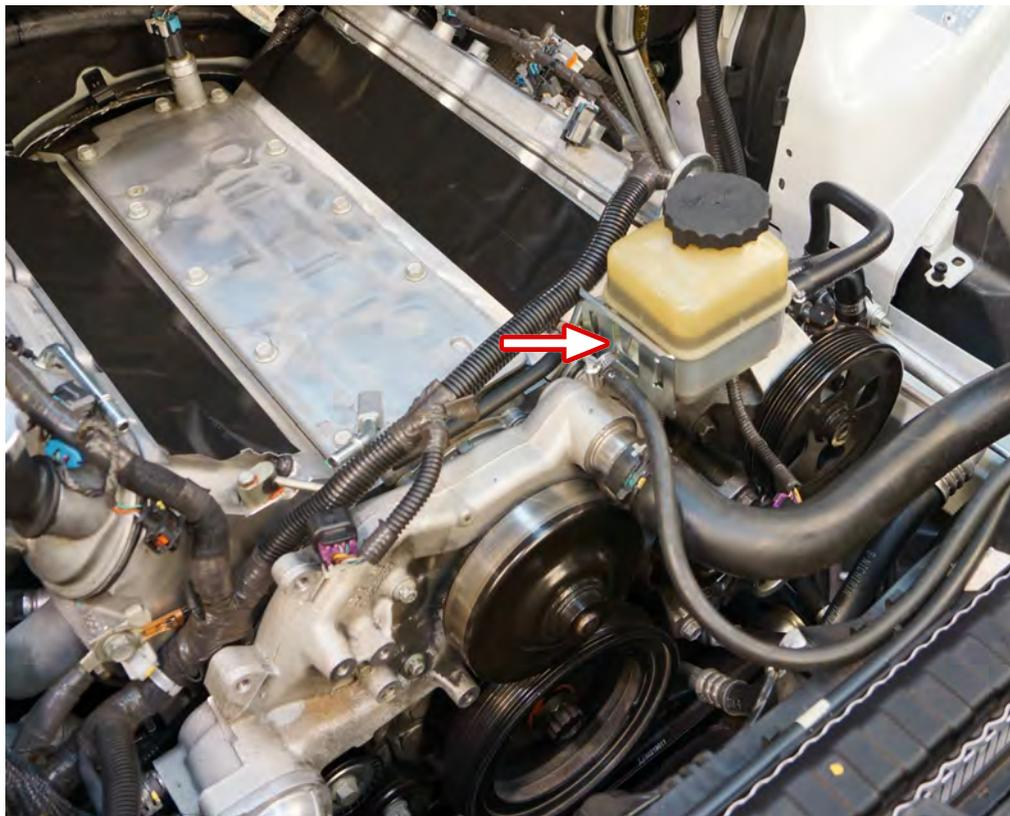
32 Remove the 2 x 15mm bolts holding the power steering bracket in place and then remove the bracket. Keep 1 of these bolts for step 88.
