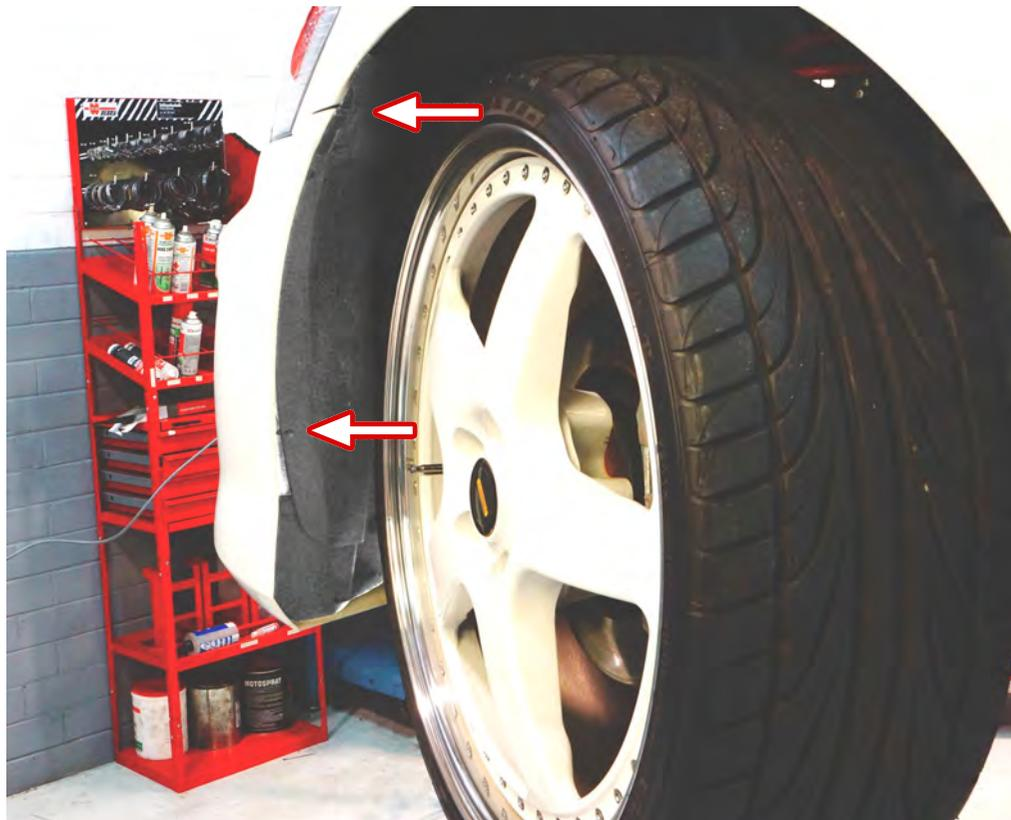
38 Remove the 3 x T15 Torx screws along the edge holding the guard liner to the front bar.
