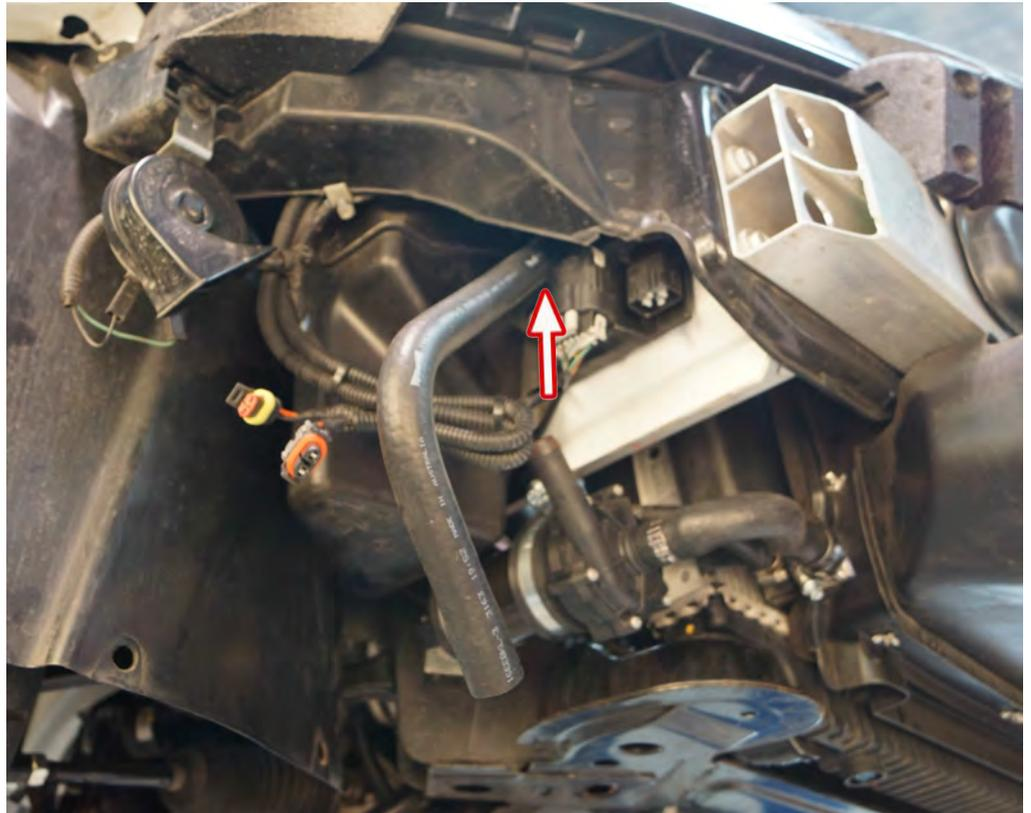
123 Clamp the short end of the cooler hose to the pump using the supplied clamp as shown.
