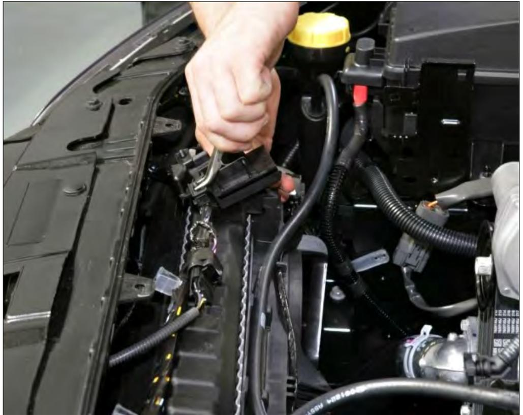
15 Disconnect the wires connected to the lower support before removal.
