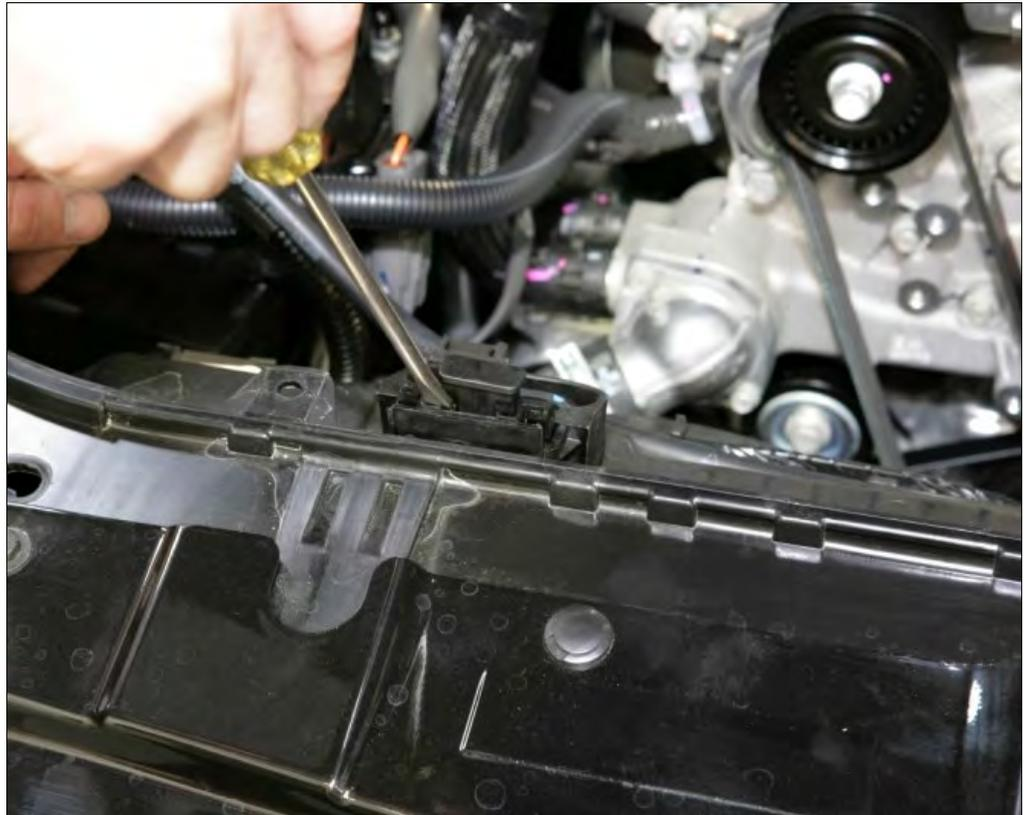
9 Lift up the top part of radiator support and then remove.
