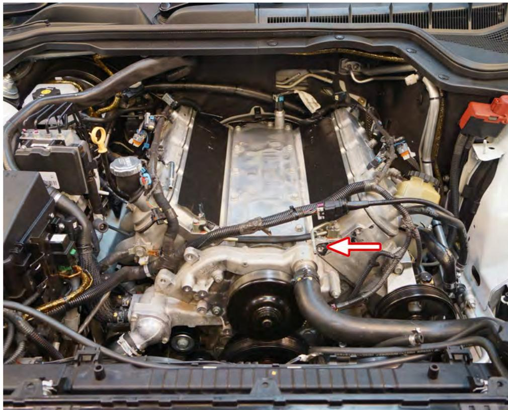
57 Remove the factory steam pipe by removing the 2 x 10mm bolts holding it to each head. Keep these bolts as these will be used in step 58.
