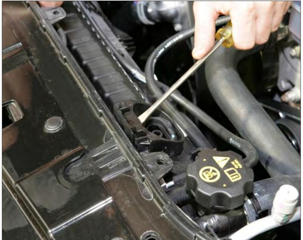
8 Lightly raise locking wedge out of position to free the radiator support.
