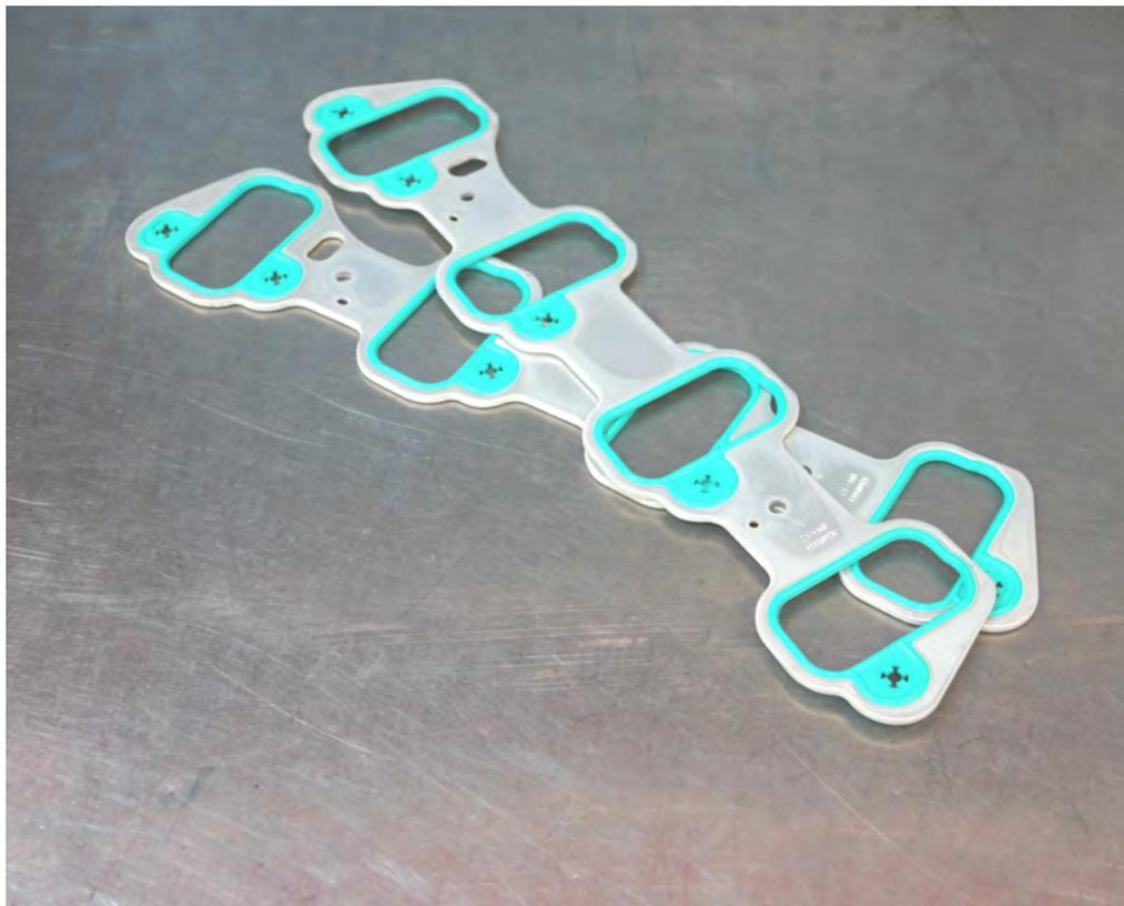
52 Place the manifold gaskets to the supercharger manifold using the manifold bolts pushed through the gaskets to help hold them to the manifold.
