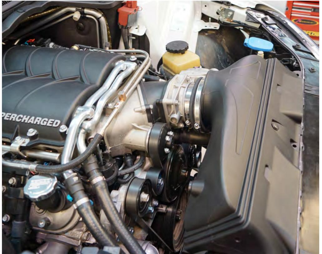
142 Secure the OTR to the radiator support using the three push clips supplied in the OTR fitting kit.
