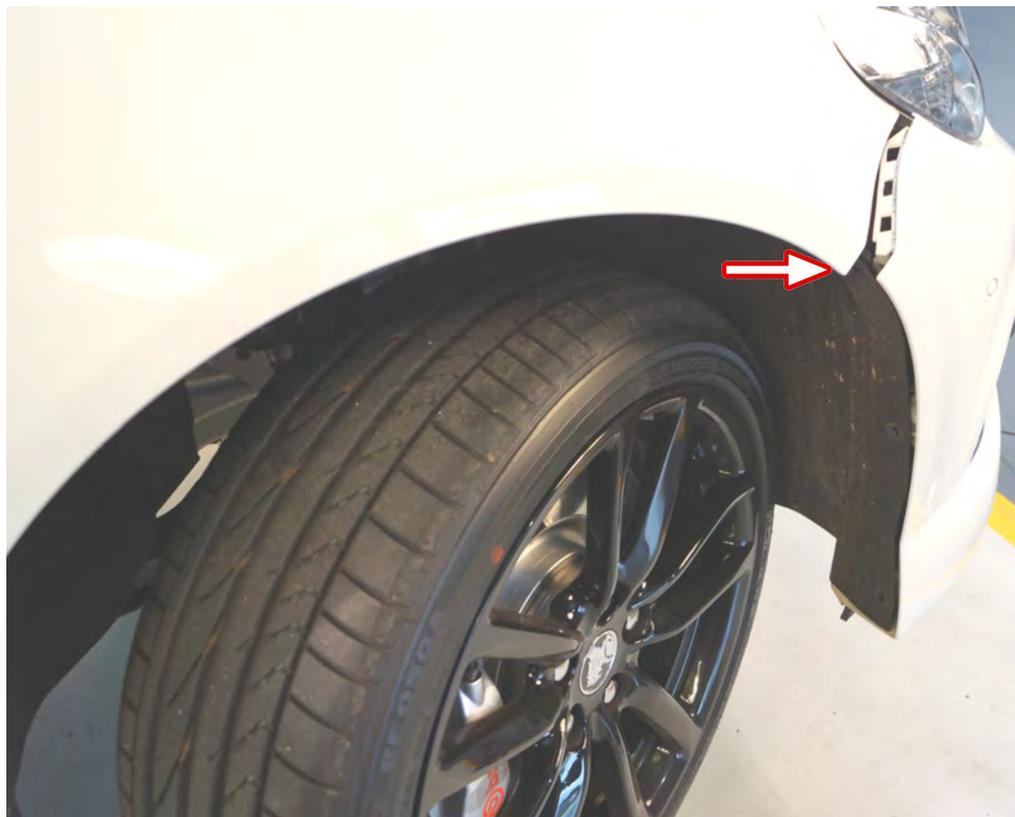
41 Undo the 5 x 13mm bolts holding the lower tray to the vehicle.
