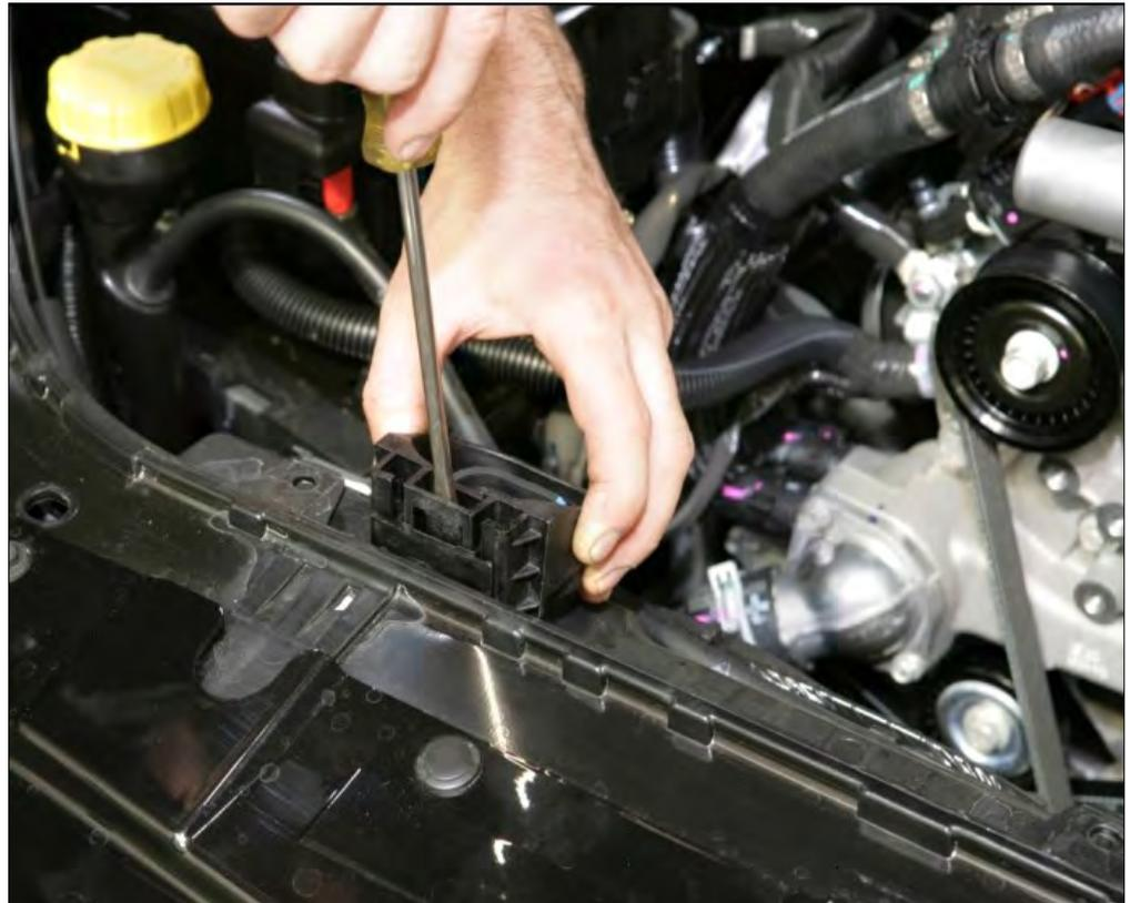
10 Remove the 10mm retaining bolts.
