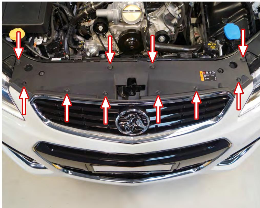
35 Remove the 4 x screws on the bottom edge of the front bar.
