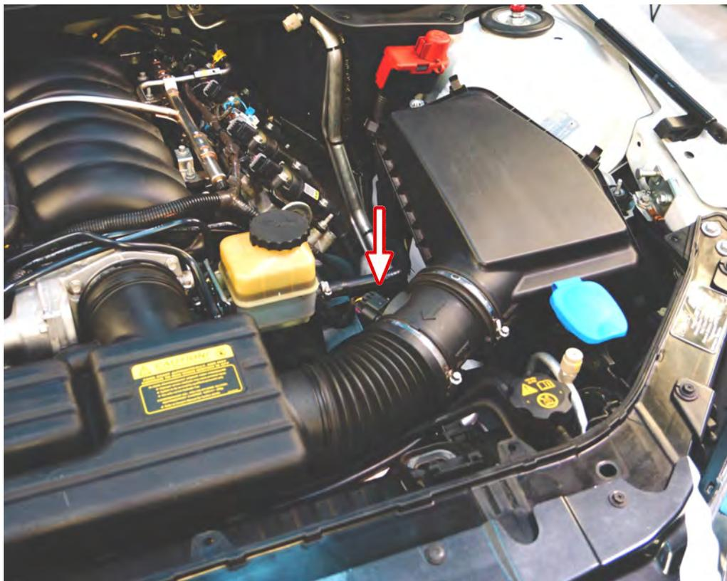
3 Remove the rocker breather from intake pipe and the rocker cover.
