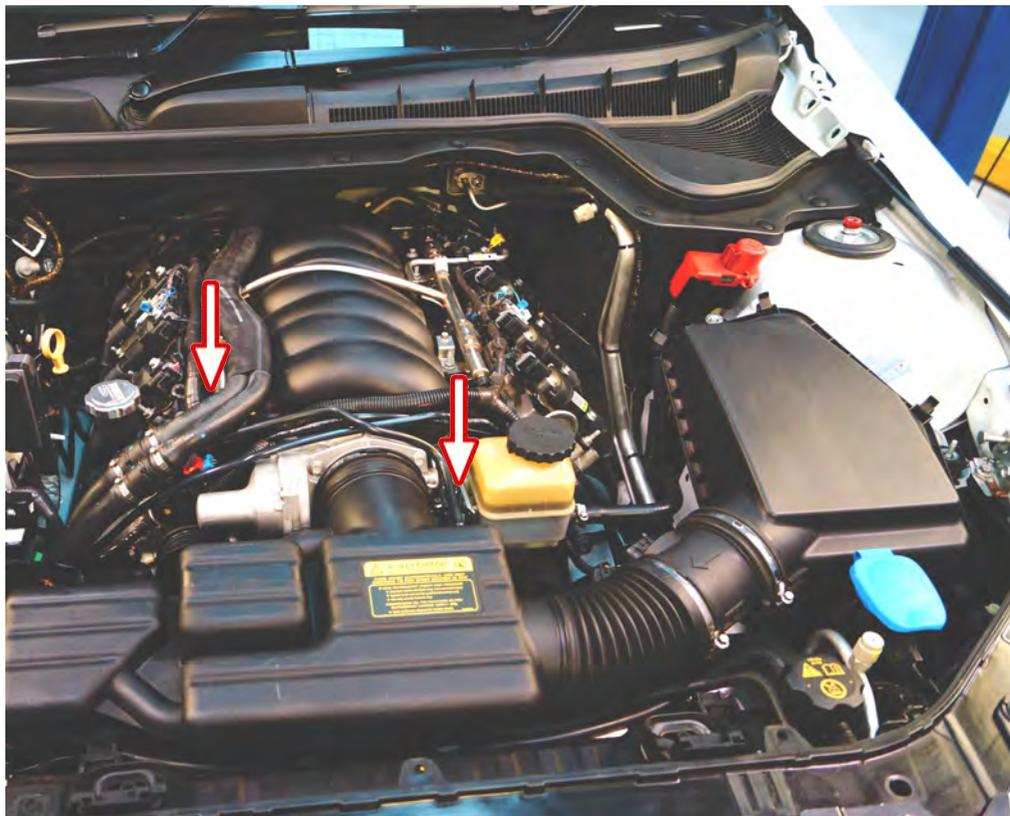
4 Loosen the 2 hose clamps as pictured and then remove the intake pipe.
