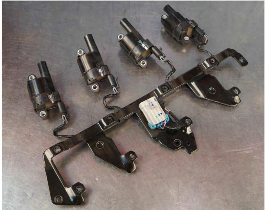
76 Slide off the main coil harness connector from the bracket.
