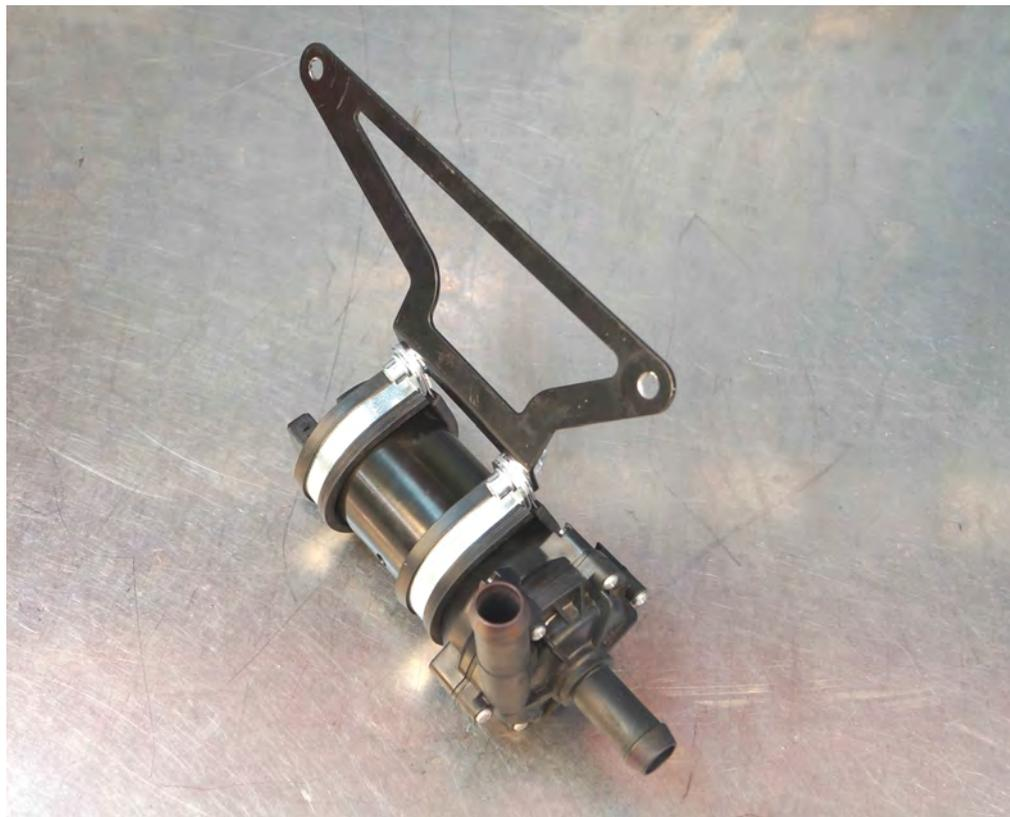
118 Note the orientation of the pump outlets in relation to the bracket. Tighten the clamps once it is in this position.
