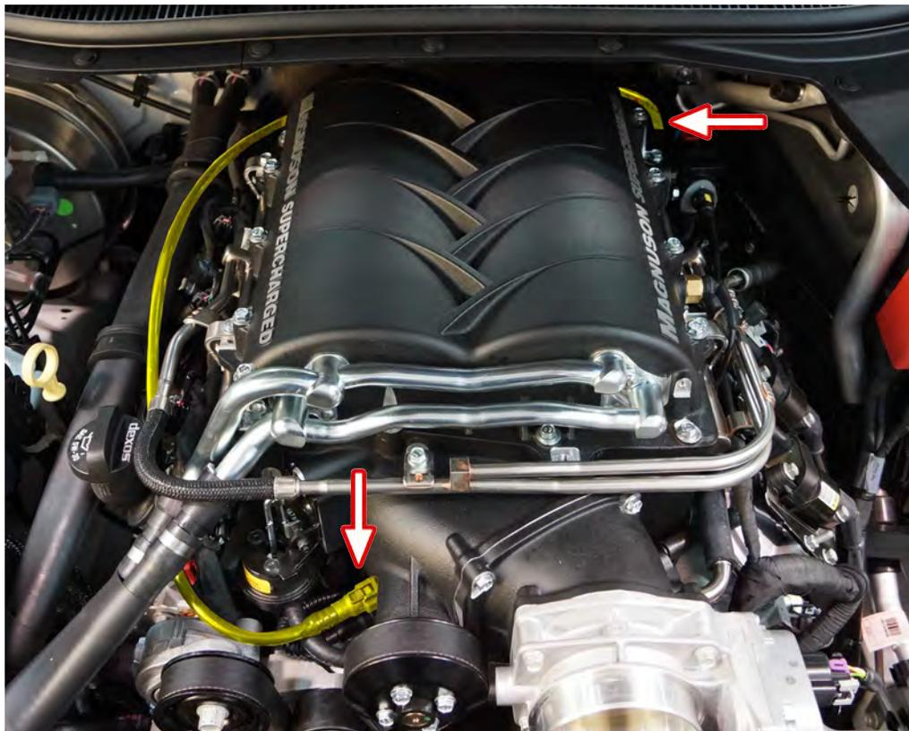
87 Remove these 2 x 15mm front power steering pump bolts. These will be used in step 88.
