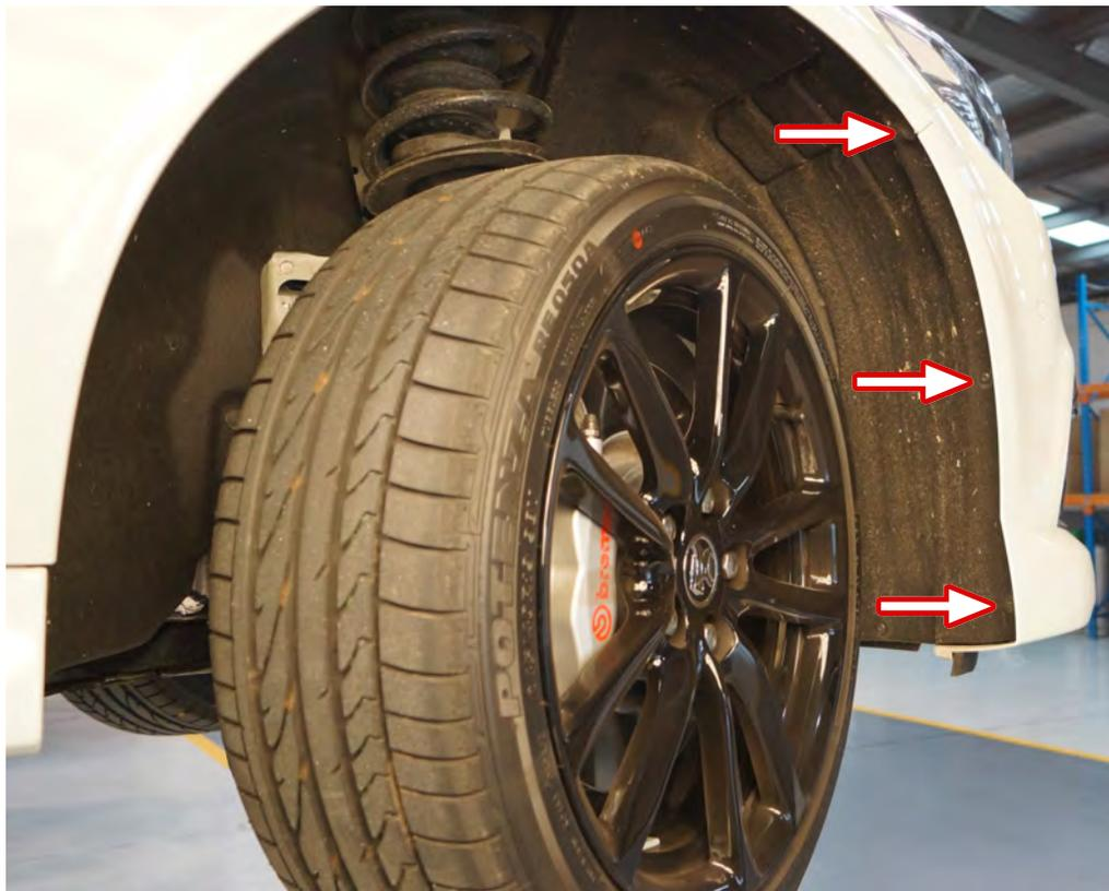
39 Pull the guard liner back and using a 10mm socket on a long extension. Loosen off the 2 x 10mm bolts holding the bar to the front quarter panels.
