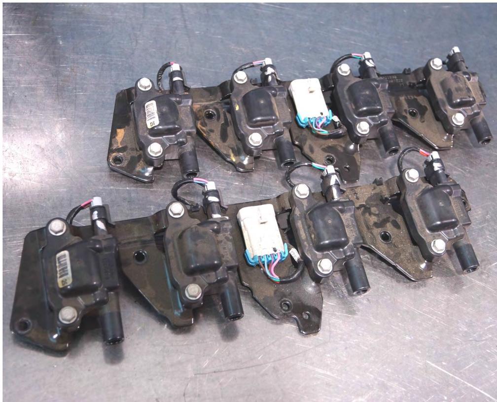
75 Start by removing each of the coils from the bracket by removing the 2 x 10mm bolts holding each coil in place.
