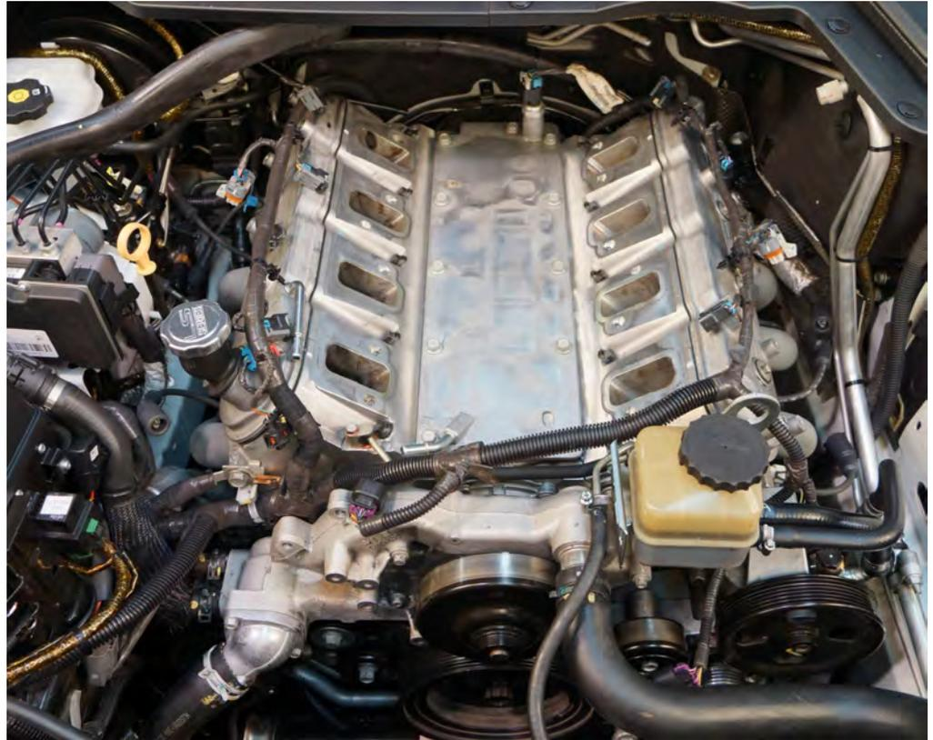
30 To prevent debris entering the intake ports whilst the next series of steps are completed, cover the intake ports with tape as pictured.
