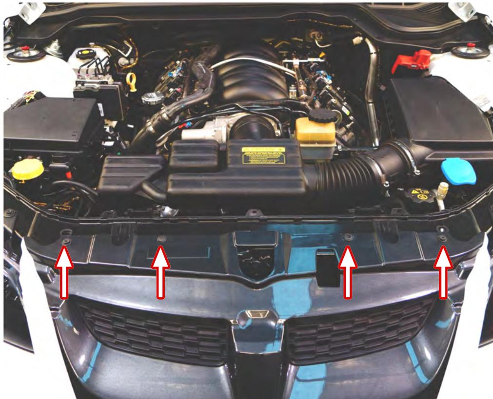
34 Remove the 4 x 10mm bolts and 6 x T15 Torx screws from the top of the bar on the radiator support panel.
