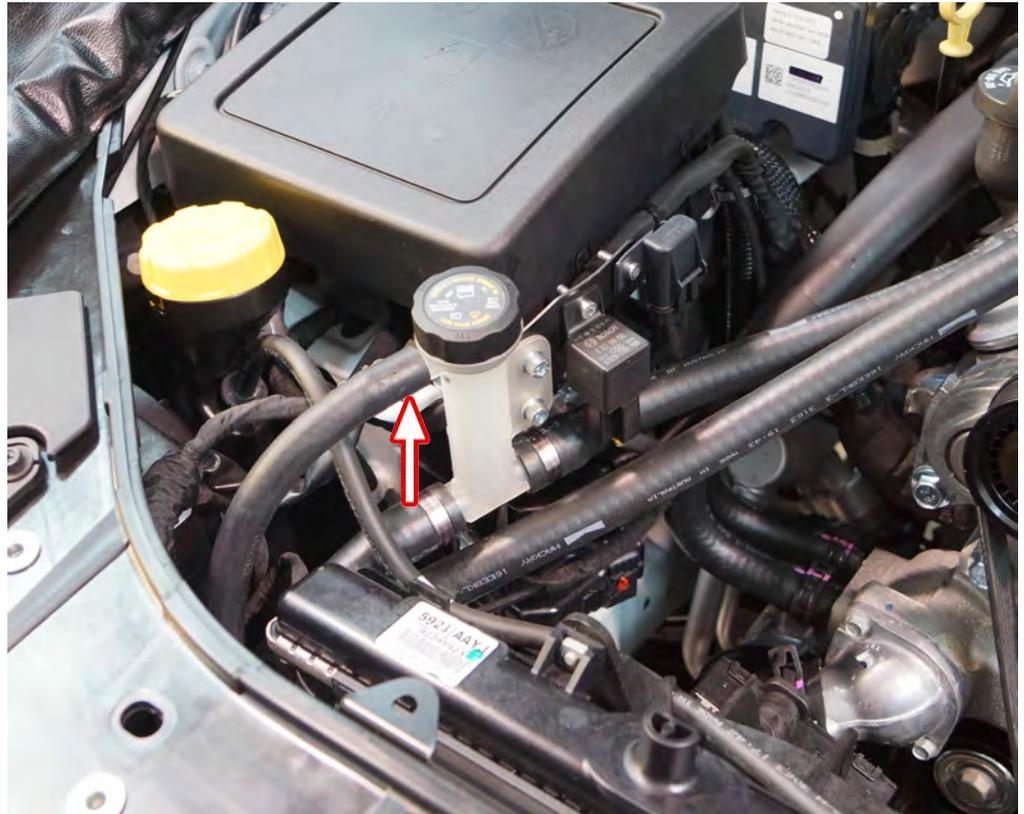
134 Connect the cooler hose from the de-gas bottle to the upper supercharger cooler pipe.
