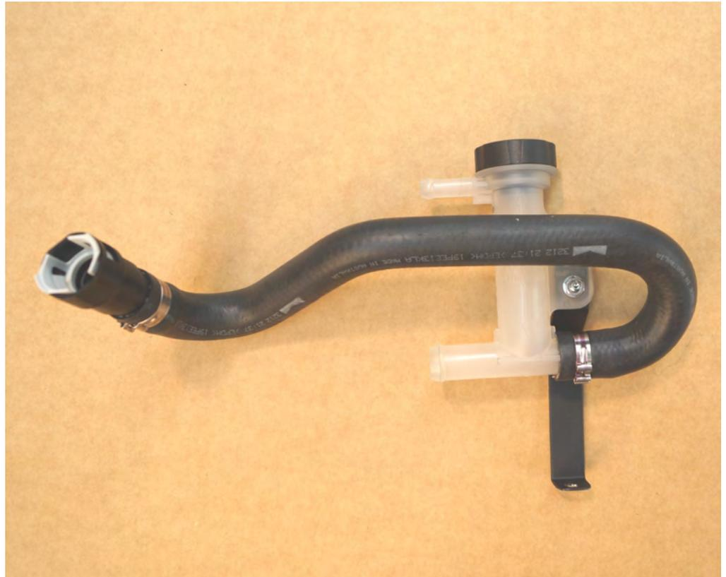
129 Mount the fuse and relay to the de-gas bottle bracket, and loosely mount the assembly into position. Once in position determine the correct length of hose coming from the top LTR to connect to the de-gas bottle barb (horizontal arrow). The excess from this cut will be used to connect the de-gas bottle to the supercharger (vertical arrow) in step 131.
