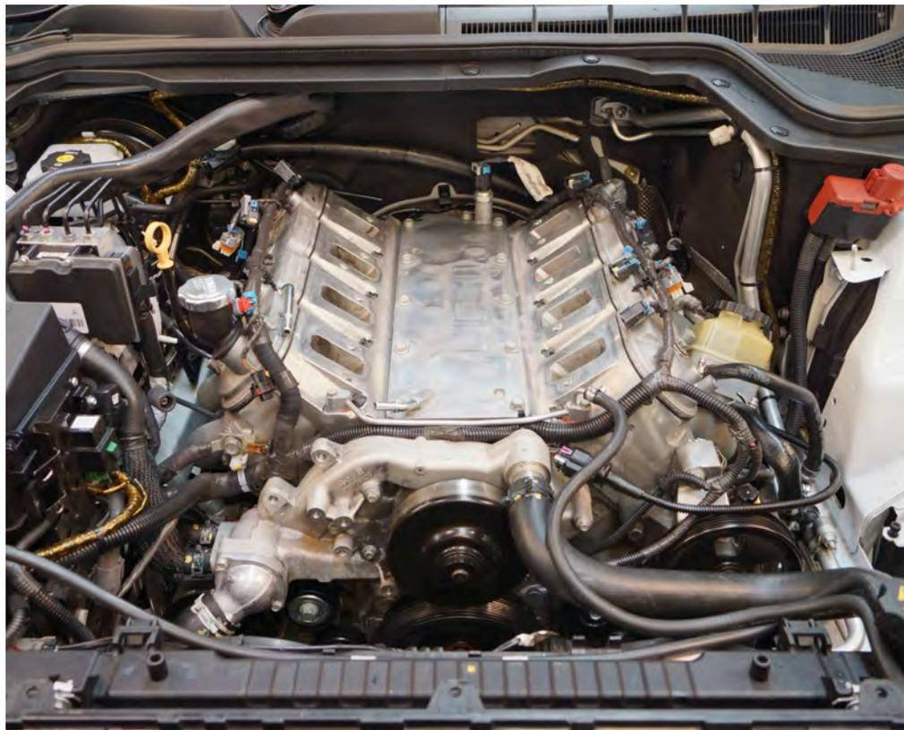
61 On non-DOD engines, refit the factory valley plate breather as shown.
