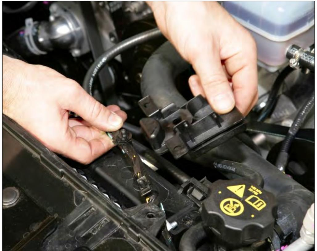
16 Remove the standard drive belt by releasing the tensioner.
