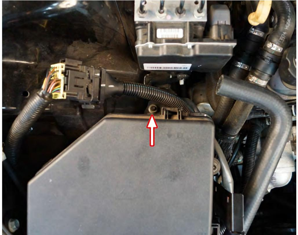
127 Fit the de-gas bottle bracket to the fuse box as shown. This bracket will also have the fuse and relay mounted to it.
