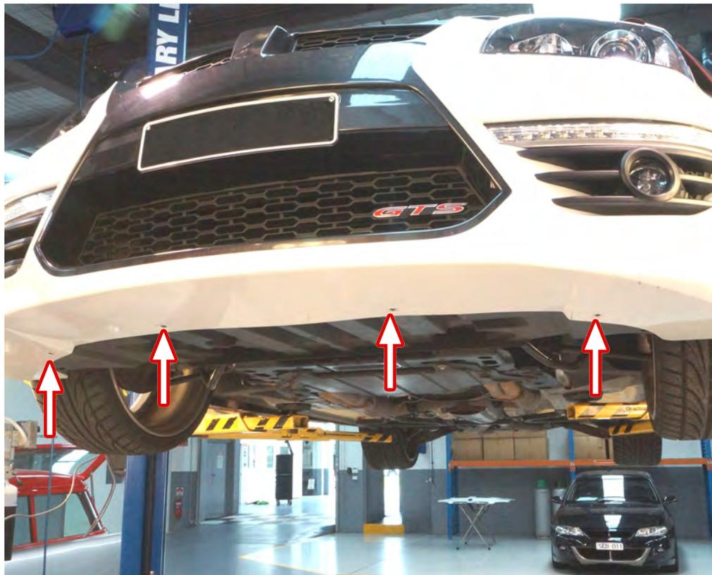
36 Remove the 5 x 13mm bolts and 11 x T15 Torx screws on the bottom edge of the front bar.
