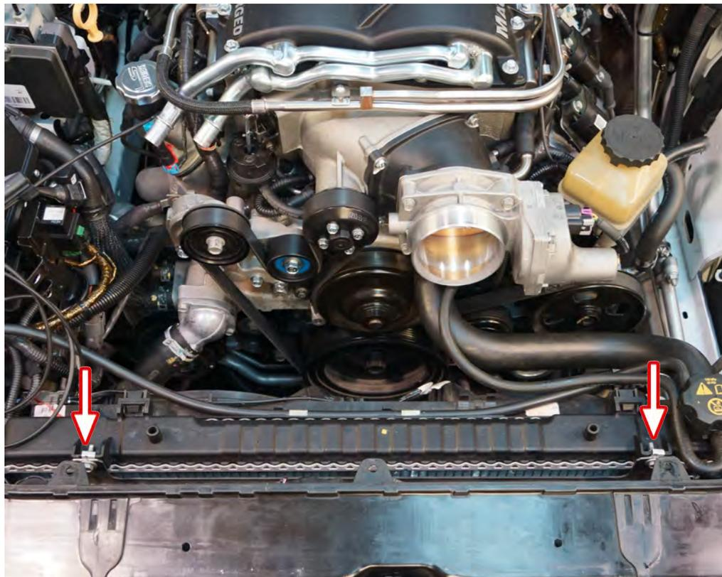
100 Remove 6 x 10mm trans cooler bracket bolts. These bolts will be used again in step 102.
