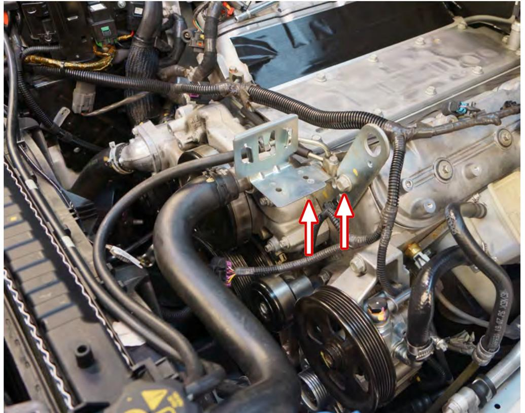
33 Remove the 2 x push clip scrivets and the 2 x 10mm bolts from the top of the bar on the radiator support panel.
