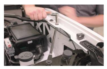
40. Remove the two upper-forward, diagonal fender-brace bars using a 10mm wrench.
