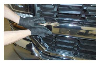
36. Pull straight out on the fascia/grille to disconnect the two remaining snap clips at the center of each side, and the bottom guiding slots. Set the fascia/grille aside carefully for later reinstall.
