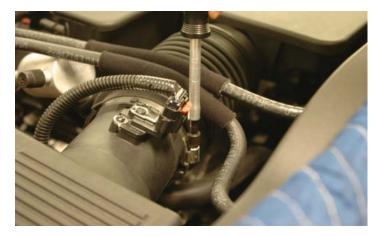
7. Loosen the clamp at the air box securing the air plenum in position.
