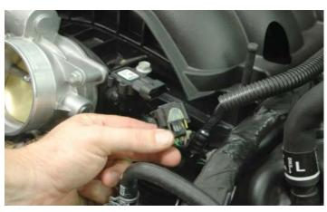
14. Unplug the electrical connector from the MAP sensor. Release blue locking tab first.
