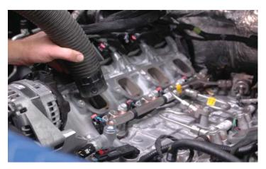
28. Use a shop vacuum to clean off the heads being careful to not allow any debris to fall into the exposed intake ports.
