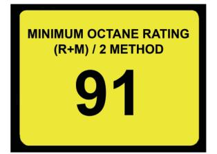
3. Your system requires the use of minimum 91 Octane gasoline fuel. This system is not compatible with E85 fuel.
