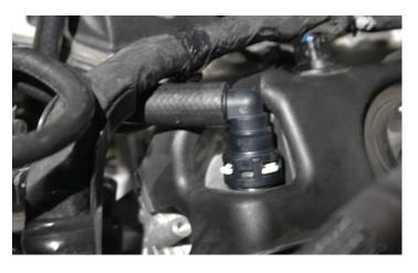
152. Connect the 90° hose barb on the uncovered side of the PCV hose to the left hand side front of the valve cover hose barb. Route the hose under the supercharger inlet toward the right hand side of the vehicle. The split loom covered section of the hose should be on the right hand side above the alternator.
