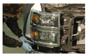
84. Reconnect the harness plug to the right side headlight removed earlier and replace the headlight using the OEM fasteners.
