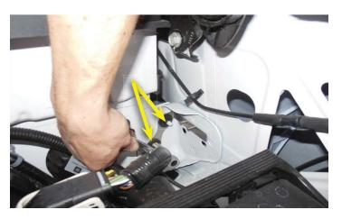
120. To install your intercooler pump harness bracket, begin by removing the two nuts with a 13mm socket where the left hand inner fender meets the firewall. This will be behind the fuse center, below the hood hinge. Place the supplied pump harness bracket onto the studs and use the factory nuts to secure it in place.
