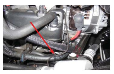
144. Route the MAF/IAT breakout behind the alternator. Make sure the harness will not get pinched by the alternator. Use a tie wrap to secure the harness to the factory heater hose as shown by the red arrow to the left.
