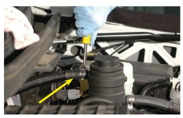
118. Connect the left side hose coming from the supercharger charge air cooler to the upper-rear hose barb on the intercooler reservoir using a provided worm gear clamp. It's important to utilize only worm gear clamps on the charge air cooler reservoir.
