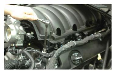
23. Use a 10mm socket wrench to remove the ten bolts securing the OEM intake manifold to the heads. The intake manifold is now ready for final removal from the vehicle.
