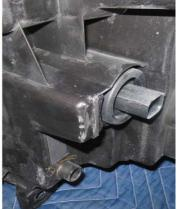
83. On the right side headlight assembly removed earlier near the electrical connection there is a tab (highlighted in green on the left photo) that needs to be removed for hose line clearance. You can use a cutoff wheel to cut this tab off. The photo to the right shows the tab removed.
