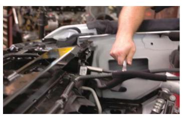
54. Replace the upper radiator mounting bolts and vibration dampers.
