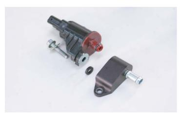
134. Mount the OEM EVAP solenoid to the provided mounting bracket using the factory mounting bolt and provided spacer using a 10mm wrench as shown. Add blue Loctite 242 to this fastener.
