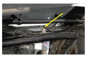
132. Connect the black ground wire "eye" terminal to the existing grounding bolt at the firewall on the left hand side, just above and inside the brake booster canister.
