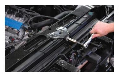
53. Replace the upper radiator cross-frame brace and secure with the OEM mounting bolts.
