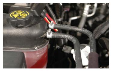
159. If you disconnected the reservoir overflow hoses earlier, reconnect using the OEM clamps.
