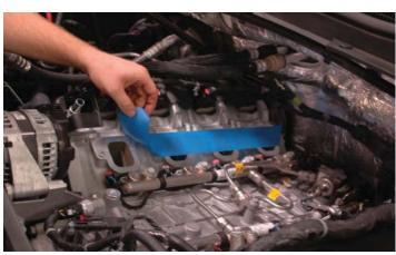
30. Use tape or clean shop towels to cover over your intake ports. It's important to keep these ports clean and avoid any debris falling into the exposed openings.
