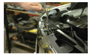
163. Replace the four bolts holding the top of the fascia/grille to the sub frame using a 10mm wrench.
