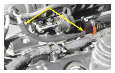
137. Connect the provided 10" x 3/8" PCV hose between the EVAP solenoid and the supercharger inlet hose barb. No clamps are required. Adjust hose length to prevent rubbing on supercharger bolt head.
