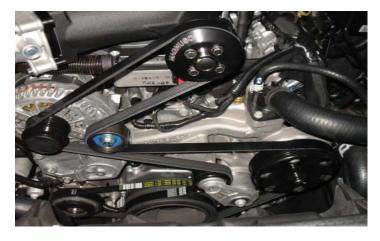
116. Install the provided accessory drive belt using the drive routing diagram. A larger diagram is included at the back of this book.
