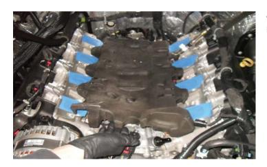
89. Install trimmed insulator from last step into manifold valley.
