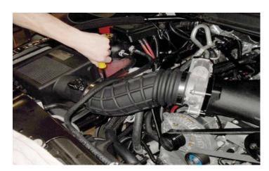
157. Tighten the hose clamps on both sides.
