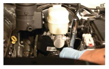
64. Replace the nuts incorporating the reservoir assembly. Torque to 33 ft-lbs. Verify your torque wrench settings.
