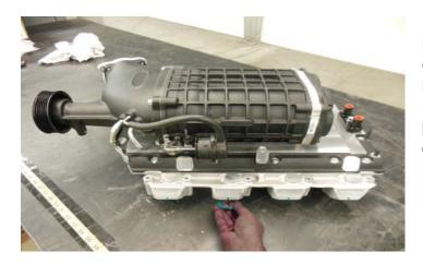
111. Remove the OEM O-ring gaskets from the intake manifold, clean, inspect and install in the grooves on the bottom of the supercharger intake manifold. If you find any damage you will need to replace the O-ring gaskets with GM replacement parts. The tab will line up with the slot on the outside edge.
