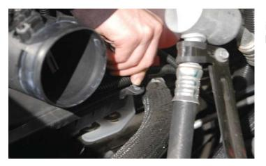
147. Push the wire loom mounting "tree" back into the hole on the back side flange of the air box.
