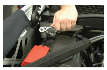
160. Re-connect the battery negative terminal using a 10mm socket wrench.
