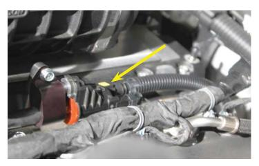
138. Connect the supplied EVAP hose to the rear of the left hand side head where the factory hose was removed earlier, and to the EVAP solenoid just mounted. The yellow locking clip end goes to the solenoid, and the gray locking clip end goes behind the cylinder head. Ensure that both "click" into locking position.
