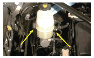
63. Remove the two nuts holding the master cylinder to the brake booster canister using a 15mm socket.
