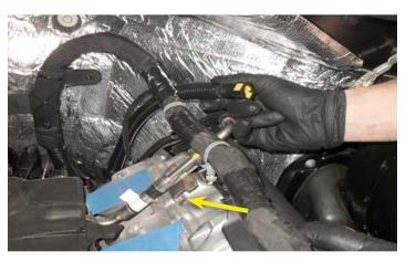
108. Connect the gray end of the new provided EVAP hose shown to the location where the factory EVAP hose was just removed. Remove the bolt holding the fuel injection line in place (shown with the arrow) to allow clearance while the supercharger is being installed. This bolt will be reinstalled after the supercharger is mounted.
