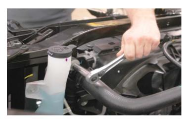
39. Remove the two upper radiator mounting bolts using a 13mm socket.
