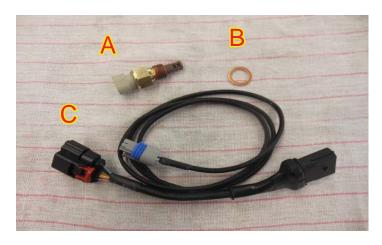
101. You should have the 3 parts shown to the left. (A) IAT sensor, (B) crush washer and (C) MAF/IAT breakout. To complete the installation of the sensor you will need a 19mm (or ¾") deep socket and a torque wrench capable of 175in-lbs (~15ft-lbs).
