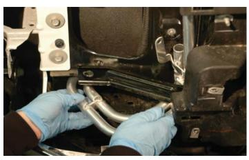
58. Rotate the assembly to push the bottom bends of the assembly into the engine compartment.
