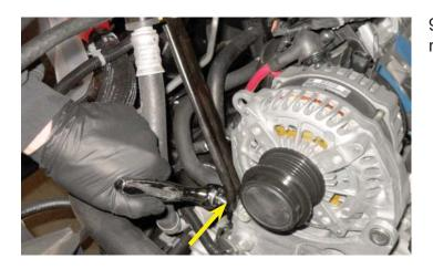
93. Remove the bracket located next to the alternator it will be re-attached later.
