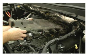
27. Carefully remove the valley cover foam insulating blanket from the vehicle. This will be reused after trimming in a later step.
