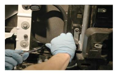
61. Replace the two nuts removed earlier and secure in place holding the angle brace back in position and the upper mounting tab of the coolant hard line assembly in position. Secure using a 10mm wrench.
