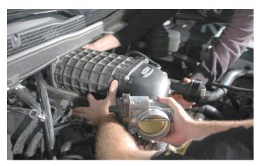
112. Spray a thin film of non-petroleum based lubricant, such as silicone spray or mild dishwashing detergent, on the port mounting surfaces to facilitate aligning and with the help of an assistant, carefully place the supercharger assembly into position.
