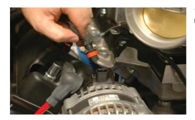
141. Connect the alternator control plug to the receptacle on the alternator.
