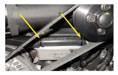
153. Anchor the PCV hose to the front of the supercharger intake manifold using the installed zip-tie tree mounts.
