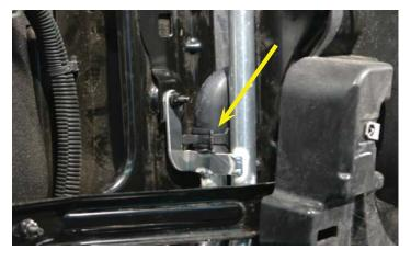
80. Connect the free end to the lower hard line hose barb using a provided spring clamp.
