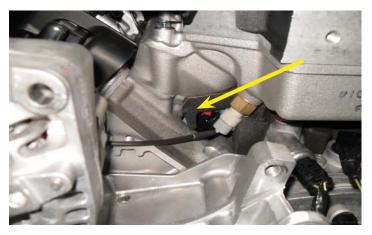
143. Plug the IAT end of the MAF/IAT breakout harness into the sensor. This can be done after the installation of the supercharger (as shown), or you can pre-install the harness and take extra precaution to not damage the connector during supercharger installation. If you choose to connect the sensor post install, it may be helpful to swing the alternator out of the way, as shown to the right.
