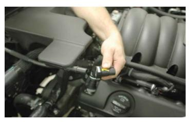
6. Depress the gray locking tab to release the PCV vent hose coming from the valve cover at the air plenum on both sides of the engine. Remove these two hoses for later reinstallation.
