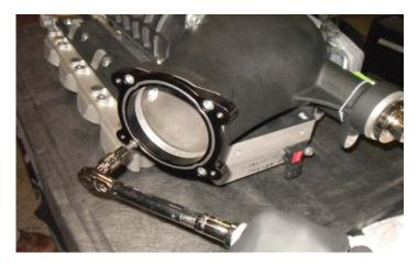
99. Install the throttle body adaptor plate, and torque to 108 in-lbs. Install the throttle body gasket removed earlier in the groove of the supercharger inlet. If the throttle body adaptor provided has a gasket you will not need to use the old one.
