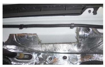
106. Here is a photo of the insulation after it has been removed.
