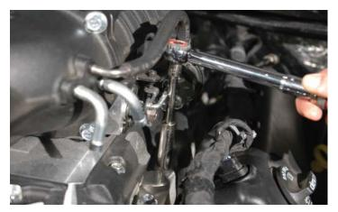
113. Apply blue Loctite 242 to the ten provided 75mm long supercharger mounting bolts. Install supercharger mounting bolts and torque in position to 106 in-lbs using a 10mm wrench. Follow the torque order given at the back of the book. At this point also reinstall the bolt holding the fuel injection line to the left side of the engine that was removed earlier.
