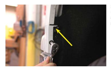
33. In the fender well, use a 7mm wrench to remove the two bolts (on each side of the vehicle) at the front skirt holding the fascia/grille bottom panel to the sub-frame.
