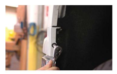
165. In the fender wells, use a 7mm wrench to replace the two bolts (on each side of the vehicle) at the front skirt holding the fascia/grille bottom panel to the sub-frame.
