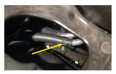
117. Route the hose from the right hand side of the charge air cooler forward, down, and connect to the remaining hardline hose barb below the airbox using a provided spring clamp. Secure the hose along its path with a few provided zip-ties.
