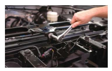
45. Remove the cross-frame support brace center bolt using a 13mm wrench.
