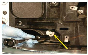
56. Use a 13mm socket to remove the bolt on the vertical frame below the diagonal brace. This bolt will not be reused.
