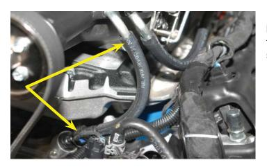
149. Connect the provided PCV hose with the blue colored quick connect locking pin between the existing valley cover hose barb on the left side and forward supercharger inlet hose barb.
