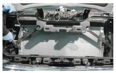
51. Attach the mounting brackets to the LTR mounting flange using the supplied bolts and a 12mm wrench. Do not tighten until you have aligned the LTR to be level, cross checking against the existing horizontal lines of the radiator. Secure in place when you've got proper alignment.
