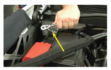
4. Loosen the nut shown with an arrow to disconnect the negative battery terminal. Cap or cover the terminal to protect against accidental contact with the battery post.
