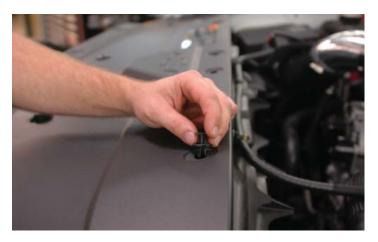
167. Replace the twelve push pin rivets in the top of the radiator cover by pushing the outside ring of the rivets in position and then push center pin down to spread the locking tabs.
