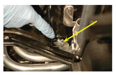
60. Use the provided bolt through the bottom mounting slot of the assembly into the hole vacated by the bolt you removed earlier. Secure in place using a 12mm wrench.
