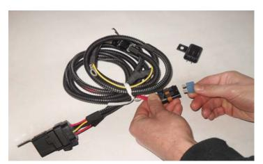
119. Install the provided fuse in the charge air cooler pump wiring harness fuse holder, replace the cap.
