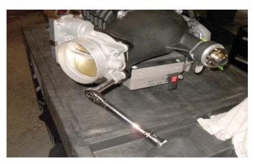
100. Install the OEM throttle body on the supercharger inlet using a 10mm wrench and torque to 106 in-lbs using the supplied 40mm long M6 fasteners.
