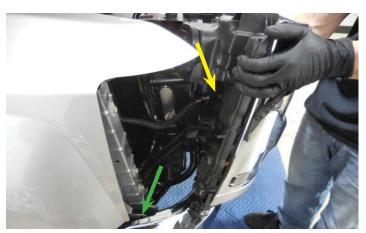
38. The green arrow in this photo shows the location for the hidden bolt that will have to be accessed from under the vehicle in the previous step if you have a 2016-17 truck. Lift up carefully on the headlight to separate it from the frame and disconnect the wiring harness plug (shown at the yellow arrow location) by pressing the release tab and pull it free. Set the headlight aside in a safe spot to be reinstalled in a later step. Repeat the removal process on the left side headlight.
