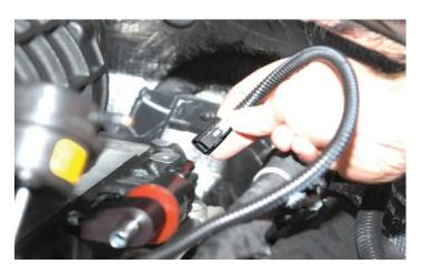
136. Connect the extended EVAP solenoid plug to the EVAP sensor. Secure the extension harness to the coil pack harness with a few of the provided zip-ties.
