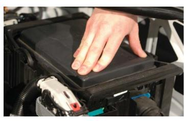
130. Replace the cover on the fuse center engaging the snaps. The lid should NOT be crimping down on the yellow wire.
