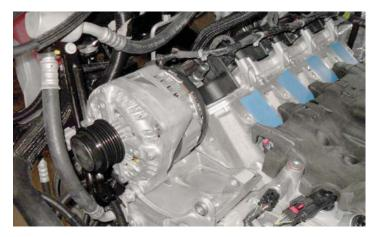
95. Alternator shown rotated out of the way.
