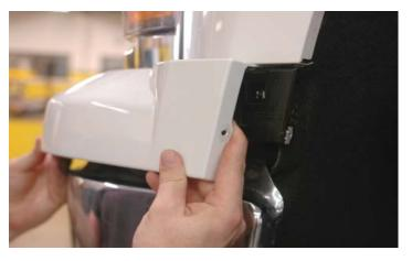
164. Carefully push in on the fascia bottom panels to snap the retaining clips into position.
