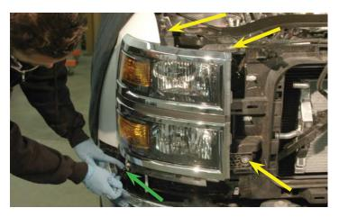
37. Use a 10mm wrench to remove the four headlight mounting bolts on the right side of the vehicle. For a 2016-17 truck the location shown with the green arrow will have to be accessed from under the vehicle. Review the photo in the next step to find the location for the bolt in the green arrow location.
