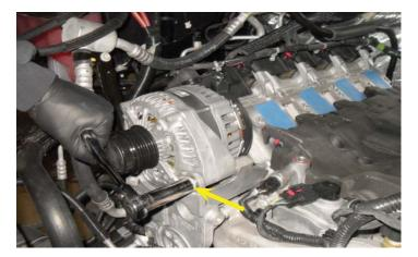
91. Remove the left alternator mounting bolt shown using a 15mm wrench.
