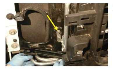
59. Align the mounting flange with the upper stud where you removed the bolt earlier.
