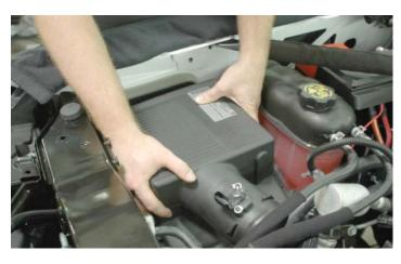
142. Replace the factory air box by pressing into position until the unit snaps in place.
