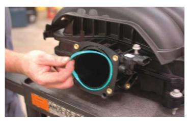
98. Remove the OEM throttle body gasket from the OEM intake manifold. Inspect for damage and clean as necessary. If you have a 5.3L engine this gasket will be re-used.
