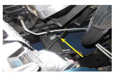
68. If you have a 2016-17 truck skip this step. Use a provided zip tie to anchor the harness to the existing black brake hard line, which runs parallel to the frame rail.
