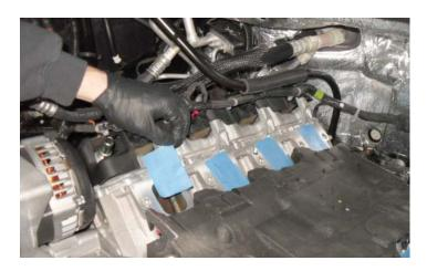
109. Remove the tape or rags covering the intake ports on the heads. Be careful to not allow any debris to fall into the exposed ports.
