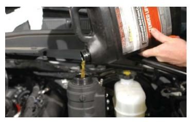
161. Fill the charge air cooler system with the vehicle manufacturer recommended coolant mixture. Have an assistant temporarily key the vehicle on to turn the pump on. Do not start the engine! Key vehicle off after 5 seconds. Fill reservoir full again and continue this process until fluid is circulating. Fill the reservoir to the top of the upper barb. At this time check engine and supercharger for any leaks.
