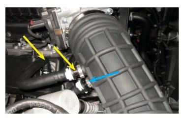
158. Connect the free end of the PCV hose from the left hand side front valve cover hose barb onto the lower hose barb of the air tube (Indicated with a blue arrow). Connect the provided 90° PCV hose between the hose barb on the right hand side front of the valve cover and the remaining upper hose barb of the air tube as shown.
