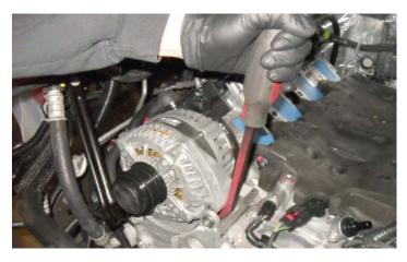
94. Pry alternator up to rotate it out of the way.
