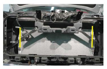
50. The LTR should now be resting on the bottom tray forward of the radiator. Center the unit and use the mounting bracket holes to align and place the mounting brackets on the "A-Frame" in front of the radiator.
