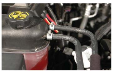
42. The hoses going to the radiator overflow tank can be disconnected. This is not absolutely necessary but does make the job a bit easier. Connect the two hoses together using a coupling (hose mender), or plug them with a plug or dowel and tuck out of the way. Again, this is not absolutely necessary.
