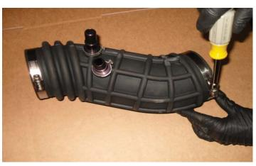
154. Gather the rubber duct shown. Loosen hose clamps to prepare for install. The left side clamp will be taken off completely to install over throttle body.
