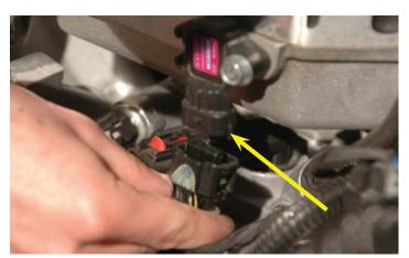
139. Connect the MAP sensor plug to the connector on the MAP sensor.
