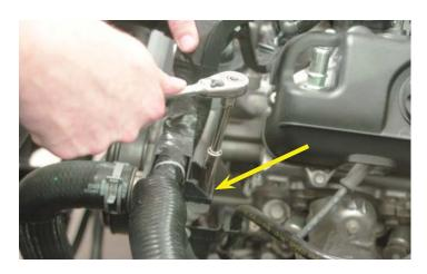
21. Use a 10 mm wrench to remove the bolt from the lower mounting bracket anchoring the wire harness.
