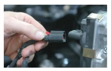
140. Connect the throttle body plug to the throttle body.
