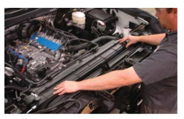
52. Replace the upper radiator shroud by snapping into place.
