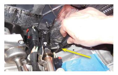
107. Remove the factory EVAP hose from behind the left side cylinder. Squeeze the connector clip to release the clip and pull free.
