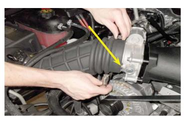
156. Install rubber duct onto throttle body side, and install hose clamp around connection. Make sure duct tabs line up with throttle body indicated with arrow.
