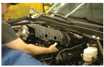
26. Pull the OEM intake manifold out of the vehicle and set aside. Parts will be used from this assembly. Gaskets, and throttle body will be reused.
