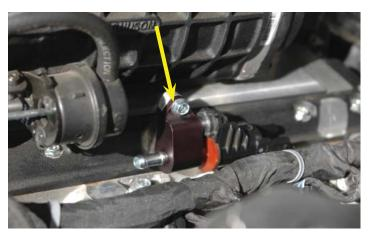
135. Mount the EVAP solenoid mounting bracket to the left side boss on the supercharger lid using the provided 16mm long bolt and secure in place with a 10mm wrench.
