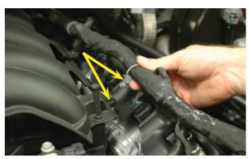
22. Remove the three harness "tree" clamps from the left side of the intake manifold.
