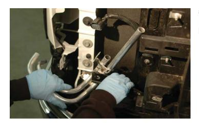
57. Gently pull out on the diagonal brace by the removed nut, and slide the provided coolant hard line assembly behind the brace as shown.
