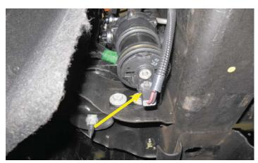
122. Route the plug from the wiring harness down to the inside of the fuse center, along the existing wiring harness and plug into the intercooler pump connector.
