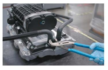
96. Connect the short leg of the cut/assembled 23" x 3" x 3/4" 90° elbow hose to the outside left hand side charge air cooler hose barb at the back of the supercharger assembly. Secure in place with a provided spring clamp. Connect the cut/assembled 51" x 3" x 3/4" 90° elbow hose to the right hand side charge air cooler hose barb at the back of the supercharger assembly. Secure in place with a provided clamp. The hoses route toward their respective sides as shown.
