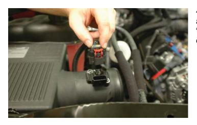
41. Disconnect the airbox MAF plug from the airbox on the right side of the vehicle. Pull the "tree" clip from the mounting hole in the airbox disconnecting the harness to the airbox.
