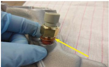
103. It is very critical that the crush washer sits between the brass sensor housing and the aluminum manifold. This will ensure there is an air tight seal between the sensor and manifold. Begin by placing the crush washer over the brass threads the IAT sensor; then thread the sensor into the manifold by hand until snug.
