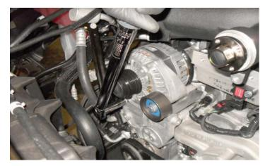
115. Torque the other alternator bolt to 25 ft-lbs. Re-attach the bracket adjacent to the bolt just torqued.
