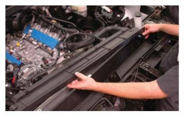
47. Pull up on the upper radiator shroud to unsnap it from the retaining slots, set aside for later re-install.
