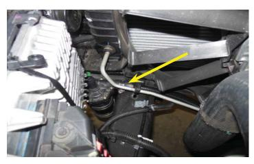
74. Install the "Pump to Hardline" hose using a provided worm gear clamp on the pump discharge hose barb.
