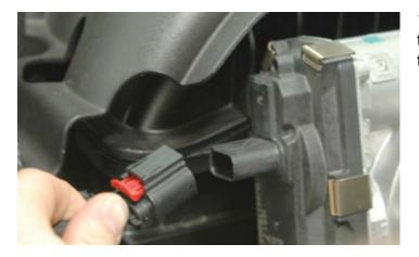
11. Disconnect the ETC connector from the throttle body. Depress the locking tab and pull the connector free.
