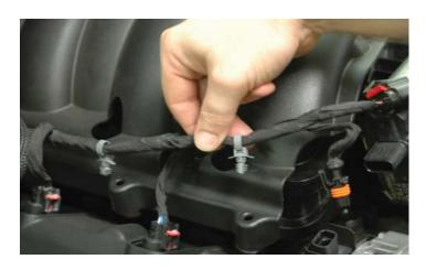
13. Pull the four "tree" tab wire loom mounting anchors from the holes in the right side of the intake manifold.
