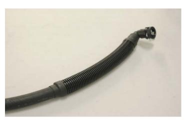
151. Slide the provided 8" section of split loom over the PCV hose and anchor in place at each end using two 1" pieces of the provided heat shrink as shown.
