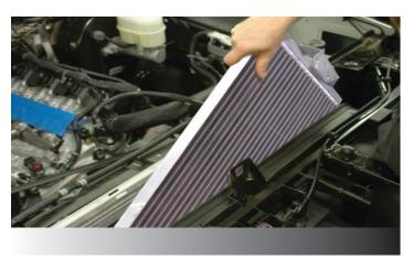
48. Slide the provided low temperature radiator (LTR) assembly into the space created by pushing the radiator assembly top section toward the rear of the vehicle. The mounting brackets should be pointing forward, the hose barbs on the right side of the vehicle. Be careful to not damage the existing radiator or the LTR.
