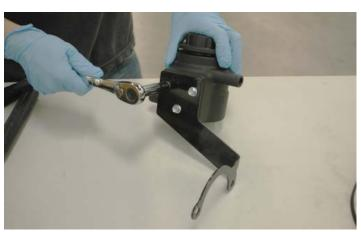
62. Attach the supplied reservoir mounting bracket to the reservoir with the provided bolts and secure using a 10mm wrench.
