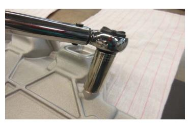
104. Once the sensor is snug to the crush washer, set your torque wrench to 175in-lbs (~15ft-lbs). With a 19mm (or ¾") deep socket attached to your torque wrench, torque the sensor down. \*Note: Take care when installing the sensor into your socket so it does not get damaged. When flipping the supercharger right side up be careful not to crush the sensor.
