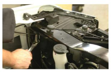
44. Remove the three (each side) upper radiator cross-frame support brace bolts using a 10mm wrench. These are all accessible only from below the support brace. Use a flathead screwdriver or a push rivet removal tool to unsnap the top rivets of the rubber air deflector on the right side to ease access.
