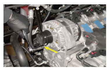
92. Loosen the other alternator support bolt shown.
