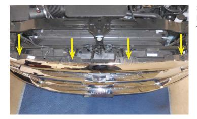
35. Remove the four bolts (shown with arrows) holding the top of the fascia/grille to the sub frame using a 10mm wrench.
