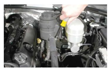
81. Connect one end of the "Reservoir to Pump" inlet hose to the reservoir using a provided worm gear clamp. It's important to utilize only worm gear clamps on the reservoir.
