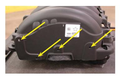
25. This image shows the location of the four tree connectors on the back of the intake manifold.
