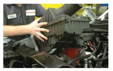
43. Pull the factory airbox from the vehicle, there are no screws anchoring the airbox in place, locating pins push through grommets, a firm pull will disconnect. Set the airbox aside for installation in a later step.
