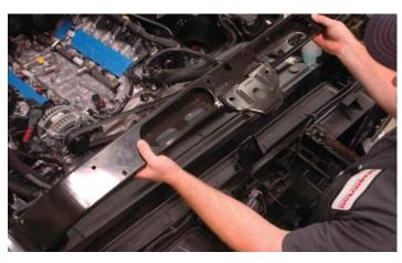
46. Pull the cross-frame support brace from the vehicle and set aside for re-install in a later step.
