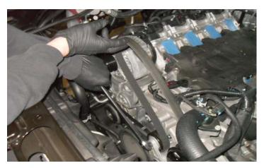
90. Remove the OEM drive belt by springing the tensioner using a ½" breaker bar or socket wrench, if necessary utilize a piece of pipe to extend the lever length. This belt will NOT be reused.
