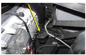
82. Route the other end forward and down to connect to the intercooler pump inlet hose barb using a provided spring clamp.
