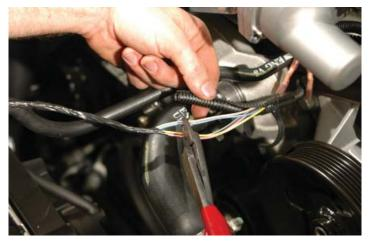
141. Pull these two wires out of the loom back to where the split-ring mount clamps to the hose barb at the water-pump. Tuck the two white wires from step #138 under the supercharger inlet and crimp one to each of the tan and blue wires. It doesn't matter which attaches to which.
