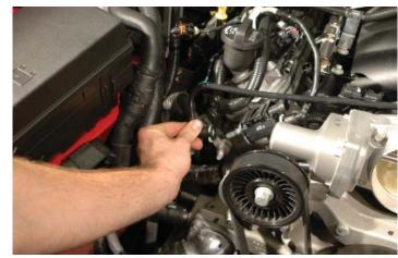
23. Unplug the remaining EVAP hose that goes from the sensor to the hard-line fitting on the passenger side. Tuck aside near the brake module for later reinstall.
