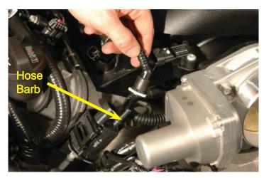
24. LS3 Engines: Unplug the PCV hose from the OEM manifold to the valley cover. This is a short "U" loop and will not be reused. L99 Engines: This hose goes from the OEM manifold back to the hose barb at the rear of the driver sided valve cover and will also not be reused.
