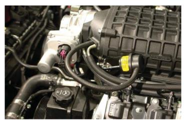
136. Tie the PCV, Brake Booster, and Bypass hoses together loosely with a zip tie as shown.
