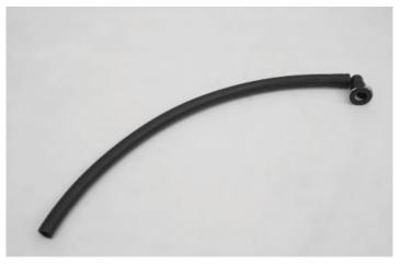
129. Connect the 90° fitting to the bottom barb of the EVAP solenoid. Route the other end over the jack shaft to the hose barb on the Supercharger inlet on the passenger side of the engine, again no clamp is necessary.
