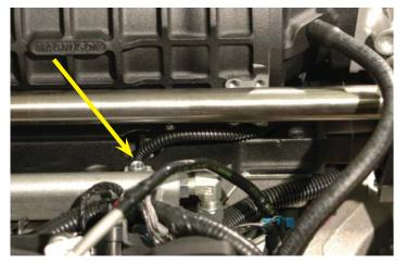
145. Use a 15mm wrench to remove the OEM tensioner pulley.
