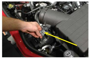
151. On the passenger side of the engine, near the thermostat on the frame rail, unplug the fuse center wire loom hold-down clip by pulling it away from the frame.
