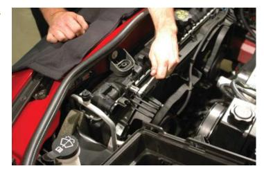
42. Carefully lift the fan shroud assembly from the vehicle and put aside for later reinstallation.
