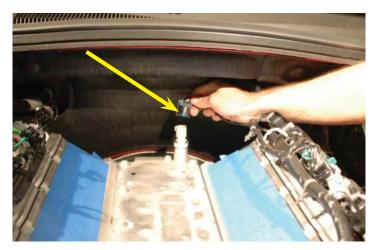
56. Remove the oil pressure sensor from the valley cover using a 6-point 1-1/16" socket or wrench, put aside for later re-installation. NOTE: L-99 cars or cars with Displacement On Demand (D.O.D.) will retain D.O.D. valley cover, skip to step #62. Damage to engine may occur if MagnaCharger valley cover is installed on D.O.D. equipped vehicles.
