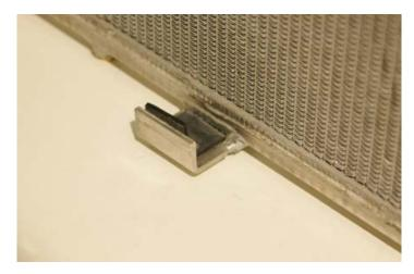
78. Attach one strip of the adhesive backed foam to the inside-upper edge of the heat exchanger, overlapping the rubber strips as shown.
