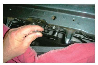
68. Loosen the 13mm bolts securing the bottom of the "A-frame" member to the frame rails on each side of the vehicle.
