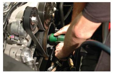
53. Using a 24mm socket tighten the new Harmonic Balancer bolt according to General Motors specifications. Tighten to 50 N-m (37 ft/lbs) then tighten an additional 140° using a torque angle meter.
