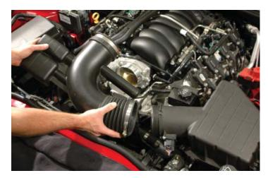
14. Rotate the passenger side vent tube removed from the air inlet in step #11 to expose the release tab. This will be at the front of the passenger side valve cover adjacent to the oil fill spout. Spread the tab to release from the hose barb and remove the hose. This will not be reused.
