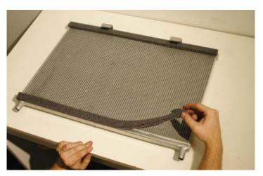
80. Replace the plastic plug on the top of the heat exchanger with the provided brass plug. Cut 1-3/4" off the short side of the ¾" x 4" x 60" x 90° angle hose. Use the supplied spring hose clamps to attach the short end to the passenger side barb of the heat exchanger. This hose will angle directly outward from the heat exchanger as shown. With the mounting angles pointing down, this will be the left hose barb.
