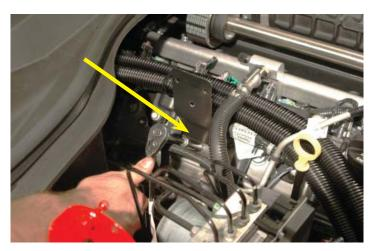
156. Attach the reservoir bottle to the bracket as shown with the supplied bolts and a 10mm wrench.
