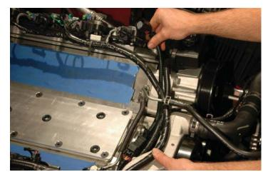
94. Disconnect the main coil connectors from the center of the coil rails on both sides of the engine.
