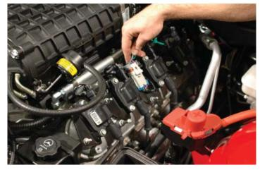
121. Attach the stock plug connectors back onto the coils on the coil brackets on both sides of the engine.
