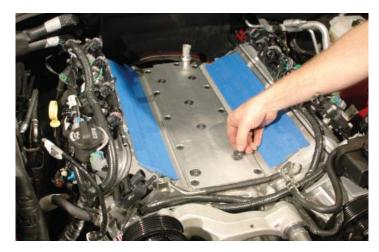
66. Replace the oil pressure sensor plug and locking clip on the oil pressure sensor.
