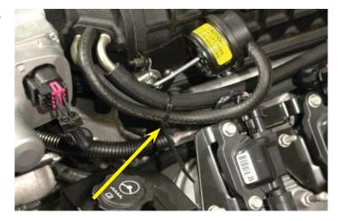
137. Add a zip tie to loosely tie the brake booster hose and the PCV hose together where they meet at the rear of the engine.
