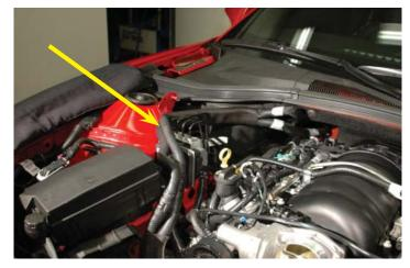
17. Disconnect the EVAP solenoid electrical connector.
