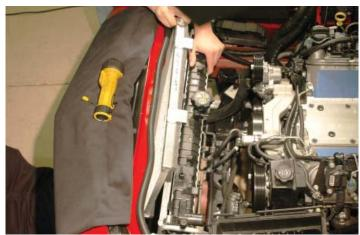
84. Guide the "hooks" of the intercooler heat exchanger over the top of the AC Condenser. Ensure that the foam is between the two (both top and bottom), and the rubber strips are still in place around the "hooks".
