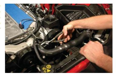
38. Disconnect the overflow hose from the radiator fill spout, pull free from the mounting clamps and wrap up around the overflow bottle cap out of the way.
