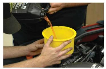
195. Fill the Intercooler System with the vehicle manufacturer recommended coolant mixture. Have an assistant temporarily key vehicle on to accessory mode (Do Not start the vehicle) to turn the pump on. Key vehicle off after 5 seconds. Fill reservoir full again and continue this process until fluid is circulating. At this time check your intercooler system, and fuel system for leaks.
