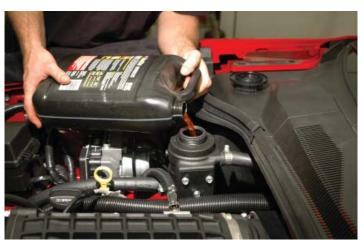
196. Start the vehicle for 5 seconds and shut off. Check for fuel leaks and supercharger belt alignment. Check the intercooler reservoir level. Now start your engine and let it run for a few minutes to let it get to operating conditions. Let the engine cool down, and check all your levels again.
