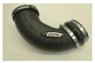
188. Push the air inlet tube onto the air-box and throttle body necks and tighten all clamps securely.
