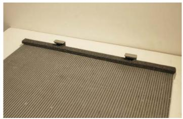
79. Attach the other strip to the inside-bottom edge of the heat exchanger as shown.
