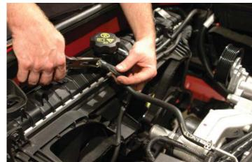
91. Pull the radiator upper hose from between the PS pump and air box, and relocate to the stock barbs on the water pump and radiator, re-attach the hose clamps to secure the hose to the hose barbs.
