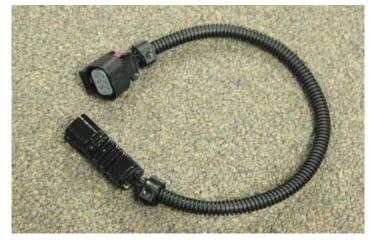
93. Locate the ETC connector on the OEM engine harness. Plug the extension harness into the existing ETC connector and route adjacent to the steam pipe to the driver side of the engine.
