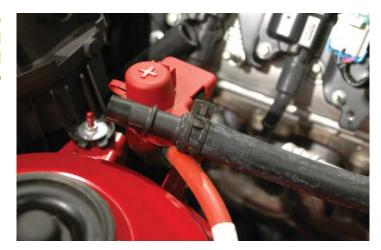
166. Route the remaining driver side intercooler heat exchanger hose up into the engine compartment toward the air conditioner hoses. Cut 2-1/2" off the hose end and using the provided clamp join the hose to the hose coupler just installed in the previous step. Use a zip tie to anchor the coupling to the existing battery wire loom bundle behind the air-box.
