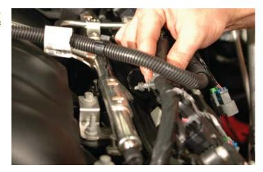
22. Press on the light tabs of the EVAP line to release the clips from the EVAP solenoid and the Throttle Body. Put aside for later modification.
