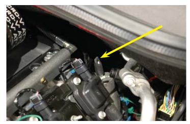
131. Cut a section of the 3/8" hose to 22" in length. Plug one end of this hose on this PCV valve barb just uncovered.
