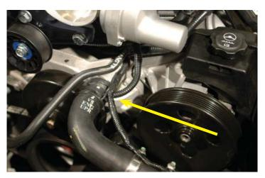
144. The other end should reach all the way to the other end of the wires at the Supercharger lid. It's a good idea to cross tape the junction of the two split looms at the water-pump hose barb.
