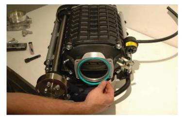
109. Install the OEM throttle body onto the supercharger inlet using a 10mm socket wrench. Torque the bolts to 106 in-lbs. Make sure you are using the correct settings on your torque wrench.
