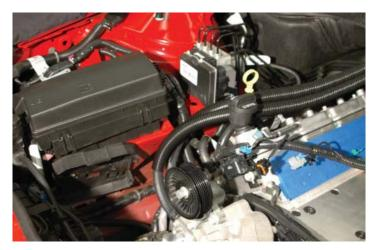
104. Remove the MAP sensor from the OEM intake manifold using a T-25 Torx wrench.
