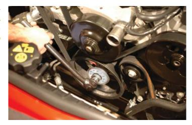
54. Using a 15mm socket on the Tensioner Pulley bolt, spring the pulley down to remove tension on the drive belt and remove the belt when tension has been released.
