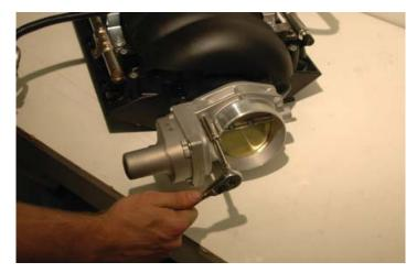
106. Remove the O-ring from the stock throttle body connector groove.
