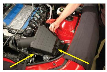
36. Rotate the air-box cover up and away from the clips, remove the filter and put both the filter and the cover aside for later reinstallation.
