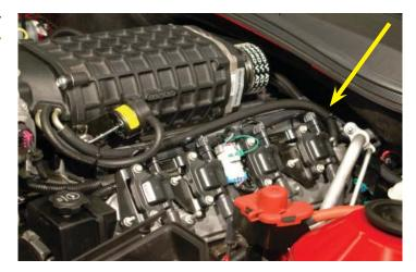
138. On the passenger side of the Supercharger assembly, near the front are two white wires exiting the intercooler lid. These are the IAT sensor wires. Strip off about 3/8" of the insulation on each of these wires.
