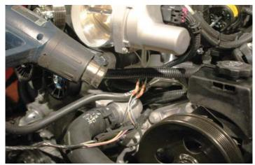
143. Cut a piece of the provided split loom (about 18") to reach from the split-ring clamp, following the white wires back to where they enter the Supercharger lid on the passenger side of the Supercharger. Slide the split loom over the wires, one end should be at the junction by the split-ring clamp.
