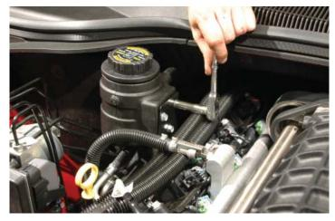
157. Route the passenger side hose from the intercooler heat exchanger up into the engine compartment. Cut the hose to fit at the intercooler pump discharge barb. Clamp on using a supplied spring clamp. Save the cut section of hose for the next step.
