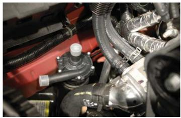
155. Mount the supplied reservoir mounting bracket to the center stud of the passenger side coil bracket using the supplied nut and a 10mm wrench.
