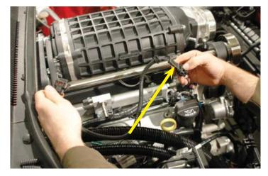
117. Plug the other end of the extension harness into the MAP sensor located under the rear fuel rail cross-over tube at the back of the passenger side of the engine.
