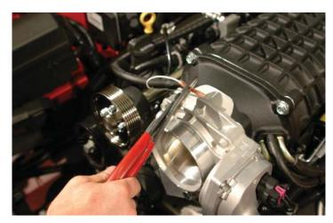
140. Uncover the MAF wire loom connector that hooks to the air box. This should be by the upper radiator hose at the water-pump. Cut the blue and the tan wire even with the end of the existing wire loom. Strip off about 3/8" of insulation from the end of the two wires that continue back in the split loom toward the engine.
