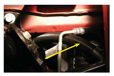
168. Slide a length of the provided 1" split loom over the driver side intercooler heat exchanger hose to protect the hose from chaffing at the rectangular hole in the splash shield and adjacent edges.
