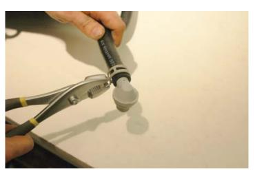
108. Install the O-ring just removed from the manifold into the groove on the supercharger inlet.
