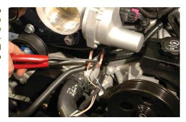
142. Use a heat gun or hair dryer set on high to shrink these connections securely. The ends of the blue and tan wires that go to the plug are abandoned and can be taped off and recovered with the existing split loom.
