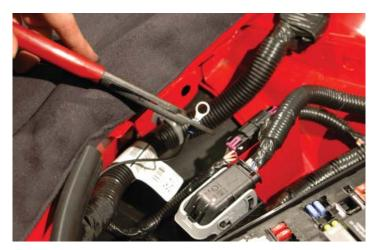
180. Use the self tapping bolt from step #178, incorporate the just installed "eyelet" on the black wire from step #179, and ground the wire harness to the automobile body at the prepped hole. Tighten snugly being careful to not strip the threads.
