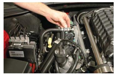
125. Plug in the EVAP solenoid electrical connection at the front of the passenger side valve cover.
