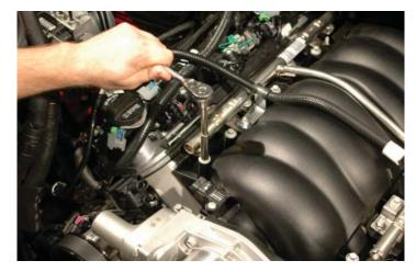
30. Carefully lift the OEM intake manifold assembly from the vehicle. Put aside for the moment, we will be using some components later.
