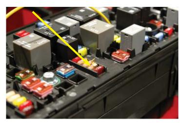
184. Strip off 3/8" of the insulation off the end of the yellow wire and crimp on the provided spade connector.
