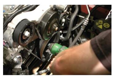
44. Install the supplied drill guide using the supplied bolt. Torque the bolt to 30 ft-lbs using a 24mm socket and torque wrench. Verify your torque wrench settings.
