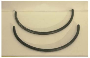
101. Take the 34" x 5/8" hose and use one of the clamps removed to attach the hose to the smaller barb at the water-pump. Route the other end up between the oil fill spout and dipstick. Use one of the removed clamps to connect the hose to the smaller barb (outside) on the firewall.
