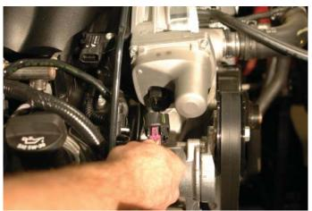
21. Pull the wire loom anchors free from the mounting holes on the OEM fuel rails on both sides of the engine.
