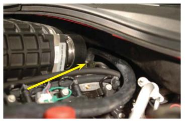
165. Cut 11" off the end of this hose and route below the air conditioner hose bending toward the front of the vehicle. Insert the provided hose coupler and use the provided clamp to prepare the end of this hose.
