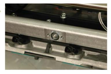
113. Install the fuel supply manifold on the fuel rail and torque to 106 in-lbs. Verify your torque wrench settings.
