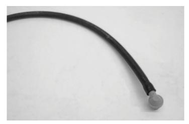
134. Depending on the car, install the check valve or sensor with hose at the brake booster as shown. Route the hose laterally toward the engine and turn it forward to parallel the PCV hose just installed.
