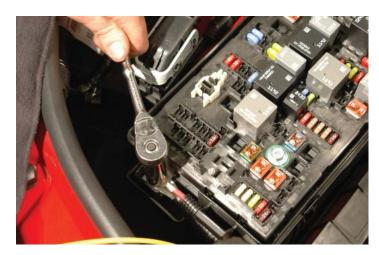
176. Zip tie the fuse holder of the wire harness to the existing wire harness by the headlight adjusting screw as shown.
