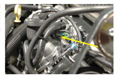
190. Route the other end of the hose behind the pulleys and push onto the hose barb on the bottom of the air inlet tube assembly, in front of the throttle body.
