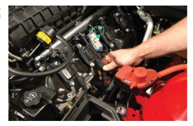
Plug in the electronic throttle body connection on the driver side of the throttle body.
