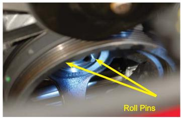
51. The use of a small hammer and punch may be necessary to tap the pins in. Make sure that the pins are in far enough that they do NOT touch the balancer bolt.
