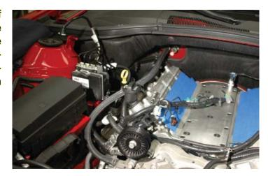
102. Use the 35" x 3/4" hose and the removed clamps to attach to the remaining barb on the water-pump. Route the other end parallel to the just installed hose and connect to the remaining hose barb at the firewall using one of the removed clamps.
