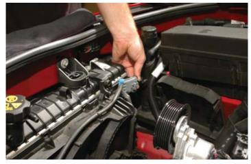
89. Uncoil the coolant overflow from the reservoir bottle, and relocate through the stock clip locations. Re-connect the coolant overflow hose back onto the hose barb on the radiator neck.
