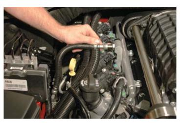
124. Remove the fuel line safety clip from the fuel line still attached to the OEM intake manifold. Use this and the clip removed in step #26 to re-attach fuel line safety clips on both ends of the fuel line.
