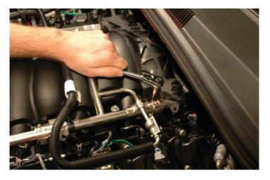
29. Unbolt the OEM intake manifold by removing the ten intake manifold bolts using an 8mm socket wrench; there are five on each side.
