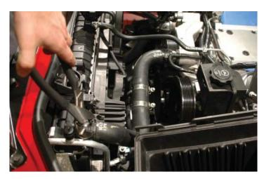
92. This is the provided Electronic Throttle control (ETC) connector extension harness.
