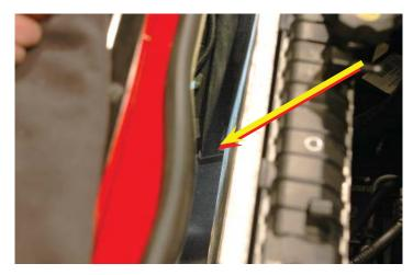
83. With the help of an assistant, guide the two hoses through these holes. From below pull on these hoses while the assistant holds the radiator pushed back and guides the heat exchanger down in front of the existing radiator and AC condenser assembly.
