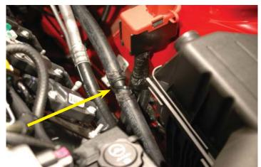
167. Slide a length of the provided 1" split loom over the passenger side intercooler heat exchanger hose to protect the hose from chaffing at the rectangular hole in the splash shield and adjacent edges.
