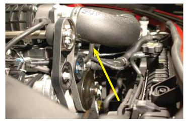
191. Attach the Vacuum routing diagram, intercooler-belt routing diagram/information sticker in a conspicuous location. We chose the underside of the hood.
