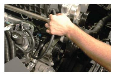
130. On the driver side of the engine, at the rear of the valve cover, adjacent to the fuel rail crossover and the coil bracket is a PCV hose barb covered with a cap. Remove this cap. NOTE: L-99 or D.O.D. vehicles will not have this cap and instead will have a PCV hose connection here.
