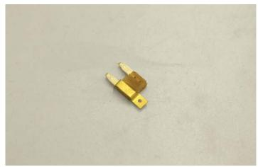
183. Replace the IGN fuse with the fuse tap back into the slot from whence it came.
