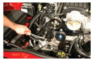
146. Install the supplied 76mm pulley and torque the bolt to 40 ft-lbs. Verify your torque wrench settings.
