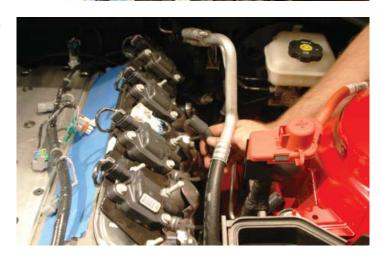
96. Use a 10mm wrench to remove the five bolts from the coil brackets on each side of the engine.
