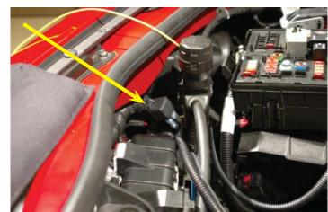
175. Replace the positive (+) lug nut incorporating the red wire "eyelet" you attached in step #173 from the new harness.
