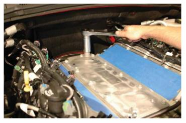
57. Remove the eleven valley cover bolts using a 13mm socket and set aside. NOTE: L-99 cars or cars with Displacement On Demand (D.O.D.) will retain D.O.D. valley cover, skip to step #62. Damage to engine may occur if MagnaCharger valley cover is installed on D.O.D. equipped vehicles.
