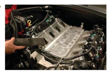
32. Wipe off the heads with some alcohol or suitable solvent to eliminate any oils or residue that may have collected.
