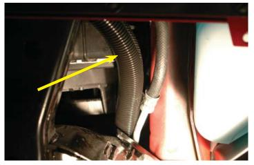
169. These are the intercooler pump wiring harness components.
