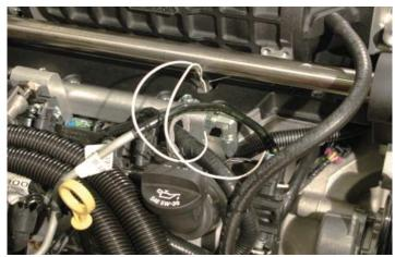
139. Crimp on a provided wire splice connector to each of these wire ends.
