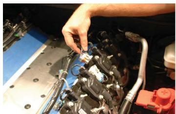
95. Disconnect all plug wires from the coils on both sides of the engine.
