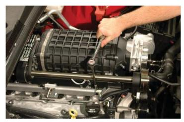
116. Attach the supplied MAP sensor extension harness to the existing MAP plug.
