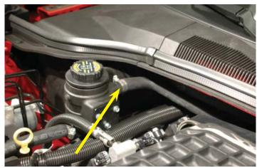
163. Cut 1-1/2" off the short leg of the remaining <sup>3</sup>/<sub>4</sub>" x 4" x 36" x 90° hose.
