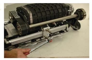
114. Remove the tape from the heads and lubricate with silicone spray, mildly soapy water spray, or a suitable lubricant (non-petroleum based-to allow some sliding movement), get an assistant to help, and carefully lift the supercharger assembly into the engine.
