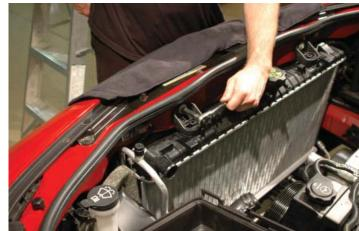
87. With the radiator mounted back in the stock location, use a 13mm wrench and the stock hardware to re-install the electric fan shroud assembly.
