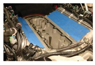
60. Remove the existing O-ring seals from the OEM valley cover, and place in the O-ring grooves of the new provided valley cover. NOTE: L-99 cars or cars with Displacement On Demand (D.O.D.) will retain D.O.D. valley cover, skip to step #62. Damage to engine may occur if MagnaCharger valley cover is installed on D.O.D. equipped vehicles.
