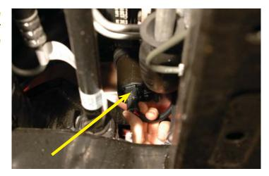
178. Use one of the provided self tapping bolts and a ½" socket to tap the hole in the fender well just forward of the shock tower and above the existing wire loom as shown.
