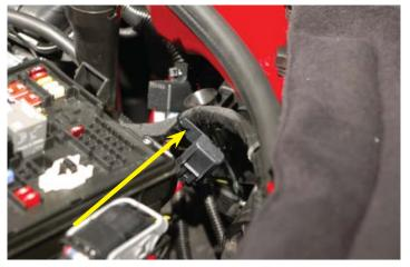
177. Route the intercooler pump plug around the fuse center and down toward the intercooler pump. Plug the end into the terminal at the bottom of the intercooler pump.
