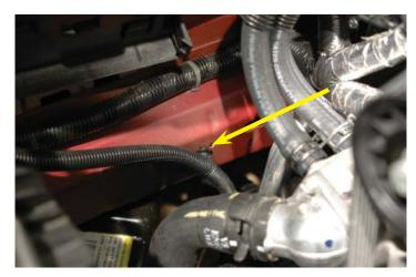
152. Use the provided self-tapping bolt and a ½" socket to prep the hole just vacated for mounting the intercooler pump. Chase the hole to ensure the proper bolt function.
