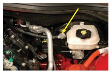
135. Route the hose just below the PCV hose between the fuel rails and coil bracket and attach the loose end to the front barb on the Supercharger inlet.
