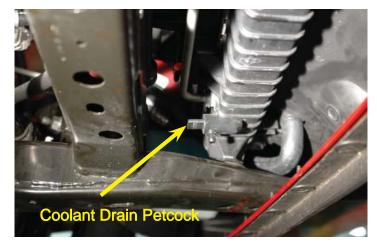
10. Remove the radiator cap to facilitate draining. When the radiator is drained, reset the petcock valve to shut, and replace the radiator cap.
