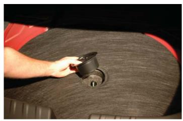
4. Pull up on the access panel to remove.
