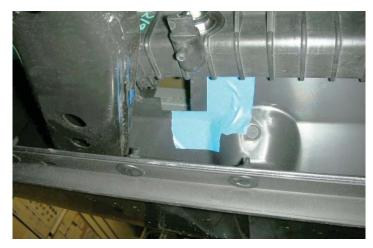
70. Once your notches are complete, reconnect the top "A-frame" bracket using the provided longer bolts, incorporating the provided spacer between the "A-frame" and the upper cross frame fascia support. Tighten all your bolts and torque to 40 ft-lbs. Verify your torque wrench settings.
