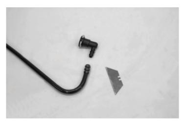
128. Cut a 15" piece of the supplied 5/16" hose and install the right angle fitting just removed in the last step.
