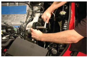
55. Unplug the oil pressure sensor from the back, driver-side of the OEM valley cover.
