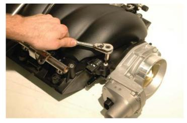
105. Use a 10mm socket wrench to unbolt and remove the throttle body from the OEM intake manifold.
