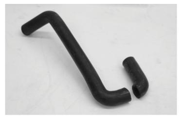
161. Use a provided spring clamp on the end of the hose you just cut and push the remaining section of the "U" onto the passenger side barb of the intercooler. Verify your hose is secure and the hose is pointed toward the passenger side of the car as shown.
