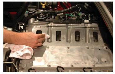
33. Cover the intake ports with tape to maintain a clean environment. It's important to keep your work surfaces clean, avoid contamination, or any debris falling into the exposed engine interior.
