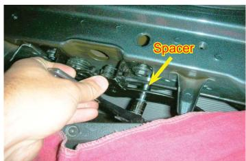
71. **NOTE:** All vehicles continue from here: Remove the two upper radiator mounting bolts using a 10mm socket wrench.
