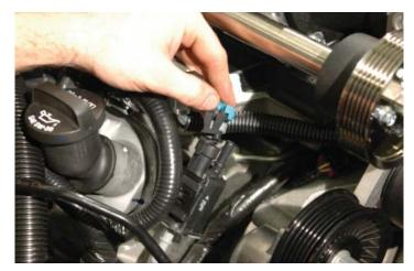
126. Plug in the 90° fitting of the EVAP tube (from the hard-line on the passenger side running over the heater hoses) to the upper EVAP solenoid barb.
