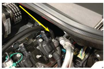
132. Route this hose along the fuel rail forward to the closest barb on the driver side of the Supercharger inlet.
