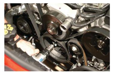
46. Using compressed air, blow the drill shavings out of the holes. (Caution: Wear safety glasses, and make sure that debris doesn't blow into surrounding openings...such as the waterpump barb etc.)
