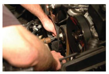
52. Install the new supplied factory GM Harmonic Balancer bolt.
