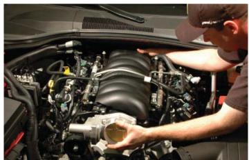
31. Vacuum off the valley cover to ensure that no debris enters the ports.
