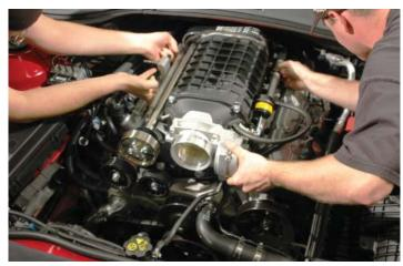
115. Remove the split loom spacers from the pre-installed manifold bolts and after an initial hand tighten using a 10mm socket, torque the bolts down to 106 in-lbs using a cross rotation pattern. Make sure to verify your torque wrench settings.
