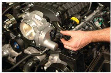
123. Attach the supplied fuel line between the fuel supply barb below the ABS Module (where the OEM fuel line was disconnected in steps # 26-27) and the new fuel rail manifold on the passenger side of the vehicle. Pull firmly on both ends to verify that you have a good connection. The EVAP sensor tube should be under the fuel line and above the heater hoses. IMPORTANT: You should NOT be able to remove the fuel line from either end without the use of the fuel line removal tool.
