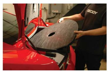
5. Pull up on the Styrofoam mount support and tire compressor to remove from the vehicle. Put these parts aside for later reinstallation.
