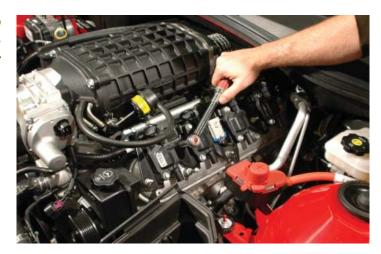
120. Plug in the main coil connectors on both sides of the engine.
