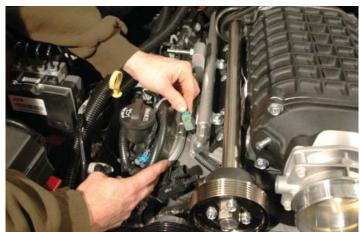
119. Re-mount the modified coil brackets to each side of the engine using the stock hardware. Torque all bolts to 106 in-lbs. Verify your torque wrench settings.
