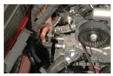
16. Tuck the hoses over the brake module and out of the way, be aware of residual fluid that may be inside the hoses.
