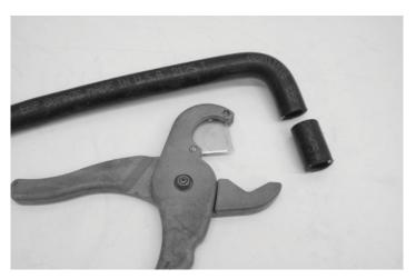
164. Place a provided clamp on the short leg of this hose and push the end onto the intercooler barb on the driver side behind the supercharger. Tighten the clamp securely with the hose pointing toward the driver side of the vehicle.
