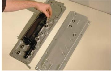
61. Install the new valley cover using the eleven provided Allen-countersunk bolts. Torque to 18 ft. Ibs using a 5mm Allen socket. Verify your torque wrench settings. NOTE: L-99 cars or cars with Displacement On Demand (D.O.D.) will retain D.O.D. valley cover, skip to step #62. Damage to engine may occur if MagnaCharger valley cover is installed on D.O.D. equipped vehicles.
