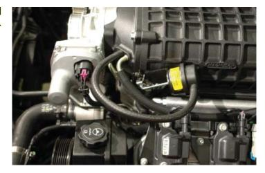
133. Cut a section of the supplied 11/32" brake hose to 30" in length. Attach the OEM check valve removed in step #107 to one end of this hose. NOTE: L-99 or D.O.D. cars; brake booster will have a sensor in place of the check valve. Install the hose onto the sensor instead. Sensor was removed from booster for ease of installation and photograph.
