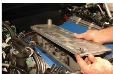
59. Verify the integrity of the existing valley cover gasket, and that it is correctly positioned on the valley surface. NOTE: L-99 cars or cars with Displacement On Demand (D.O.D.) will retain D.O.D. valley cover, skip to step #62. Damage to engine may occur if MagnaCharger valley cover is installed on D.O.D. equipped vehicles.
