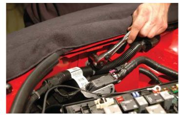
179. Cut the existing "eyelet" connector off the black ground (-) wire, strip off ½" of the insulation and crimp on the supplied larger "eyelet" connector.
