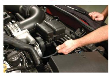
12. Use an 8mm wrench to loosen the clamps at the air box and throttle body.
