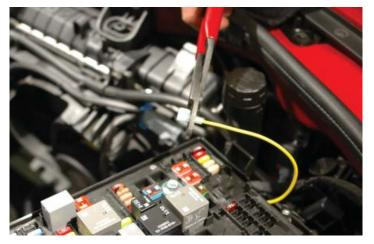
185. Route this wire into the fuse center and connect it to the fuse-tap on the IGN fuse you just reinstalled.
