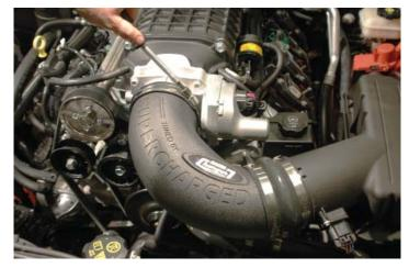
189. Cut a piece of the remaining 3/8" hose to fit between the PCV fitting on the passenger side valve cover near the oil-fill spout, and the hose barb on the bottom of the air tube assembly. Push one end onto the hose barb at the front of the valve cover.
