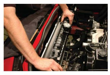
86. Reinstall the upper radiator clamps using the stock hardware and a 10mm wrench. Tighten securely.
