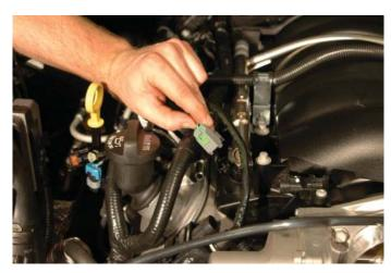
20. Unplug the electronic throttle body connection.
