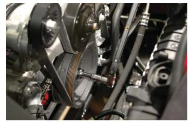
45. Using a small or angled 3/8" drill and the supplied drill bit, insert the drill into the two guide holes and drill to the second step of the drill bit. Be sure that you drill all the way to the second step, and use with suitable cutting oil. (Caution: Wear safety glasses)
