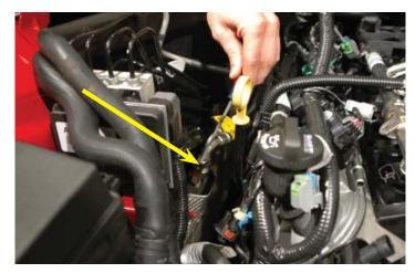
27. Use the provided fuel line removal tool to release the fuel line from the hard-line barb. The proper way to do this is to press the line into the fitting first, insert the tool and while the line is pressed in, push the tool into the fitting. Then pull the line free from the hose barb. If you have, or can improvise, we suggest that you cap both the hard-line barb and the fuel line.
