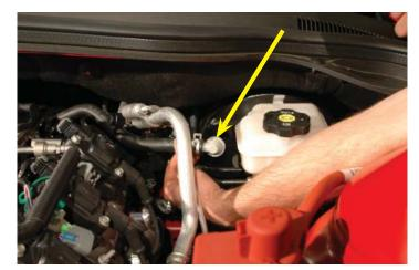
26. Pry the retaining clip off the fuel line at the passenger side of the vehicle just below the brake module. Put this clip aside for later installation.
