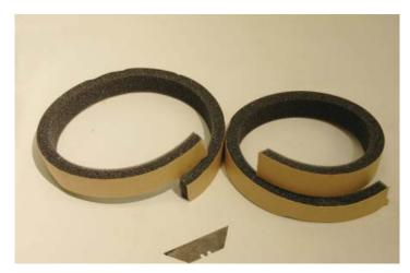
76. Cut two strips of the supplied adhesive backed rubber to fit the upper mounting angles of the heat exchanger. These will butt up against the heat exchanger and wrap around the inside edge of the angle.
