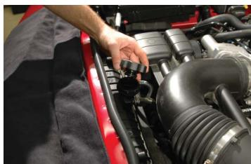
11. Pull the passenger side vent tube off at the plastic box between the throttle body and the intake air box.
