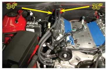
103. Cut two pieces of the supplied split loom to cover these hoses as they pass by the existing fuse center mounting platform and over the valve covers.
