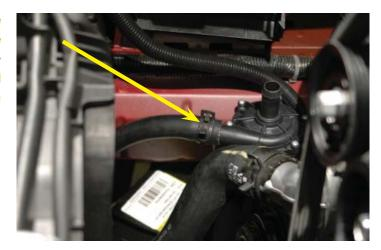
158. Take the cut-off section of the hose in the last step and attach one end to the inlet barb of the intercooler pump. Clamp on the barb with a provided spring clamp.
