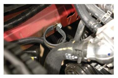
154. Slide the pump into the Adel clamp. Access to tighten the bolt is easiest if done from below.
