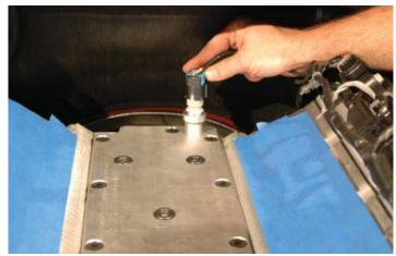
67. NOTE: If you have a convertible Camaro, the next four steps are required. The convertible model has some minor frame stiffening modifications. One of these is an additional "A-frame" type brace to the upper, fascia cross frame. Remove the two top bolts of this "A" frame brace using a 12mm wrench.
