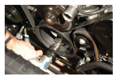
48. Using a 24mm socket, remove the large bolt and drill guide from the engine.
