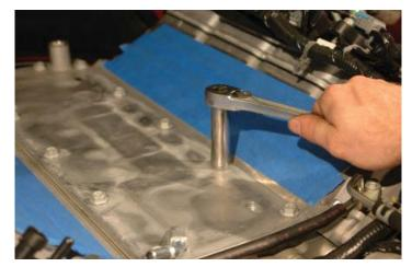
58. Remove the OEM valley cover. This will not be reused, but we will need components. NOTE: L-99 cars or cars with Displacement On Demand (D.O.D.) will retain D.O.D. valley cover, skip to step #62. Damage to engine may occur if MagnaCharger valley cover is installed on D.O.D. equipped vehicles.
