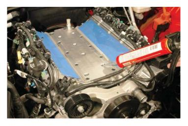
64. Place a dab of some black silicone into the recesses of the top surface of the new valley cover to hold the six provided O-rings in place. NOTE: If your vehicle is L-99 or D.O.D., skip to step 67.
