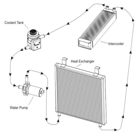
**Intercooler Routing Diagram**
