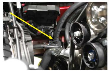
159. Route the hose up parallel to the heater hoses to the outlet barb of the intercooler reservoir. Clamp securely on the reservoir barb using a provided worm gear clamp. This may be made easier by removing the upper end of the fuel line hose to the manifold at the fuel rail temporarily.
