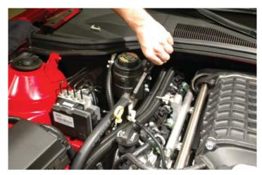
160. Cut off the "U" section short leg of the provided "J" hose. The short end will not be used.
