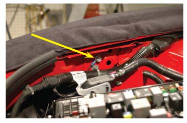
181. Use the fuse removal tool in the fuse center to pull the 5amp IGN fuse from slot 15 of the fuse center.
