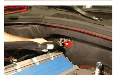
100. Cut the supplied 5/8" hose into a 34" length, and the supplied 3/4" hose into a 35" length if they are not already sized correctly.
