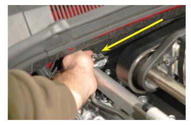
118. Plug in the fuel injector connections to the injectors on each side of the engine. Make sure to route and stuff the wiring to avoid moving components.
