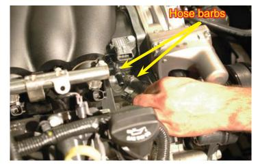
25.LS3 Engines: Disconnect the vacuum brake booster valve from the canister. It will be more out of the way if you swivel this hose behind the intake toward the passenger side of the engine. L99 Engines: Disconnect the hose from the sensor at the brake booster valve using a pair of pliers on the existing clamp.
