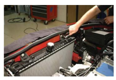
72. Remove the two upper radiator mounting brackets.
