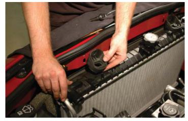
73. Pry off the rubber deflector strip from the top/ front of the radiator. Put these parts aside for later reinstallation.
