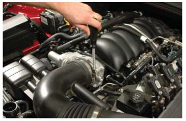
13. Pull the loosened air inlet tube free from the vehicle, this will not be reused.
