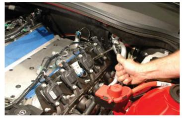
97. Remove the coil brackets from the mounts on the rocker covers on both sides and put on a bench for some required modifications.
