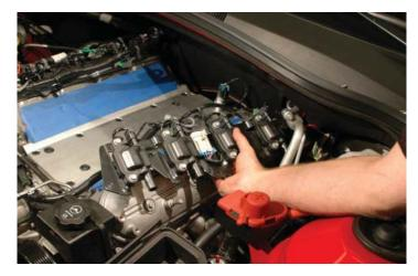
98. The plastic wire loom covers from the coil bracket assemblies must be removed. Unsnap the connecting clips and remove from both sets of coil brackets.
