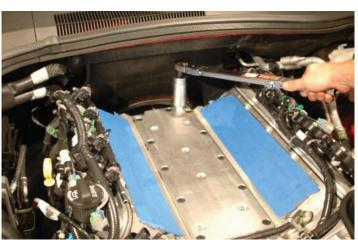
63. If the secondary locking clip lands in position #3, you will need to remove the sensor and reclock it using the supplied copper shim. Before reinstalling, wrap the sensor's threads with teflon tape or teflon paste. Reinstall the sensor and shim into position #1 by torquing to 15 ft-lbs minimum to 24 ft-lbs maximum.
