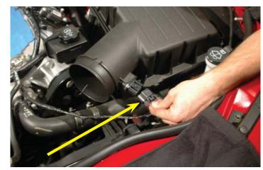
35. Release the two clips on the air-box cover.
