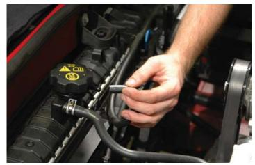
39. Disconnect the steam vent hose from the radiator fill spout, and tuck this behind the power steering pump.
