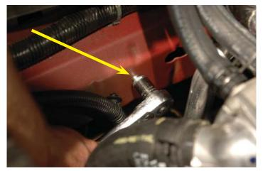
153. There are two ways to approach this. The first way: You place the Intercooler pump in the Adel clamp so that the bolt will be toward the rear. In all cases, the discharge barb points forward and directed toward the outside edge of the fan shroud. Tighten the bolt being careful not to strip the threads. The second way (pictured): Mount the Adel clamp to the frame but do not tighten. Use a mild soap solution (like Windex) to lubricate the rubber of the clamp.
