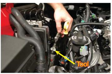
28. Remove the engine cover hold down bracket using a 10mm wrench on the driver side near the end of the fuel rail. Then pivot the hold down bracket up and pull free from the engine. This will not be reused.
