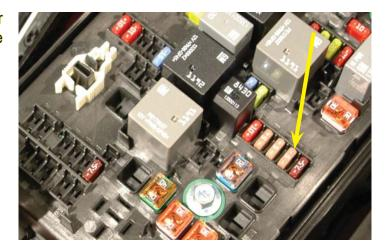
182. Install the provided fuse-tap on one leg of the fuse.
