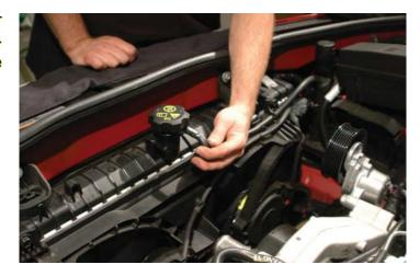
90. Reconnect the steam vent hose to the barb at the side of the radiator neck; place the stock clamp back in position.
