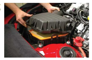
150. Plug the MAF sensor connector at the airbox neck.
