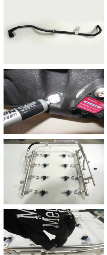
120. Place a small bead of Lubriplate lubricant in the cups of the fuel rail.
