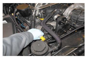
244. Connect the fitting of the "Reservoir to Supercharger" hose to the lower hose barb on the CAC manifold, again ensure the hose clamp snaps into position securely.
