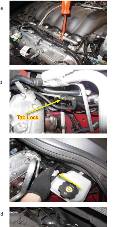
48. Remove the bracket from the engine.
