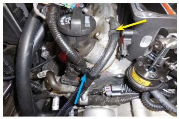
140. The hose from the last step will be routed to the right for now. The opposite end will be attached to the air inlet later in the installation.
