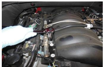
24. Place some shop towels below the fuel line connection on the left hand side of the engine to catch residual fuel.
