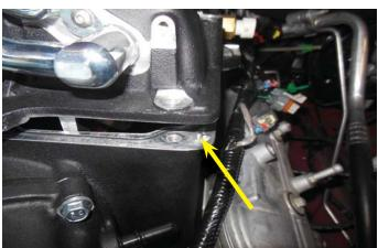
144. These are the supercharger lid mounting bolts, note the four sizes and locate appropriately. Place a small bead of blue Loctite 242 on each of the mounting fasteners. Some of the fasteners will be located in a separate bag with the other sub-assemblies.
