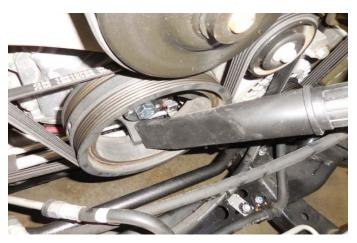
72. Install the reamer bit in your drill motor and ream out your holes. Once again use compressed air to remove debris from the two holes. Now remove the drill key way guide and mounting bolt using a 22mm socket.
