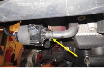
252. Connect the short end of the provided 6.5" by 2.5" length 90 degree hose to the intercooler pump discharge hose barb using a provided spring clamp. Route the long end of the hose to the lower LTR hose barb with a provided spring clamp.
