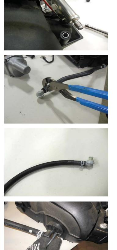
116. This is the line removed from the OEM intake manifold. Save it for later use.
