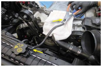
56. Pull up on the harness mounting rings that hold the harness to the water pump hose on the left hand side of the engine.
