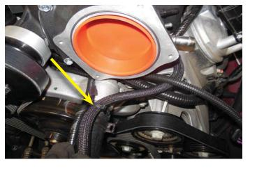
176. Connect the free end of the hose to the hose barb on the left hand side of the radiator fill cap. Secure in place with the remaining black spring clamp provided.
