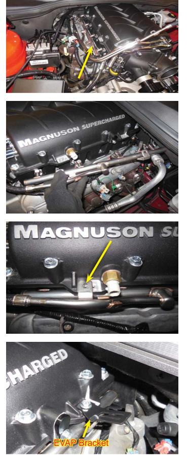
152. Torque the mounting bolts down to 108 in-lbs using a 10mm socket.
