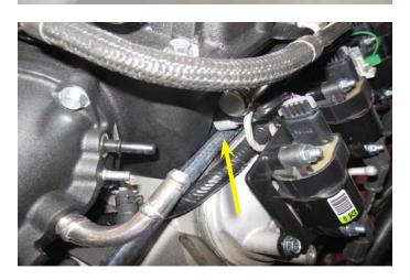
180. Pull the 1/4" diameter 21" length hose out behind the EVAP solenoid and out toward the left hand side fender to gain access as shown.
