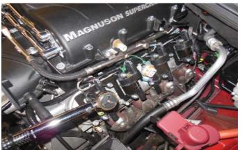
160. Connect the EVAP tube you routed behind the engine earlier to the OEM EVAP solenoid rear barb. Connect the EVAP breakout harness wire electrical connection you also routed behind the supercharger to the EVAP solenoid.
