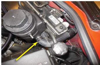
236. Just below the 90° elbow you just connected, route the elbow end of the "Upper LTR to Supercharger" hose out through the opening between the radiator and the vertical frame.
