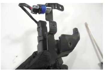
96. Use a small flathead screwdriver to release the tabs locking these covers over the harnesses on the mounting brackets.
