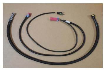
124. Press the EVAP hose extension onto the EVAP hard line on the right hand side of the engine, behind the heat shield adjacent to the capped fuel line.
