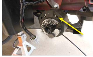
248. Here you can see the modified duct in place with the pump located.
