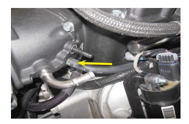
184. Connect the provided vacuum hose between the EVAP solenoid and the hose barb at the top of the supercharger inlet on the left hand side of the engine. Make sure the connections have "clicked" and are locked in place.
