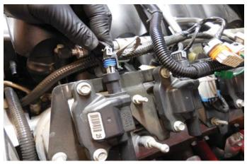
40. Use a 10 mm wrench to remove the harness mounting posts/coil pack mounting bracket screws holding the brackets to the valve cover on each side of the engine. There will be five screws per bracket.
