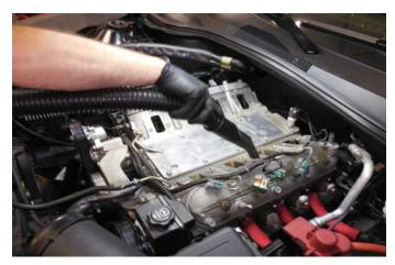
52. Now use a shop towel with denatured alcohol, or some other non-petroleum based solvent to clean around all the intake openings.
