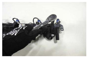
92. This is a separated coil pack set, mounting bolts, and remaining bracket.
