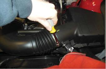
16. Lift up and pull the air supply plenum out of the engine compartment. Set aside in a safe place.
