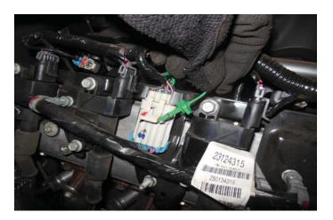
36. Press the release tab and pull the harness connector from the coil pack mounted connection.
