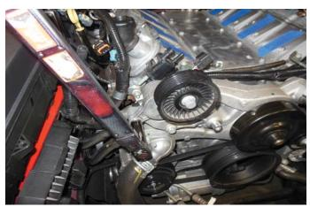
84. Mount the provided Idler pulley with the side showing in the photo facing out using the provided bolt to the boss between the crank pulley and the tensioner pulley.
