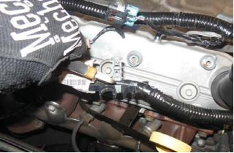
112. Use a small flathead screwdriver to release the injector locking clips from the injectors on the OEM fuel rail.
