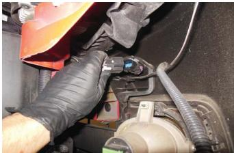
216. Remove the two (one each side) remaining bolts holding the fascia/grille to the vehicle at the top corners, verify everything is disconnected and carefully remove the fascia/grille from the vehicle. The fascia/ grille should simply pull away.
