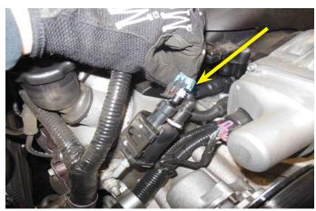
20. Disconnect the remaining tube from the EVAP Solenoid.
