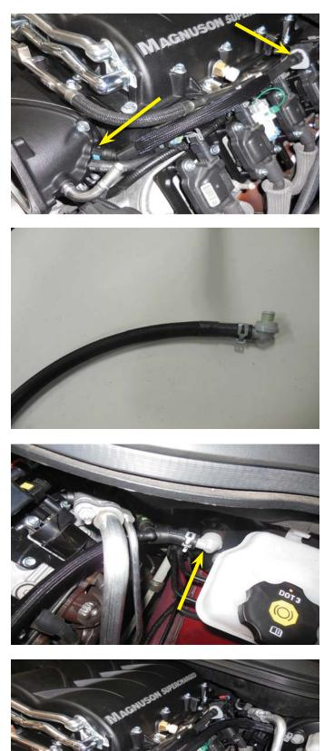
188. Use the provided hose clip to anchor the EVAP solenoid hose to the brake booster hose.
