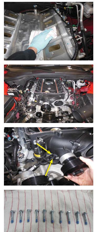
136. Very carefully insert the provided M6 x 40mm supercharger mounting bolts through the holes in the outer ring of the supercharger. It's a good idea to use a magnet tool to avoid the bolts dropping into the exposed ports.
