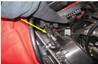
172. Re-connect the OEM radiator hose to the water pump hose barb using the OEM spring clamp. Reconnect the free end of the hose back to the upper radiator hose barb on the left hand side of the radiator using the OEM spring clamp.
