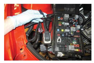
224. Install the provided 15A fuse in the fuse center, and mount the fuse center tab to the stud remaining on the mounting bracket using the provided nut and secure with a 10 mm wrench.
