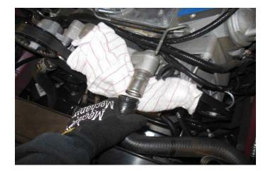
60. Also place towels below the radiator end of the upper radiator hose, remove the clamp and pull the radiator hose off the left hand side, upper radiator hose barb.
