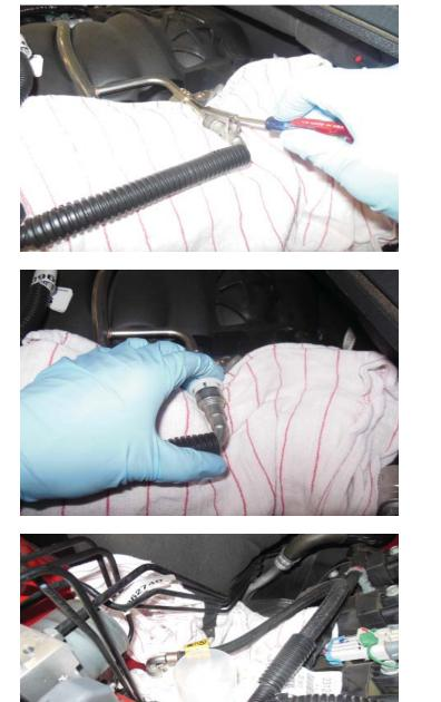
28. Pry out on the safety clip to release the clip from the fuel line/hard line.
