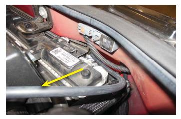
240. Use a provided spring clamp to secure the "Upper LTR to Supercharger" hose 90° elbow of to the upper hose barb on the LTR. Orient the tabs of the spring clamp downward.
