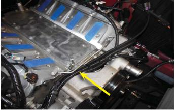
108. Use a pry tool hook to remove the injector harness mounting tie "trees". These will not be reused. You can also cut them off, just be careful to not damage the harness.
