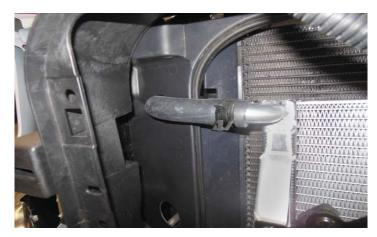
113. Gather the provided cable tie with clip attached. Remove the clip shown in the next step.
