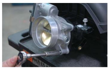
91. Remove the OEM throttle body gasket from the OEM intake manifold. Inspect for damage and clean as necessary. If you have a 5.3L engine this gasket will be re-used.
