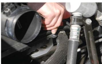
151. Clean up your wiring adding zip-ties as needed to secure the wiring.
