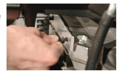
154. Slide the provided 8" section of split loom over the PCV hose and anchor in place at each end using two 1" pieces of the provided heat shrink as shown.
