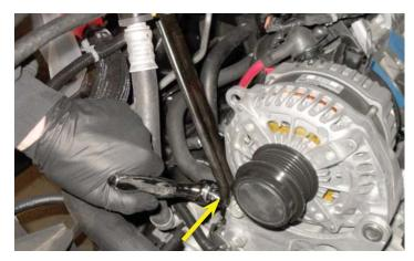
87. Pry the alternator up to rotate it out of the way.
