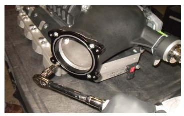
93. Install the OEM throttle body on the supercharger inlet using a 10mm wrench and torque to 106 in-lbs using the supplied 40mm long M6 fasteners.
