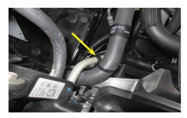
117. Slide the long straight section of the "Pump to Lower LTR" hose through the space shown with the arrow. This will be routed to the output of the pump.
