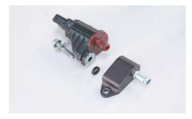
138. Mount the EVAP solenoid mounting bracket to the left side boss on the supercharger lid using the provided 16mm long bolt and secure in place with a 10mm wrench.
