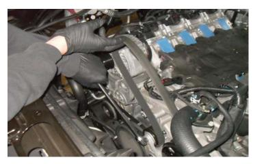
84. Remove the left alternator mounting bolt shown using a 15mm wrench.
