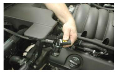
7. Loosen the clamp at the air box securing the air plenum in position.
