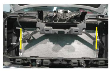
60. Attach the mounting brackets to the LTR mounting flange using the supplied bolts and a 12mm wrench. Do not tighten until you have aligned the LTR to be level, cross checking against the existing horizontal lines of the radiator. Secure in place when you've got proper alignment.
