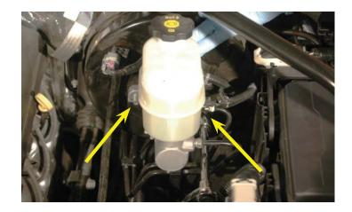
66. Replace the nuts incorporating the reservoir assembly. Torque to 33 ft-lbs. Verify your torque wrench settings.
