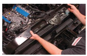
48. Pull up on the upper radiator shroud to unsnap it from the retaining slots, set aside for later re-install.
