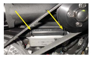
157. Gather the rubber duct shown. Loosen hose clamps to prepare for install. The left side clamp will be taken off completely to install over throttle body.
