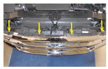
37. Pull straight out on the fascia/grille to disconnect the two remaining snap clips at the center of each side, and the bottom guiding slots. Set the fascia/grille aside carefully for later reinstall.
