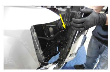
40. Remove the two upper radiator mounting bolts using a 13mm socket.
