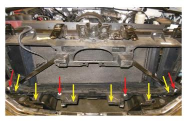
36. Remove the four bolts (shown with arrows) holding the top of the fascia/grille to the sub frame using a 10mm wrench. Also remove the four bolts from the lower portion of the grille that were mentioned in the last step.
