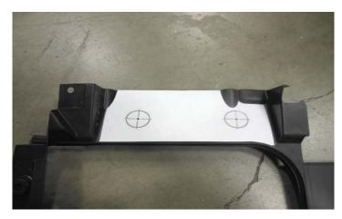
56. Install the two provided grommets at the hole locations. Now re-install the panel back into its original location using the OEM push rivets.
