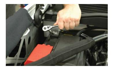
164. Fill the charge air cooler system with the vehicle manufacturer recommended coolant mixture. Have an assistant temporarily key the vehicle on to turn the pump on. Do not start the engine! Key vehicle off after 5 seconds. Fill reservoir full again and continue this process until fluid is circulating. Fill the reservoir to the top of the upper barb. At this time check engine and supercharger for any leaks.
