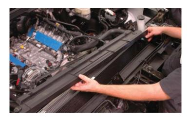
49. Remove the two retainers holding the hood latch release cable as shown with arrows.
