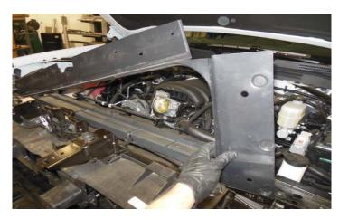
55. Cut out the provided template and install it in the location shown on the panel just removed. Use this template to mark the location for the two holes, and cut the holes out using a rotary tool or knife.
