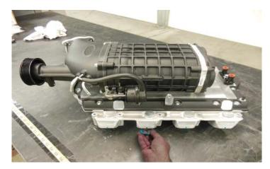
105. Spray a thin film of non-petroleum based lubricant, such as silicone spray or mild dishwashing detergent, on the port mounting surfaces to facilitate aligning and with the help of an assistant, carefully place the supercharger assembly into position.
