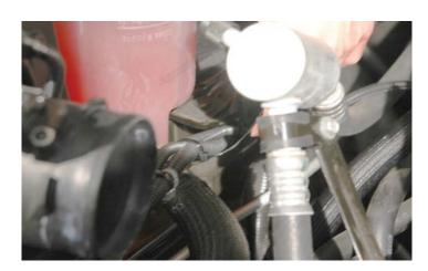
152. Connect the provided PCV hose with the blue colored quick connect locking pin between the existing valley cover hose barb on the left side and forward supercharger inlet hose barb.
