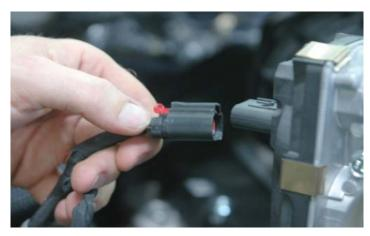
144. Connect the alternator control plug to the receptacle on the alternator.
