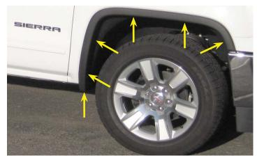
33. In the fender well, use a 7mm wrench to remove the two bolts (on each side of the vehicle) at the front skirt holding the fascia/grille bottom panel to the sub-frame.
