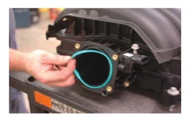
92. Install the throttle body adaptor plate, and torque to 108 in-lbs. Install the throttle body gasket removed earlier in the groove of the supercharger inlet. If the throttle body adaptor provided has a gasket you will not need to use the old one.
