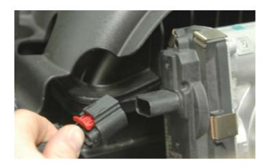
12. Disconnect the alternator control sensor plug from the alternator.
