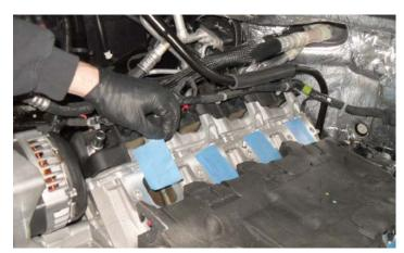
103. Wipe intake port sealing surfaces clean with lacquer thinner, alcohol, or some other non-petroleum based solvent.
