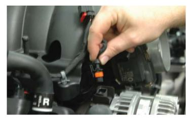
13. Pull the four "tree" tab wire loom mounting anchors from the holes in the right side of the intake manifold.
