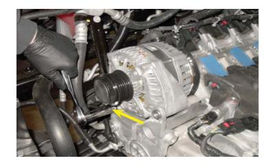
86. Remove the bracket located next to the alternator it will be re-attached later.
