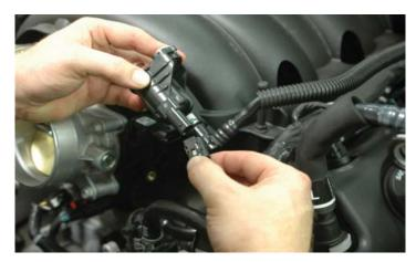
17. With the EVAP Solenoid free, you can now easily disconnect the EVAP tube from the Solenoid by pressing the gray release tab and pulling free. Save the EVAP Solenoid, and its fastener, for a later step.
