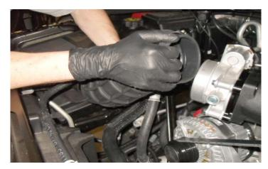
159. Install rubber duct onto throttle body side, and install hose clamp around connection. Make sure duct tabs line up with throttle body indicated with arrow.
