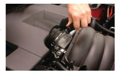
6. Depress the gray locking tab to release the PCV vent hose coming from the valve cover at the air plenum on both sides of the engine. Remove these two hoses for later reinstallation.
