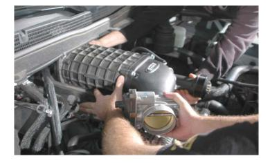
106. Apply blue Loctite 242 to the ten provided 75mm long supercharger mounting bolts. Install supercharger mounting bolts and torque in position to 106 in-lbs using a 10mm wrench. Follow the torque order given at the back of the book. At this point also reinstall the bolt holding the fuel injection line to the left side of the engine that was removed earlier.
