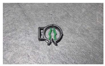
115. Here you can see the two tabs on the left that have been removed from the clamp on the right. Reinstall this clip onto the cable tie.
