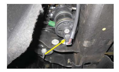
126. Secure the pump harness to the existing harness using the provided cable ties.
