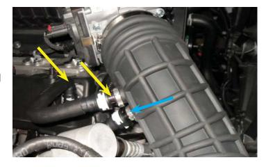
162. If you disconnected the reservoir overflow hoses earlier, reconnect using the OEM clamps. Ensure that you remove any plugs that you may have installed on these hoses.
