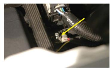
135. Connect the black ground wire "eye" terminal to the existing grounding bolt at the firewall on the left hand side, just above and inside the brake booster canister.
