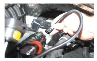
140. Connect the provided 10" x 3/8" PCV hose between the EVAP solenoid and the supercharger inlet hose barb. No clamps are required. Adjust hose length to prevent rubbing on supercharger bolt head.
