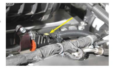
142. Connect the MAP sensor plug to the connector on the MAP sensor.
