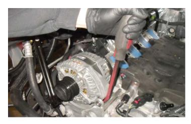
88. Alternator shown rotated out of the way.
