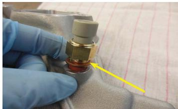
97. Once the sensor is snug to the crush washer, set your torque wrench to 175in-lbs (~15ft-lbs). With a 19mm (or ¾") deep socket attached to your torque wrench, torque the sensor down.
