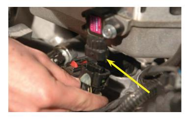
143. Connect the throttle body plug to the throttle body.
