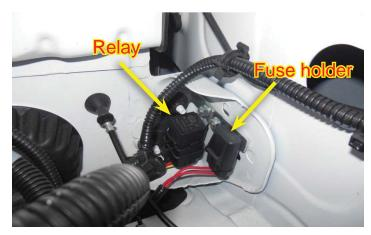
125. Route the plug from the wiring harness down to the inside of the fuse center, along the existing wiring harness and plug into the intercooler pump connector.
