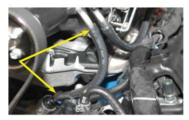
153. Push the two provided zip-tie "tree" connectors into the two bolt holes in the front of the supercharger intake manifold. The flat part of the connector should be pointing up.
