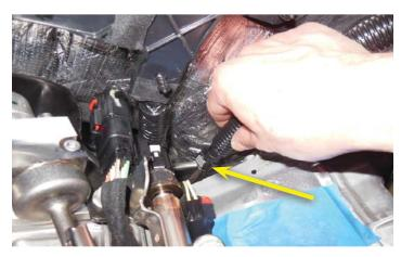
101. Connect the gray end of the new provided EVAP hose shown to the location where the factory EVAP hose was just removed (shown with a yellow arrow). Remove the bolt holding the fuel injection line in place (shown with a green arrow) to allow clearance while the supercharger is being installed. This bolt will be reinstalled after the supercharger is mounted.
