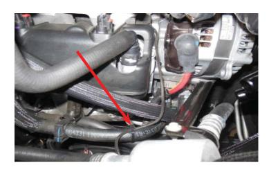
148. Continue to pass the MAF/IAT breakout harness to the right underneath the AC line. Secure the MAF/IAT breakout harness with another tie wrap to the factory MAF harness as shown by the red arrow to the right. \*Note: The green arrow is a reference to the fie wrap installed in the previous step.
