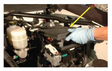
128. Cut a small slot in the back lip of the fuse center tray as shown.
