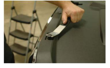
32. Remove the front wheel well fender trim from both sides by removing the 6 bolts located around the perimeter.
