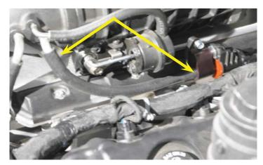
141. Connect the opposite end of the supplied EVAP hose, that was connected to the rear of the left hand side head where the factory hose was removed earlier, to the EVAP solenoid where shown with the arrow. The yellow locking clip end goes to the solenoid, and the gray locking clip end goes behind the cylinder head. Ensure that both "click" into locking position.
