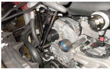
109. Install the provided accessory drive belt using the drive belt routing diagram. A larger diagram is included at the back of this book.
