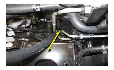
118. Route the end of the "Pump to Lower LTR" with the 90° bend through the hole made in the plastic cover earlier (shown with an arrow).
