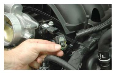
15. Use a 10mm wrench to remove the EVAP Solenoid from the intake manifold. This is located just behind the throttle body on the left side, below the MAP Sensor.
