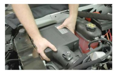
146. Plug the IAT end of the MAF/IAT breakout harness into the sensor. This can be done after the installation of the supercharger (as shown), or you can pre-install the harness and take extra precaution to not damage the connector during supercharger installation. If you choose to connect the sensor post install, it may be helpful to swing the alternator out of the way, as shown to the right.
