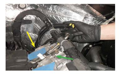
102. Remove the tape or rags covering the intake ports on the heads. Be careful to not allow any debris to fall into the exposed ports.
