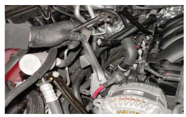
11. Disconnect the ETC connector from the throttle body. Depress the locking tab and pull the connector free.
