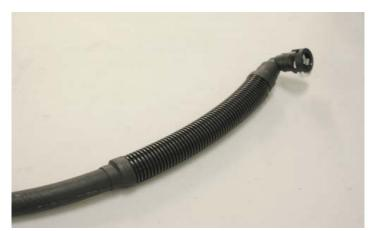
155. Connect the 90° hose barb on the uncovered side of the PCV hose to the left hand side front of the valve cover hose barb. Route the hose under the supercharger inlet toward the right hand side of the vehicle. The split loom covered section of the hose should be on the right hand side above the alternator.
