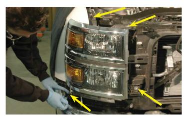
39. Lift up carefully on the headlight to separate it from the frame and disconnect the wiring harness plug (shown at the yellow arrow location) by pressing the release tab and pull it free. Set the headlight aside in a safe spot to be reinstalled in a later step. Repeat the removal process on the left side headlight.
