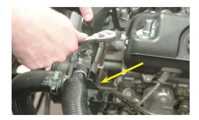
22. Remove the three harness "tree" clamps from the left side of the intake manifold.
