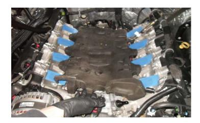
83. Remove the OEM drive belt by springing the tensioner using a ½" breaker bar or socket wrench. If necessary utilize a piece of pipe to extend the lever length. This belt will NOT be reused.
