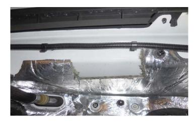
100. Remove the factory EVAP hose from behind the left side cylinder. Squeeze the connector clip to release the clip and pull free.
