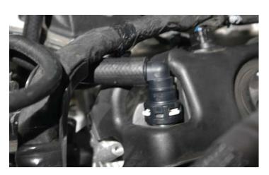
156. Anchor the PCV hose to the front of the supercharger intake manifold using the installed zip-tie tree mounts.
