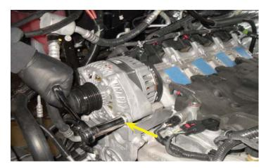
85. Loosen the other alternator support bolt shown.
