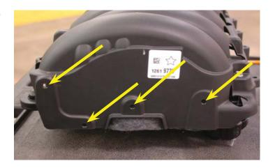
26. Pull the OEM intake manifold out of the vehicle and set aside. Parts will be used from this assembly. Gaskets, and throttle body will be reused.
