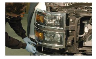
166. Replace the fascia/grille in position and push on the center of each side grille opening to reconnect the two snap clips, and the bottom guiding slots.
