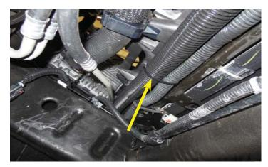
121. Install the end of the "Pump to Lower LTR" hose to the output side of the intercooler pump and secure in place with a provided worm gear clamp.
