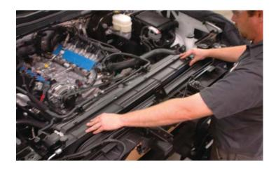
62. Replace the upper radiator cross-frame brace and secure with the OEM mounting bolts.
