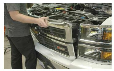
167. Replace the four bolts holding the top of the fascia/grille to the sub frame and the four bolts on the underside of the grille using a 10mm wrench.
