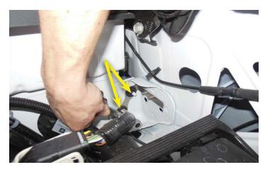
124. Place the relay on the stud closest to the firewall and secure with a supplied 6mm nut, using a 10mm socket. Use the remaining supplied 6mm nut to secure the fuse holder to the bracket. Make sure to route the wires to the fuse holder as shown, so that they do not rub on the sheet metal below.
