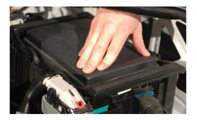
134. Remove the nut of the hot lead at the back of the fuse center using a 12mm wrench. Replace the nut incorporating the "eye" terminal on the red wire from the intercooler wiring harness.
