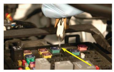
129. Remove the fuse number 3A (labeled: MISC IGN) from the slot in the fuse center.
