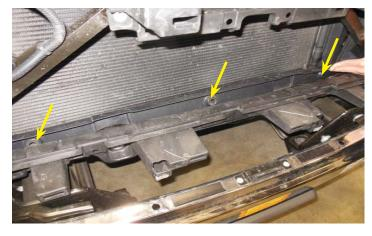
53. Once the rivets have been removed you will have to pull the sides of the panel inward to release them from their locations as you pull upward. Be careful not to damage any radiator fins while you remove this panel.
