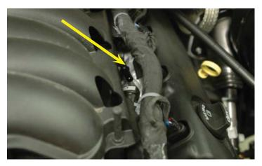
20. Use a 10 mm wrench to remove the nut holding the wire harness to the base of the bracket in front of the left side valve cover.
