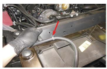
51. Remove the plastic push rivets from the plastic panel that is located around the radiator. This is the same shroud that retainer clips were removed from in the last two steps. There are 3 push rivets on top, 2 on each side, and 3 on the bottom. All the rivet heads are hidden from view in this photo. The top and bottom rivets are located on the back sides of this panel.
