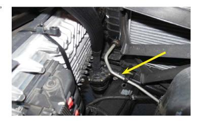
122. Install the provided fuse in the charge air cooler pump wiring harness fuse holder, and replace the cap.
