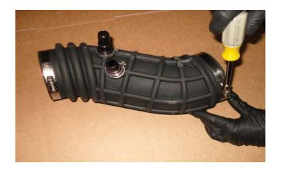
158. Install the rubber duct from previous step on the air box. Apply Lubriplate grease to the side near the throttle body to help it slide better.
