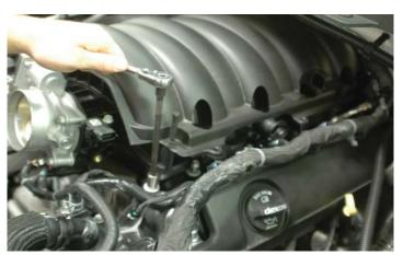
24. Pull the intake manifold forward a bit to gain access to the wiring harness "tree" anchors that hold the harness to the back of the intake manifold. Use a screwdriver or tree clamp remover to unplug these trees from the OEM intake manifold.
