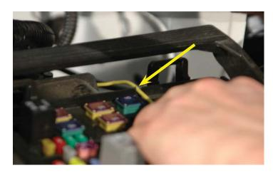
133. Replace the cover on the fuse center engaging the snaps. The lid should NOT be crimping down on the yellow wire.
