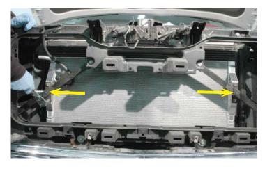
61. Replace the upper radiator shroud by snapping into place.
