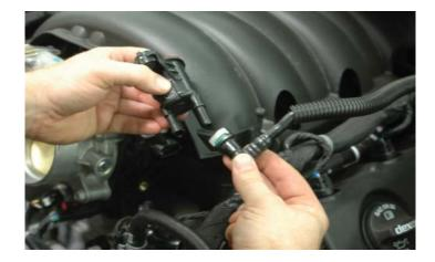
18. Remove the PCV hose from the valley cover on the left side below the throttle body.
