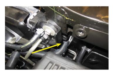
112. Connect the hose from the last step that came from the right side of the charge air cooler to the upper LTR barb and secure with a wide band spring clamp. Secure the hose along its path with a few provided zip-ties.
