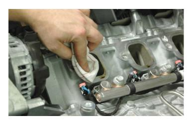
104. Remove the OEM O-ring gaskets from the intake manifold, clean, inspect and install in the grooves on the bottom of the supercharger intake manifold. If you find any damage you will need to replace the O-ring gaskets with GM replacement parts. The tab will line up with the slot on the outside edge.
