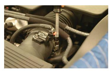
8. Remove the air intake plenum from the vehicle. This will not be reused.
