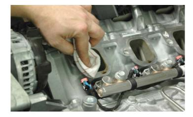
30. Use tape or clean shop towels to cover over your intake ports. It's important to keep these ports clean and avoid any debris falling into the exposed openings.
