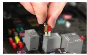
131. Replace the fuse in slot number 3A (labeled: MISC IGN) with the fuse tap installed on one leg.
