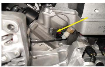
147. Route the MAF/IAT breakout harness behind the alternator. Make sure the harness will not get pinched by the alternator. Use a tie wrap to secure the harness to the factory heater hose as shown by the red arrow to the left.
