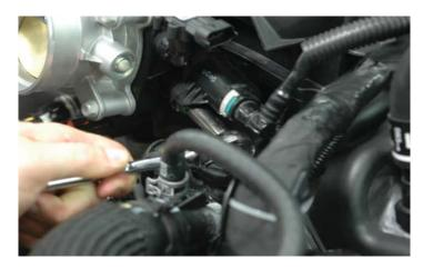
16. With the EVAP Solenoid free you can now remove the electrical connection by pressing the release tab and unplugging.
