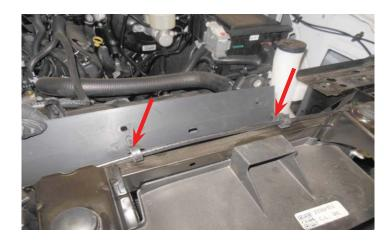
50. Remove the retainer holding the wiring harness shown with an arrow.
