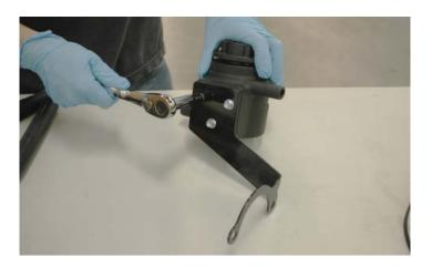
65. Remove the two nuts holding the master cylinder to the brake booster canister using a 15mm socket.
