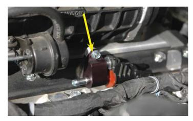
139. Connect the extended EVAP solenoid plug to the EVAP sensor. Secure the extension harness to the coil pack harness with a few of the provided zip-ties.
