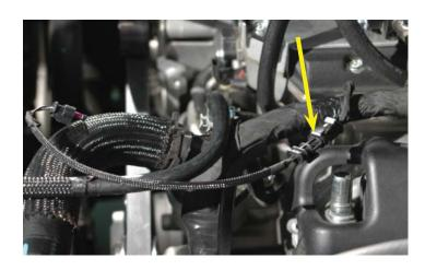
137. Mount the OEM EVAP solenoid to the provided mounting bracket using the factory mounting bolt and provided spacer using a 10mm wrench as shown. Add blue Loctite 242 to this fastener.
