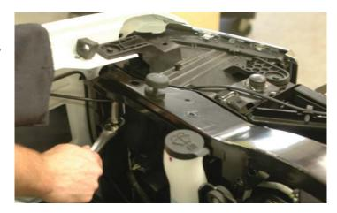
46. Remove the cross-frame support brace center bolt using a 13mm wrench.
