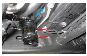
75. Refer to the expanded diagram at the end of the instruction manual to prepare your intercooler system plumbing hoses for install. When measuring the mesh sleeve make sure it is in a relaxed state.
