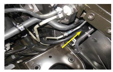
119. Connect the hose from the last step to the lower LTR barb and secure in place with a provided wide band spring clamp.
