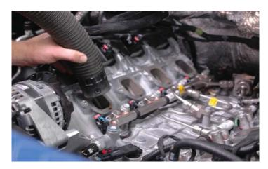
29. Use denatured alcohol, lacquer thinner or some other non-petroleum based solvent to wipe the surfaces of the head intake ports.
