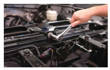
47. Pull the cross-frame support brace from the vehicle and set aside for re-install in a later step.
