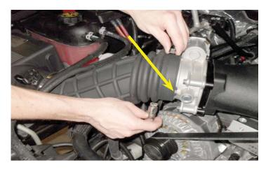
160. Tighten the hose clamps on both sides.
