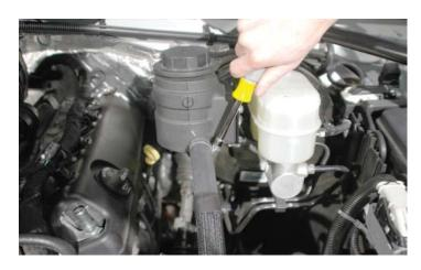
77. Route the other end of the hose from the last step forward and down to connect to the intercooler pump inlet hose barb using a provided wide band spring clamp.
