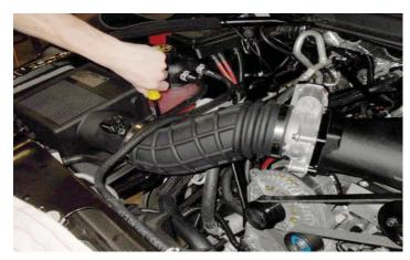
161. Connect the free end of the PCV hose from the left hand side front valve cover hose barb onto the lower hose barb of the air tube (Indicated with a blue arrow). Connect the provided 90° PCV hose between the hose barb on the right hand side front of the valve cover and the remaining upper hose barb of the air tube as shown.
