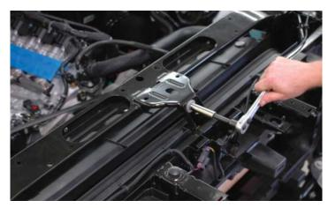
63. Replace the upper radiator mounting bolts and vibration dampers.
