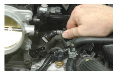
19. Rotate the hose approximately 180° to gain access to the release tab on the left side valve cover, depress the tab and pull the hose free from the vehicle. Set aside for later usage.
