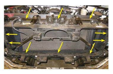
52. Here you can see the three lower locations after the rivets have been removed.
