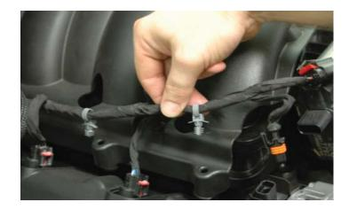
14. Unplug the electrical connector from the MAP sensor. Release blue locking tab first.
