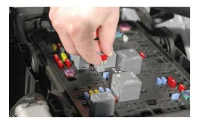
130. Connect the fuse tap end of the yellow wire from the intercooler wiring harness to one leg of the fuse just removed.
