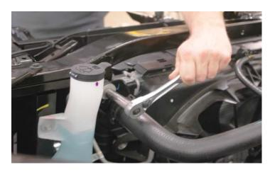
41. Remove the two upper-forward, diagonal fender-brace bars using a 10mm wrench.
