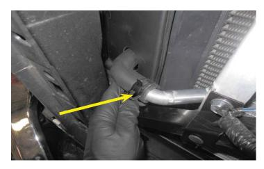
120. This view is from under the vehicle looking to the left front. Run the opposite end of the "Pump to Lower LTR" hose behind the lower portion of the radiator as shown and secure in place with provide cable ties as shown with the arrow.
