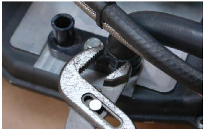
96. Connect the short end of the other modified 4" x 36" x 90° elbow hose to the left hand side charge air cooler hose barb behind the supercharger using a provided spring clamp. This hose will also route toward the right hand side of the vehicle.
