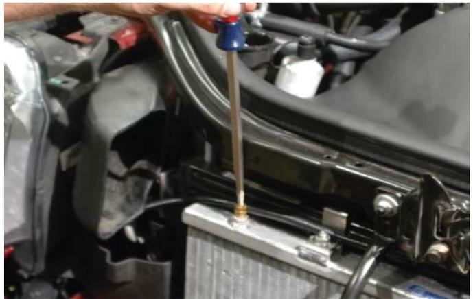
198. Fill the radiator back up with the fluid drained earlier. Be sure to incorporate a filter in case any debris contaminated your fluid. Top off as necessary.
