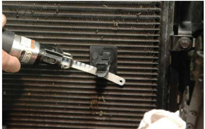
70. There is an existing threaded hole in the top surface of the bumper support on the left hand side. Use a drill motor and drill bit to open this hole to 1/4".
