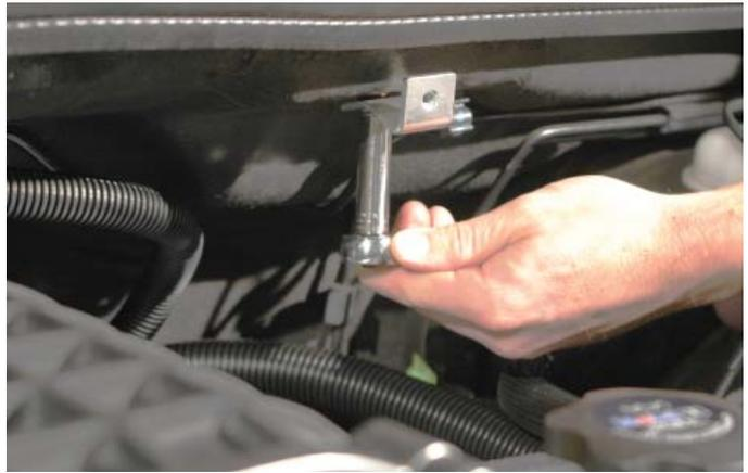
113. Use the provided Adel clamp and bolt to attach the oil separator to the bracket just installed using a 10mm wrench. The embossed arrow on the top of the valve points toward the left hand side fender. Once installed, twist the left hand side barb to point down and the bottom barb to point toward the oil fill spout.
