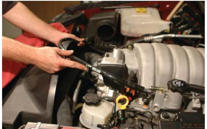
26. Disconnect the EVAP hose from the left hand side of the manifold, just behind the throttle body.
