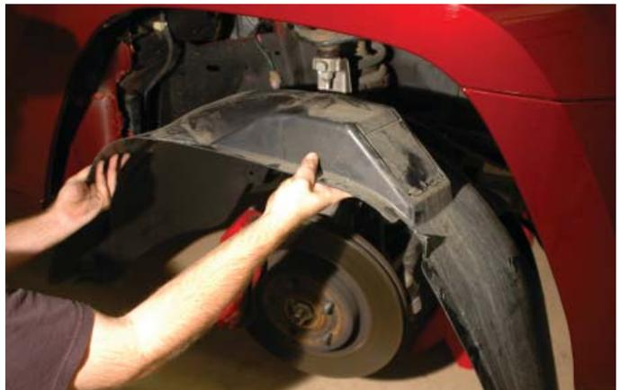
128. Mark a hole  $\frac{3}{4}$ " down from the center of the vertical-to-horizontal bend of the fender cross brace.
