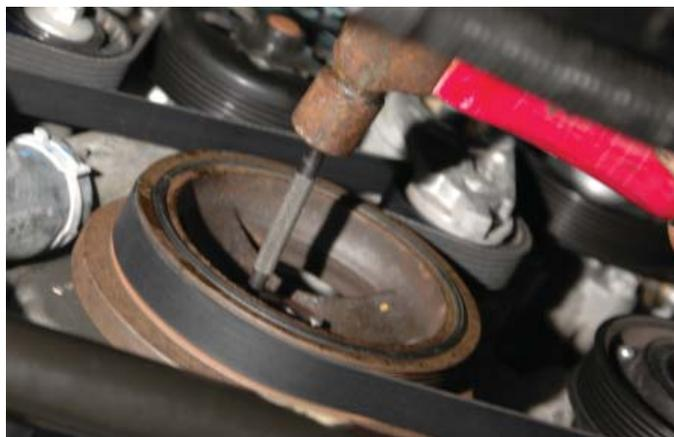
194. Install the OEM crank pulley bolt and torque to 129 ft. lbs.
