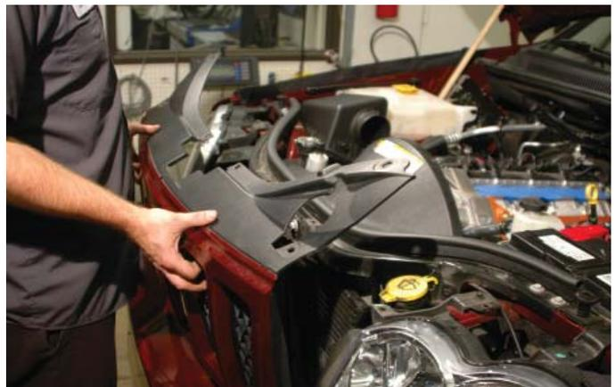
64. Cut strips of the supplied adhesive backed rubber and apply to the inside surfaces of the low temperature radiator mounting brackets, on top of the strips applied, cut and add the ½” adhesive backed rubber as shown.
