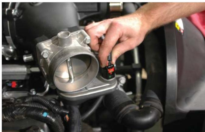
105. Plug the EVAP sensor tube onto the inlet on the supercharger inlet as shown.
