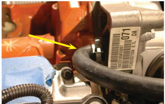
51. Route the hose toward the right hand side fender. Use the bolt hole at the front of the right hand side head near the water pump, add the supplied spacer, then the Adel clamp with the lobe up and pointed toward the rear of the vehicle, and the supplied bolt to anchor the heater hose as shown in this picture.
