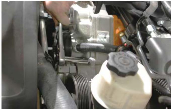
174. Replace the second water pump bolt (you just removed) incorporating the supplied idler bracket as shown. Fingertighten the bolt at this time.
