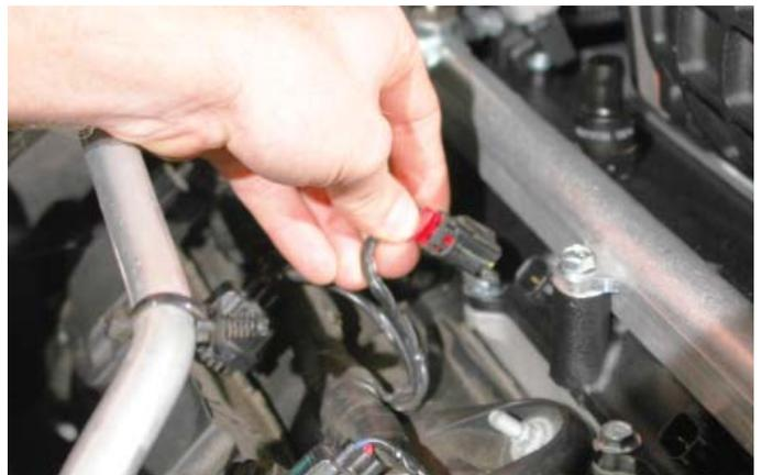
103. The IAT extension harness should be exiting below the supercharger intake manifold assembly on the right hand side of the engine. Connect the extension to the existing IAT plug and tuck the wires under the throttle body upon completion.
