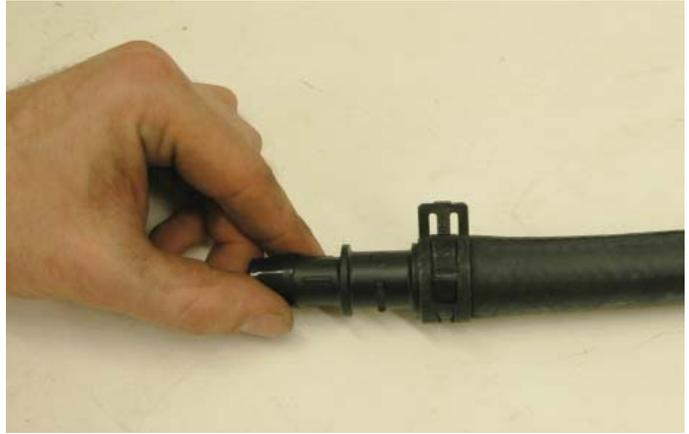
53. Use the stock clamp removed from the OEM heater hose removed earlier to attach the 7" piece of hose to the center-most heater barb at the firewall on the right hand side of the engine compartment.
