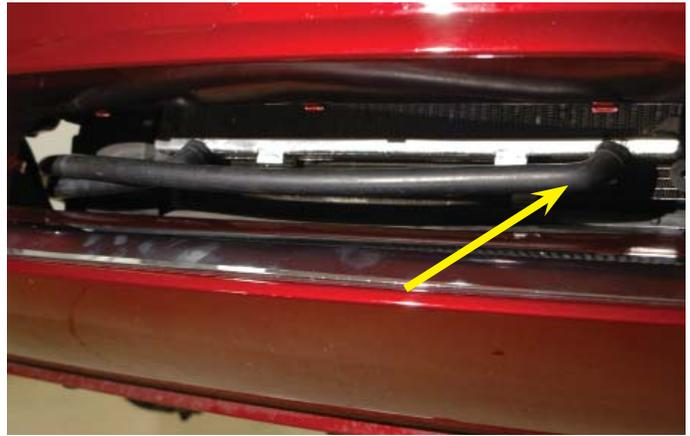
137. Cut the hose to fit and connect to the charge air cooler pump discharge barb using one of the provided spring clamps.
