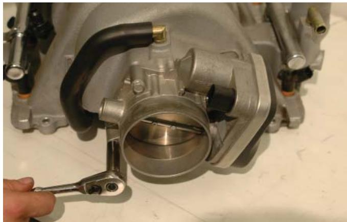
86. Inspect the installed throttle body O-Ring on the new supercharger inlet. If there is any nicks or damage to the O-Ring it must be replaced.
