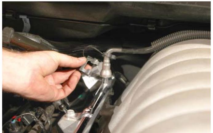
28. Use shop rags to catch residual fuel and the fuel line removal tool to disconnect the fuel line from the right hand side fuel rail. First press the fuel line further onto the fuel rail barb, then push the fuel line removal tool into the fuel line to release the locking clip. Now pull the fuel line free. **We recommend plugging the fuel line and capping the fuel rail barb. Clean up residual fuel using shop rags and dispose of the contaminated rags properly.**
