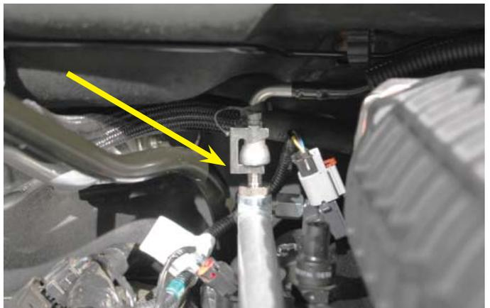
111. Extend the 'lobe' of the notch in the left hand side coil pack cover approximately 1" further toward the rear of the cover and press in place over the coil packs in the original location. This modification is to create clearance with the oil separator drain hose to be installed next.
