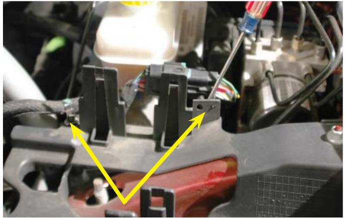
13. Use a 10mm wrench to remove the three nuts holding the fuse center mounting bracket to the strut tower/interior tire well studs.
