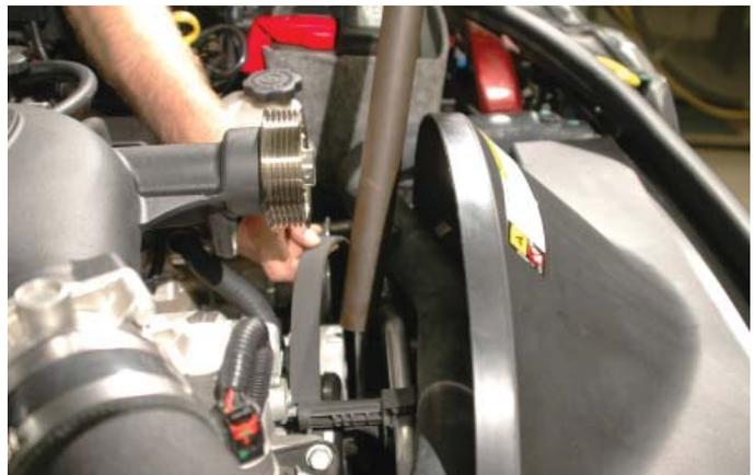
171. Remove the top water pump bolt using a 13mm wrench.
