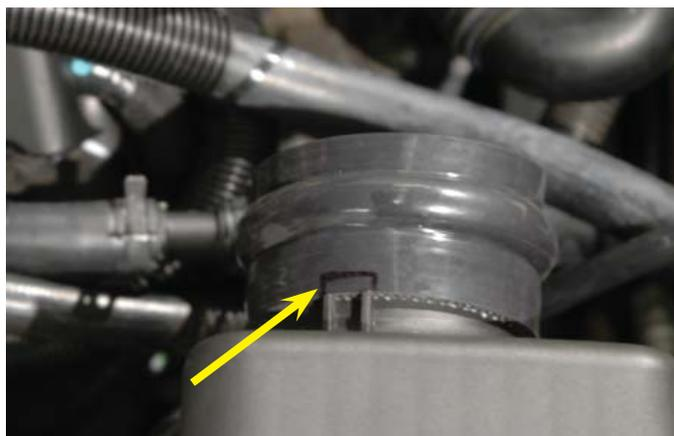
168. Install the notched hose in place on the air box. Slide the other hose completely onto the new air tube throttle body end. Press the air box end of the air tube into the receiving end of the hump hose...rotate the air tube to fit and slide the straight hose onto the throttle body. Tighten all clamps securely.
