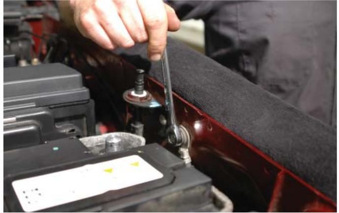
161. Route the black wire from the relay harness over toward the ground bolt. The existing “eye” terminal is not large enough to fit over the ground bolt. Cut the “eye” terminal off, strip off 3/8” of insulation from the end and crimp on the new “eye” and crimp on securely. Replace the ground wires and bolt incorporating the new black ground wire from the relay harness. **Ensure that you have ALL the ground wires attached.**
