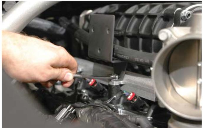
142. Modify the OEM right hand side coil pack cover to create clearance with the throttle body, slide under the charge air cooler reservoir mounting bracket and press onto the mounting studs locking in place.
