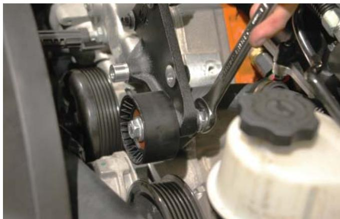
178. Install the second idler pulley using the supplied bolt. Use a 14mm wrench and torque the bolt to 40 ft. lbs.
