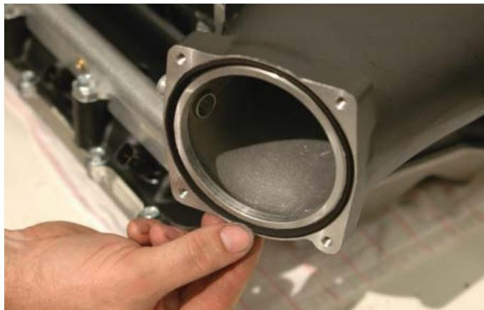
87. Install the throttle body on the new supercharger intake with the motor pointing down. Use the stock bolts removed from the OEM manifold and torque to 106" lbs. Verify your torque wrench settings.
