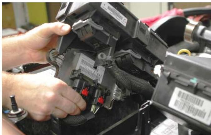
120. Install the forward fuse center onto the three fuse center mounting bracket posts. An audible click is heard when locked in place.
