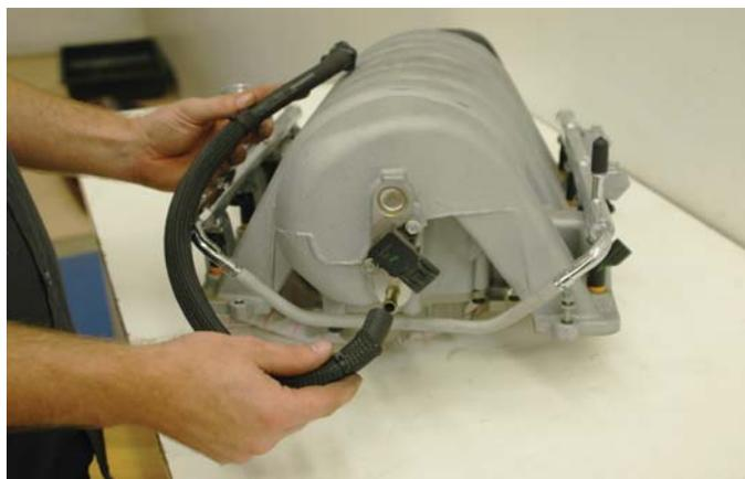
107. Remove the brake booster valve from the end of the hose and re-connect the valve to the opposite end of the hose by the "J" bend.
