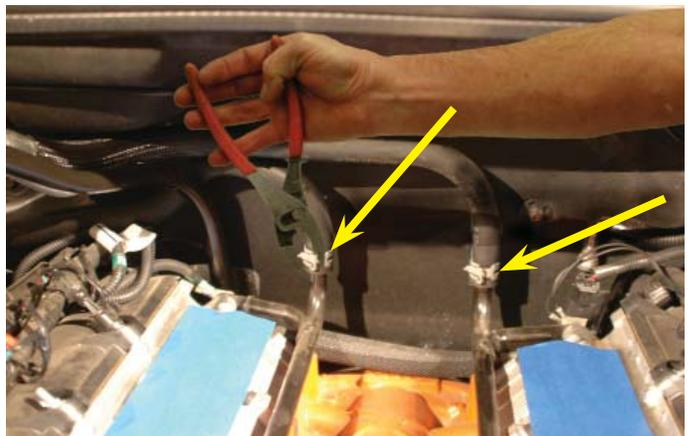
35. Disconnect the two heater hoses from the hard line barbs. There will likely be some residual coolant in the hoses and tubes, so take appropriate precaution and dispose of contaminated shop towels properly.
