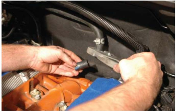
57. Install the provided 5/8" 90° elbow on the end of the hose you just cut. Secure the elbow on the hose so that the open end points toward the left hand side fender and the handles of the hose clamp point toward the right hand side fender.
