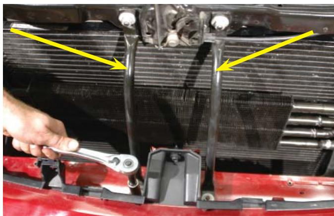
67. Use pinch off pliers or (carefully) vice grips to clamp off the two power steering hoses prior to the power steering cooler.
