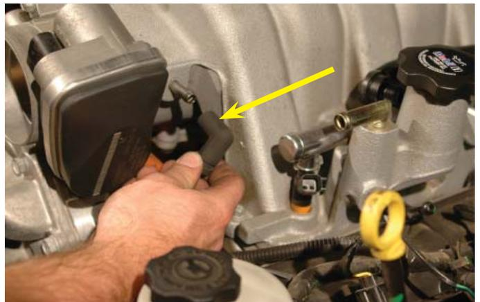
27. Remove the fuel line safety clip. Set aside for later.
