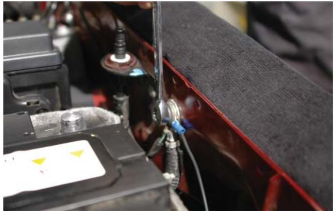
162. Cover the black ground wire with a length of the supplied split loom.
