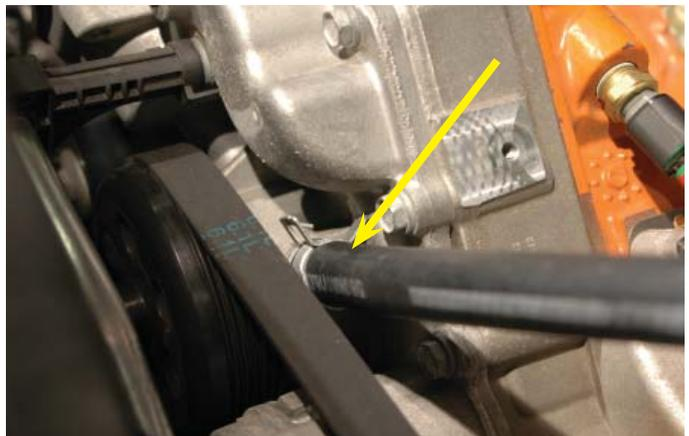
59. Use the bolt hole on the front of the left hand side head, the supplied spacer, then Adel clamp and bolt to anchor the hose you just installed to the engine. The lobe of the Adel clamp should be pointing up and toward the front of the vehicle.
