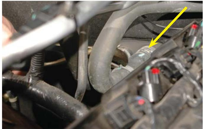
50. Cut 2-1/2" off the short end of the supplied 4" x 48" x 5/8" 90° elbow hose and attach the short end to the barb just installed on the right hand side of the water pump using a provided spring clamp.
