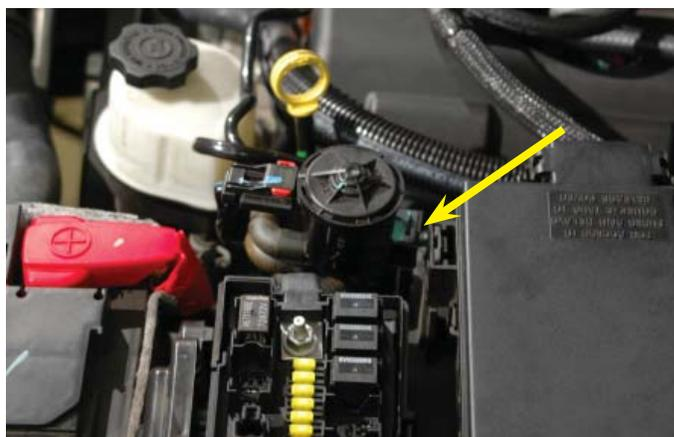
123. This is the charge air cooler pump and mounting hardware.
