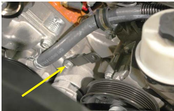
175. Attach the supplied idler bracket to the top water pump bolt location and the supercharger pulley support using the provided bolts. Torque to 20 ft. lbs.
