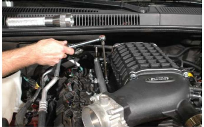
101. Connect the MAP Sensor plug onto the MAP Sensor located on the right hand side behind the supercharger.
