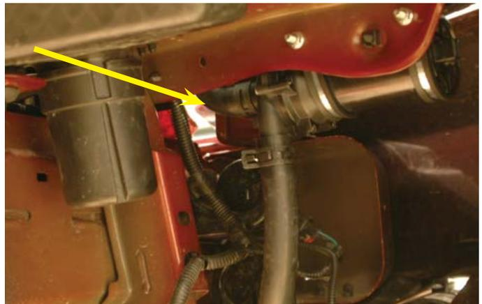
140. Remove the forward right hand side fuel rail mounting bolt using a 10mm wrench.
