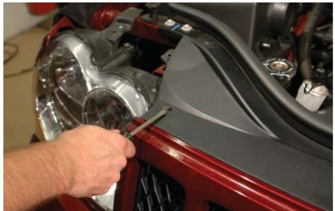
63. Pull forward and up to remove the fascia grille. Set aside in a safe location for later re-install.
