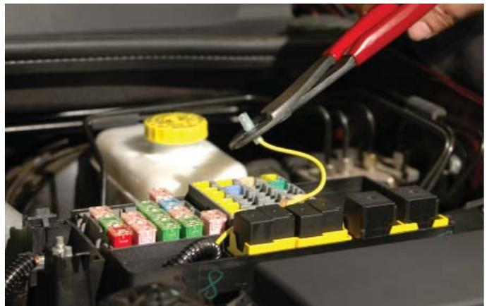
159. Route this wire over to the fuse tap just installed and plug the spade end onto the fuse tap. Bend the wire over toward the center of the box and close the cover.
