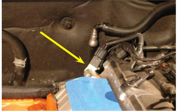
45. Replace the right hand side ground wires to the head using the original stud. Make sure you have accounted for all the wires.
