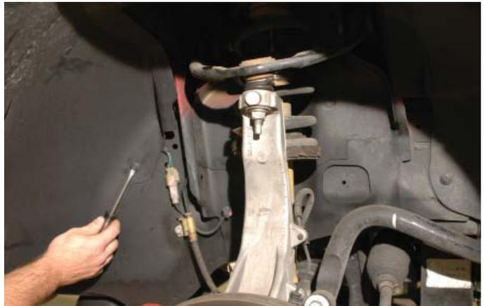
126. There are five plastic 'pop' rivets. Use an awl or tiny screwdriver to push in on the center post of the rivets to release the lock, the rivets can then be pulled free.
