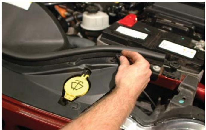
200. Find a place to loop the cable of the OBD port (a panel behind the port can be opened and the cable looped around the wire harness inside) and press the cover over the port.
