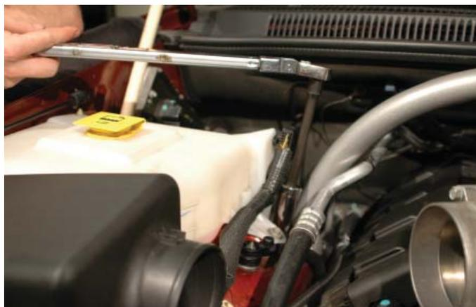
118. Install the fuse center mounting bracket using the original three nuts and tighten using a 10mm wrench.
