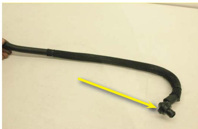
108. Connect the brake booster valve to the brake booster canister and route the hose forward to connect to the hose barb on the supercharger inlet as shown.
