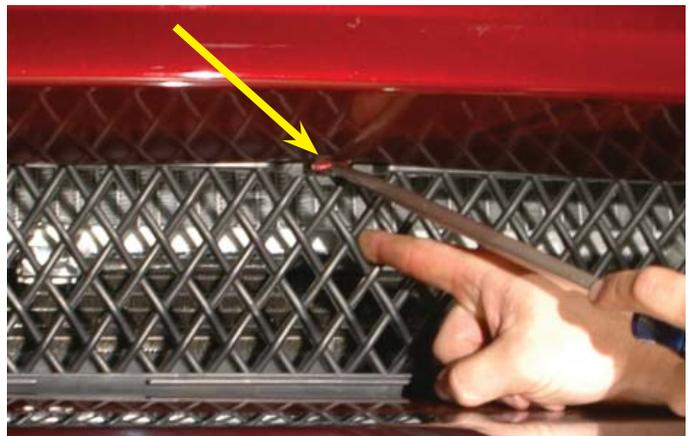
75. Place the remaining low temperature radiator mounting clamp on the bottom left hand side of the low temperature radiator, hooking over the bottom tank of the air conditioning condenser and secure in place with the remaining carriage bolt and nut.
