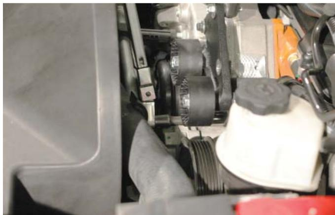
180. Tighten the OEM tensioner assembly back down using a 15mm wrench to 20 ft. lbs.
