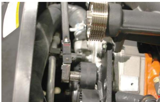
179. Torque the second water pump bolt (finger-tightened earlier) using a 13mm wrench and torque to 20 ft. lbs. Always verify your torque wrench settings.
