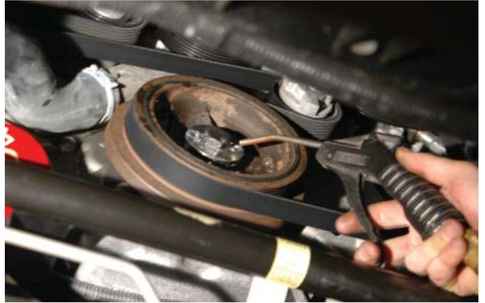
189. Ream out the two holes using the provided reaming bit.
