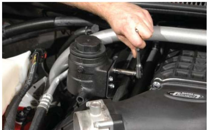
144. Route the hose from the charge air cooler pump inlet barb to the forward barb of the charge air cooler reservoir bottle. Tie the hose down to the existing harness below the throttle body using a supplied zip-tie, cut the hose to fit and secure to the reservoir bottle using a supplied worm gear clamp. **NOTE: It's important to use worm gear clamps on the reservoir bottle.**
