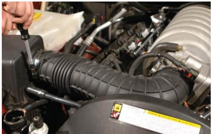
19. Remove the intake air tube from the vehicle. This will not be reused. There is a PCV vent tube running from the air box to the oil fill spout, this has a soft mounting clip on the intake air tube. Be careful to not damage the PCV vent tube.
