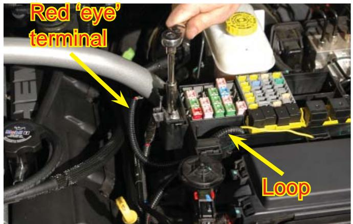
154. Replace the nut incorporating the "eye" on the end of the red wire of the relay harness.
