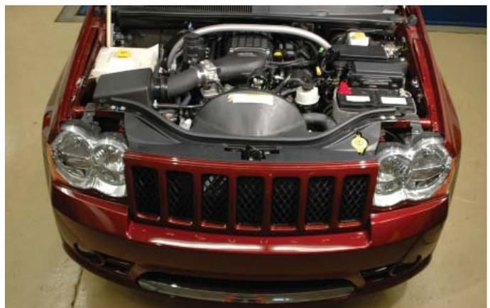
204. Test drive the vehicle for the first few miles under normal driving conditions. Listen for any noises, vibrations, engine miss fires or anything that does not seem normal. The supercharger does have a slight whining noise under boost conditions, this is normal. Also during the supercharger break-in, the rotors are self-honing, the noise will reduce quickly.
