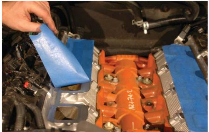
98. Wipe any tape residue or debris off using lacquer thinner or alcohol or some other suitable non-petroleum based solvent.
