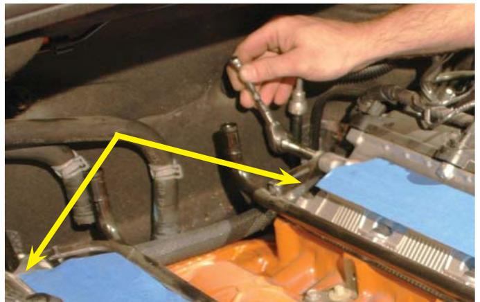
39. The left hand side heater hard line has two additional mounting bolts. Use a 10mm wrench to remove the center mounting bolt from the middle of the valley.
