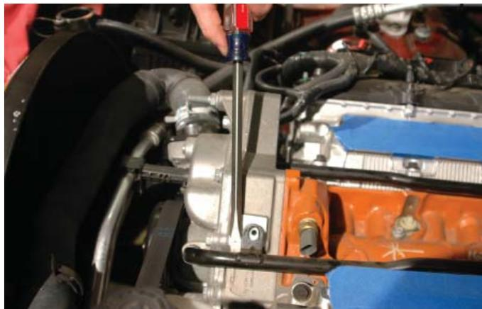
43. On the right hand side the heater hard line needs to be pulled toward the rear to remove it from the water pump. Use the large screwdriver with the head as a fulcrum to lever the hard line free from the water pump.
