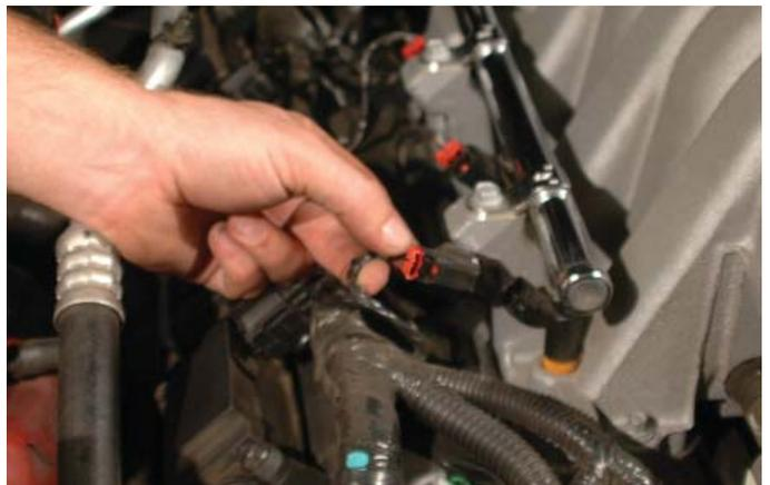
23. Disconnect the MAP sensor from behind the air intake manifold on the right hand side behind the OEM manifold. If you cannot get this unplugged easily, you will have another chance while you are removing the OEM manifold a little later in the instructions.
