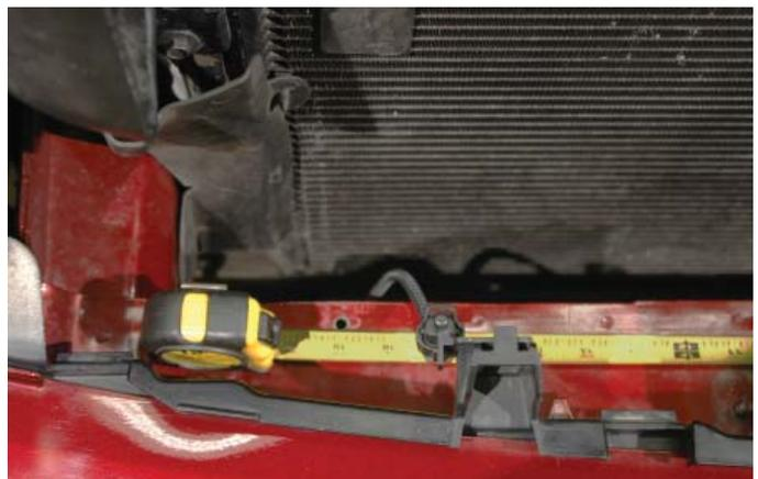
72. Slide the two carriage bolts into the slots of the charge air cooler low temperature radiator and place the low temperature radiator just in front of the air conditioning condenser on top of the bumper support. Use the location of the two bolts to locate where to place two of the prepared charge air cooler low temperature radiator mounting brackets. Press the mounts into position on the air conditioning condenser top tank.
