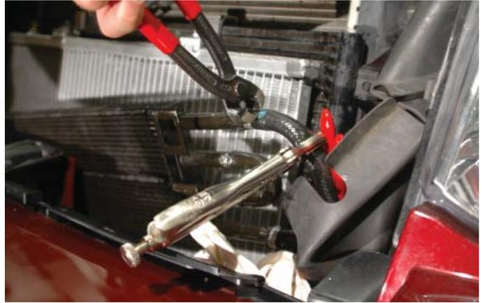
77. Remove the pinching pliers or vice grips from the two power steering cooler hoses. Attach the supplied acute (below 90°) angle mounting bracket to the right hand side, lower power steering bracket with the angle being up leg pointing forward. Use the supplied threaded plate as backing with the supplied bolt. Align the backing plate flush with the top of the bracket and tighten securely.
