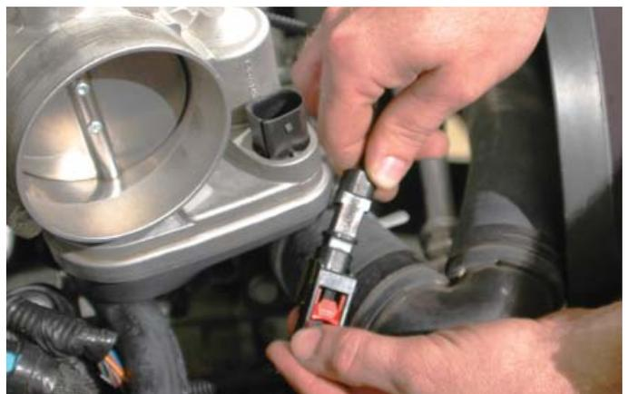
104. Plug in the throttle body connection.
