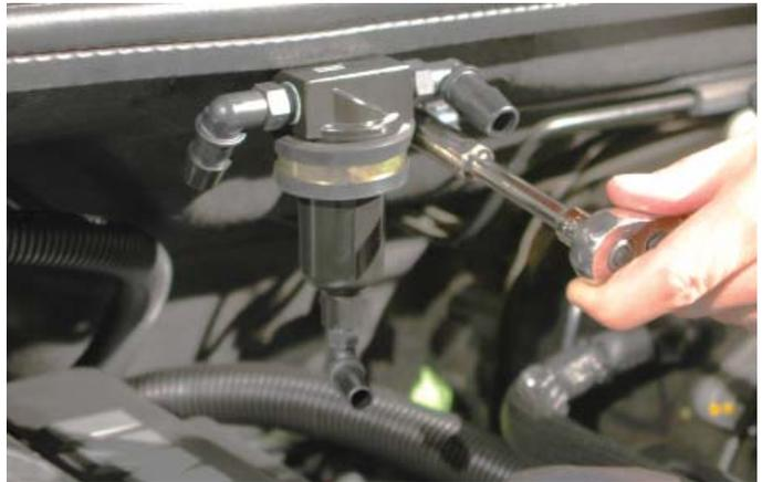
114. Trim the 3/8" hose to fit between the oil separator valve and oil fill spout barb and install between the two, no clamps are necessary.
