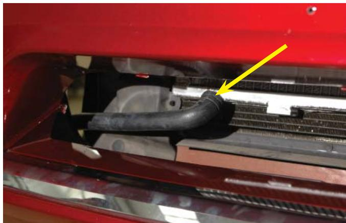
135. Continue to route the hose around the radiator support frame, in and over the lower radiator hose and up into the engine compartment on the right hand side over the coil packs back toward the rear of the vehicle.
