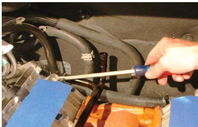
44. Replace the left hand side ground sensor and ground wires to the head using the original stud. Clock the ground sensor toward the left hand side fender to gain the clearance necessary for the supercharger installation.
