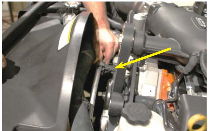
183. Remove the air box end of the hose from the OEM PCV plastic line and replace with the provided 4" section of 5/8" hose. Connect the remaining OEM hose end to the front oil fill spout hose barb and the new hose end to the air box end and air box. Secure to the air box using the provided spring clamp.
