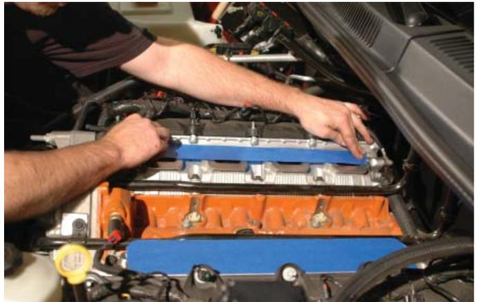
34. Remove the two heater hose clamps from the hard line barbs at the rear of the valley by the firewall, they run over the valley to the water pump.
