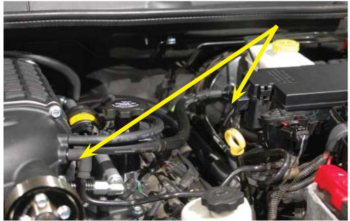
109. Install the fuel line on the new fuel manifold barb at the rear-right hand side fuel rail.
