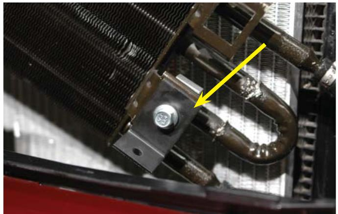
79. Use the provided bolts and nuts to attach the two mounting brackets to the two holes prepared in the top surface of the bumper support. Tighten the bolt and backing plate of the left hand side mounting bracket.
