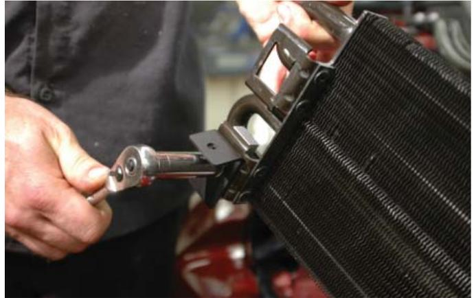
78. Attach the obtuse (greater than 90°) angle mounting bracket to the left hand side lower mounting bracket using the supplied threaded plate with the angle being down leg pointing forward. Finger-tighten the bolt to the backing plate at this time.
