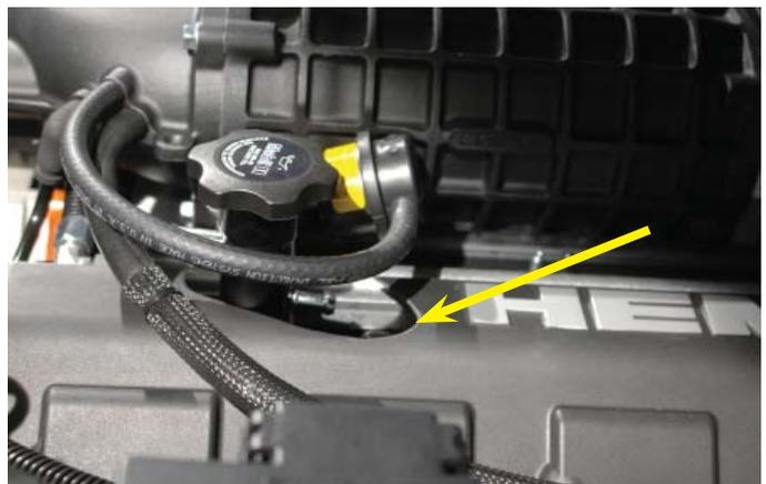
112. On the left hand side below the windshield cross brace is an existing stud pointing down. Use the provided nut to attach the provided bracket to the stud and tighten with a 10mm wrench.
