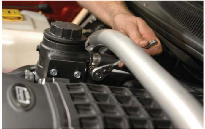
146. Connect the hose from the left hand side barb of the supercharger charge air cooler to meet the hose from the charge air cooler pump inlet barb. Cut the hoses to fit and connect together using the provided coupling (hose mender), and secure in place using the provided spring clamps.
