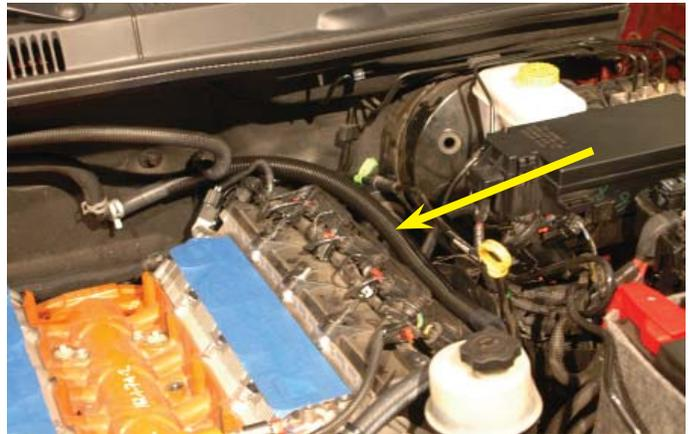
62. Remove the six push pin rivets securing the fascia by prying up the center spreading pin using a flat head screwdriver and then pull the pins out.
