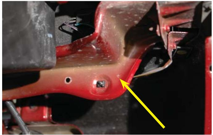
129. Drill a  $\frac{1}{4}$ " hole at the mark for an charge air cooler pump mounting clamp.
