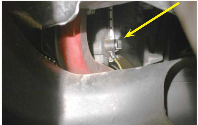
6. Remove the radiator cap to facilitate draining. Upon drainage completion, replace the cap loosely and tighten up the drain valve.
