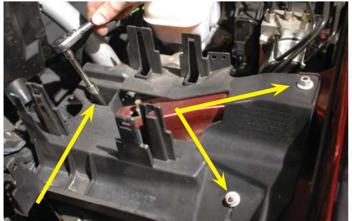
14. You now have access to the left hand side bolts holding the strut tower brace in place. Use an 18mm wrench to remove the nuts securing the strut tower brace in position (two each side). We used an impact wrench but this is not necessary.
