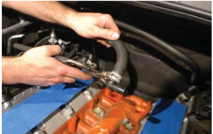
58. Attach the supplied 5/8" x 48" hose to the left hand side barb installed on the water pump using a supplied spring clamp.
