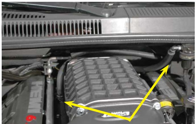
116. Install a 42" piece of the supplied 1/2" hose between the right hand side barb on the supercharger inlet and the left hand side barb of the oil separator valve.
