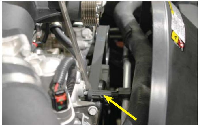
170. Use a 3/8" socket or breaker bar to spring the tensioner to remove the factory drive belt. **We used a piece of pipe over a ratchet to gain leverage.**
