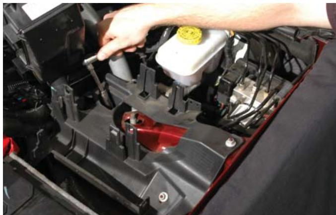
119. Re-connect the two forward fuse center plug connections.
