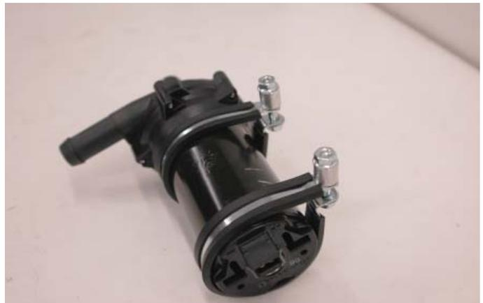
131. Secure the pump as described using the supplied nuts on the rear side of the fender cross brace. The discharge barb of the pump is to point down with the inlet barb of the pump pointing toward the left hand side of the vehicle. Tighten in place using a 10mm wrench.
