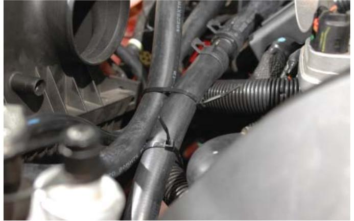
149. This is the charge air cooler pump relay harness. Install the provided 15A fuse in the fuse holder of the harness and replace the fuse cap.
