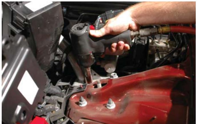
15. Pull up on the strut tower brace to pull it off the studs. On the left hand side, the mounting flange will hit the bottom of the brake cylinder. Pull the brace completely off the right hand side, and angle the brace to the rear to gain clearance to further pull the strut tower brace from the vehicle. Set aside for later use.
