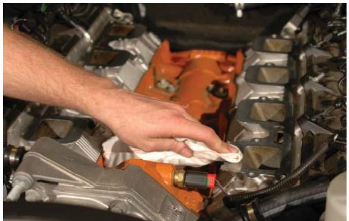
99. With the help of an assistant, set the supercharger assembly in place. Be careful with the protruding bolts and the IAT sensor harness wires which must exit below the assembly toward the front of the supercharger on the right hand side.
