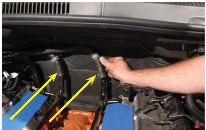
36. Use a 10mm wrench to remove the nuts holding the ground wires and ground sensor from the studs anchoring the heater hard lines to the back of the block. There are ground wires on both the left hand side and right hand side. Pull these wires and the ground sensor from their studs.
