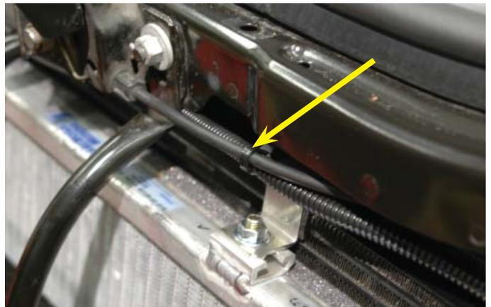
152. Connect the charge air cooler relay harness plug to the receptacle on the charge air cooler pump.
