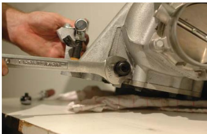
83. Install the PCV valve in the right hand side hole of the supercharger lid and tighten with 15/16" wrench.
