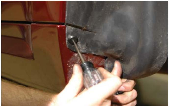
127. Remove the splash shield fender well from the vehicle and set aside to re-install later.
