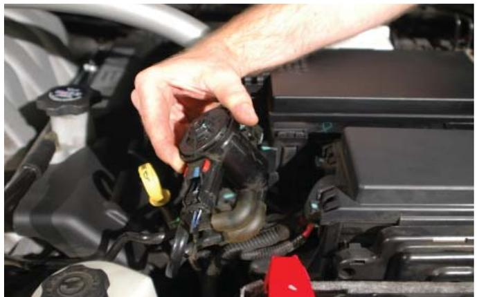
8. Open the cover of the forward fuse center just behind the battery on the left hand side of the engine compartment, and un-snap the hinges from their posts to remove the cover. Set aside for later usage.
