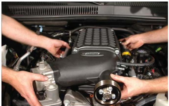
100. Torque the supercharger mounting bolts to 106" lbs. using a center-out, crisscross pattern. Verify your torque wrench settings.
