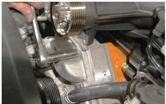
172. Loosen the tensioner assembly using a 15mm wrench. **This does not need to be removed just loosened enough to remove the next bolt.**
