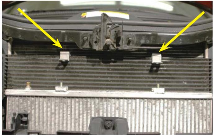
73. Slide the charge air cooler low temperature radiator up and secure to the located mounting brackets using the provided nuts.
