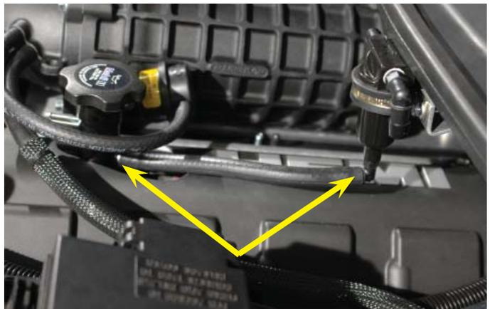
115. Install a 24" piece of the supplied 1/2" hose between the right hand side PCV barb in the supercharger lid and the right hand side barb of the oil separator valve.
