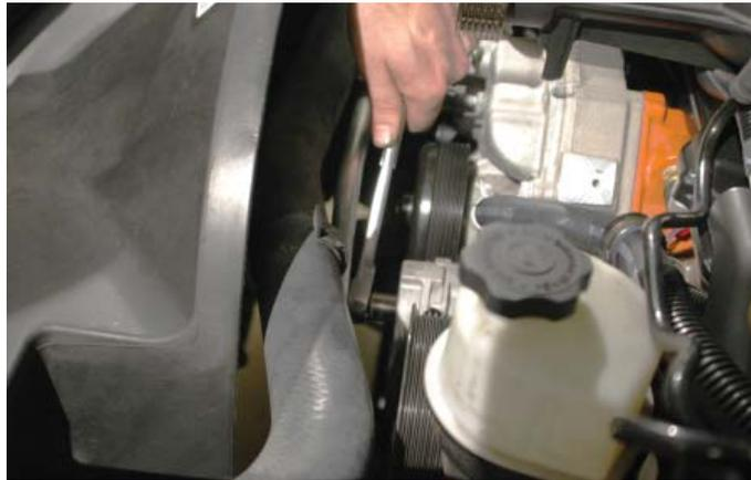
173. Going clockwise (toward the left hand side) from the first water pump bolt, skip one, then using a 13mm wrench remove the next bolt. **You may need to rotate the tensioner assembly to pull the bolt free.**
