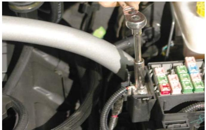
155. Remove the 25A fuse #43 for the **fuel pump** from the rear fuse center. Verify using the owner's manual that you are removing the coil-actuators fuse. **Do not rely on just the fuse number specified, verify by name.**
