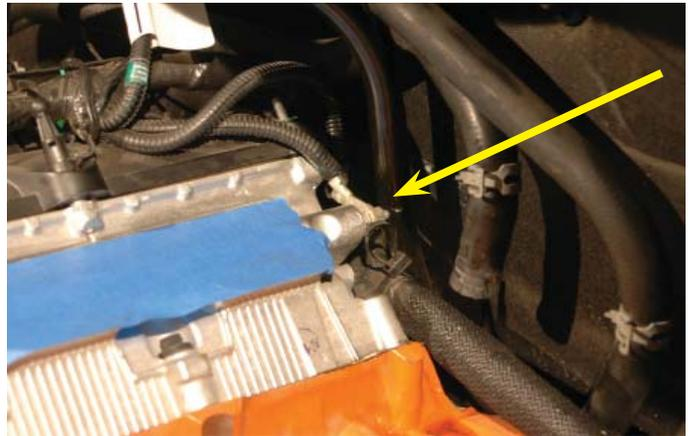
46. Place a generous bead of the supplied Green Loctite on the two supplied water pump hose barbs.
