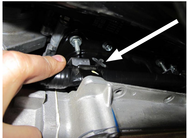
Fig. 12-b: Oil Drain Fitting Installation Location
