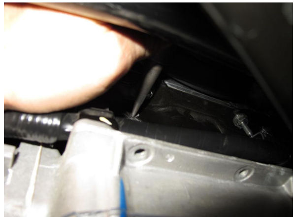
Fig. 12-d: Punching Hole in Oil Pan
