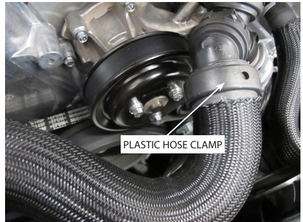
Fig. 7-b: Cut Plastic Hose Clamp
