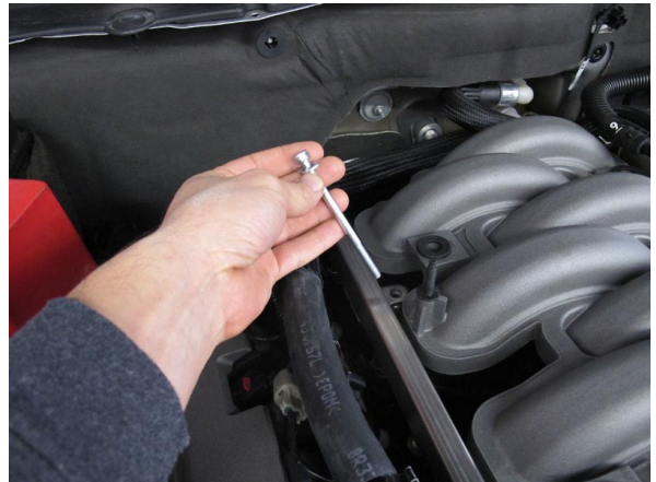
Fig. 6-m: Re-securing Fuel Rails
