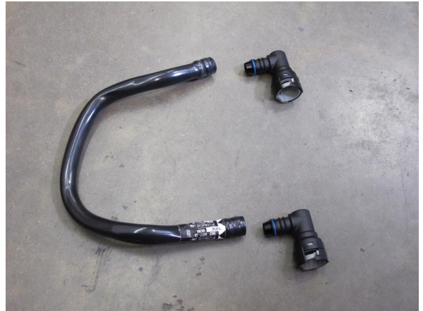
Fig. 4-a: OEM Passenger Side PCV Hose with fittings removed
