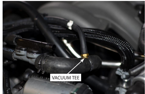
Fig. 9-b: Vacuum Tee Installation
