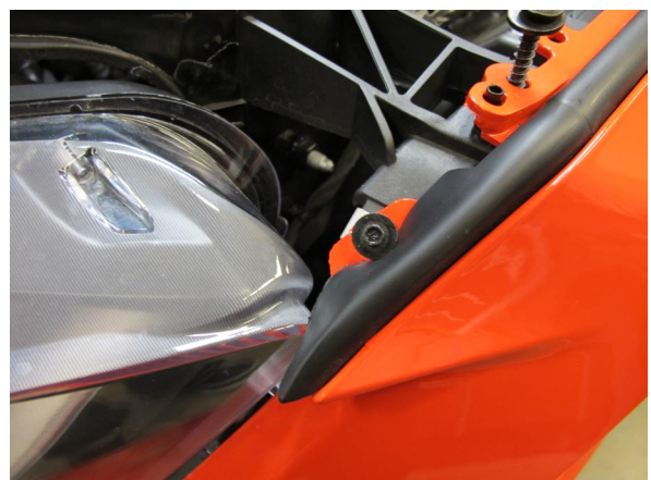
Fig. 1-c: Remove 5.5mm-Headed Fastener
