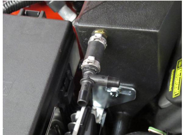
Fig. 7-i: \text{\O}3/8'' \times 2'' Hose
