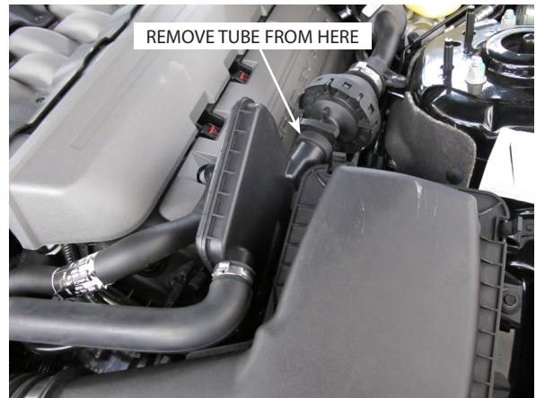
Fig. 1-n: Remove Interior Sound Tube
