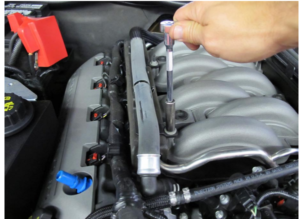
Fig. 6-b: Hose Guide Removal
