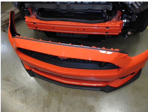
Fig. 1-h: Front Bumper Cover Removed
