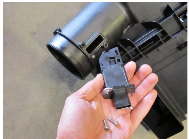
Fig. 1-s: MAF Insert (shown with OEM airbox removed)
