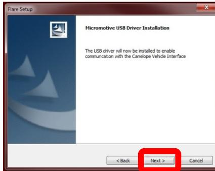
11. Device Driver window should pop up for installation of the USB drivers. Select **"NEXT"**.
