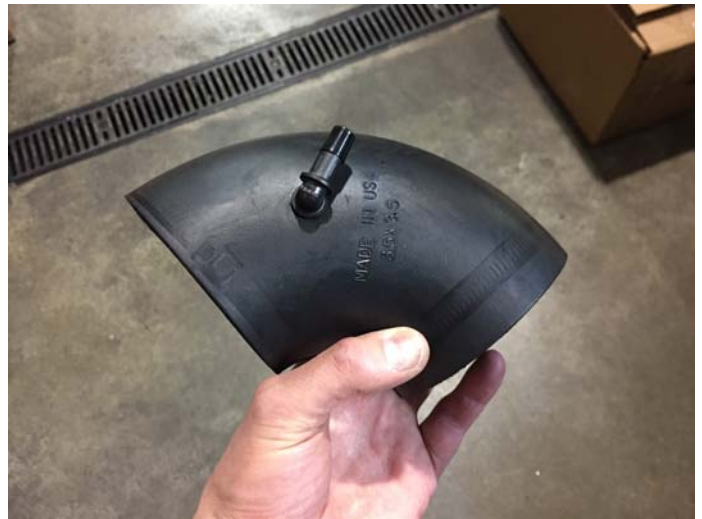
90° Plastic Barb Fitting Installed
