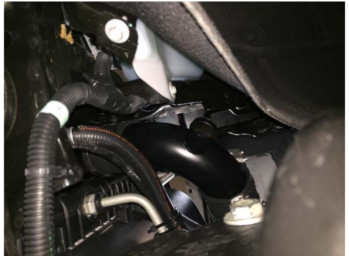
Surge Tube (From Bottom Side)
