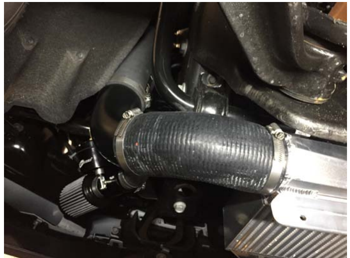
Tubing To Intercooler Installed
