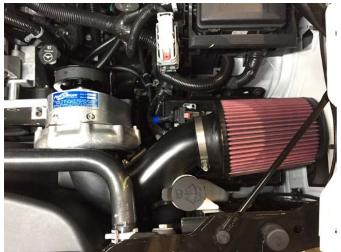
Air Inlet Installed
