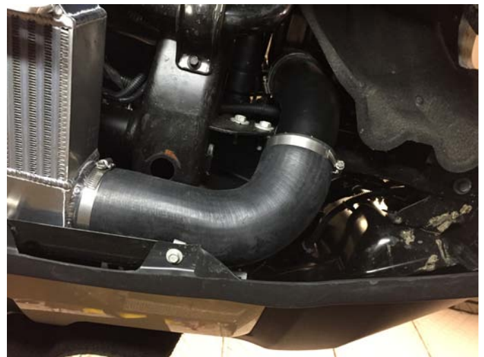
Tubing Out Of Intercooler Installed
