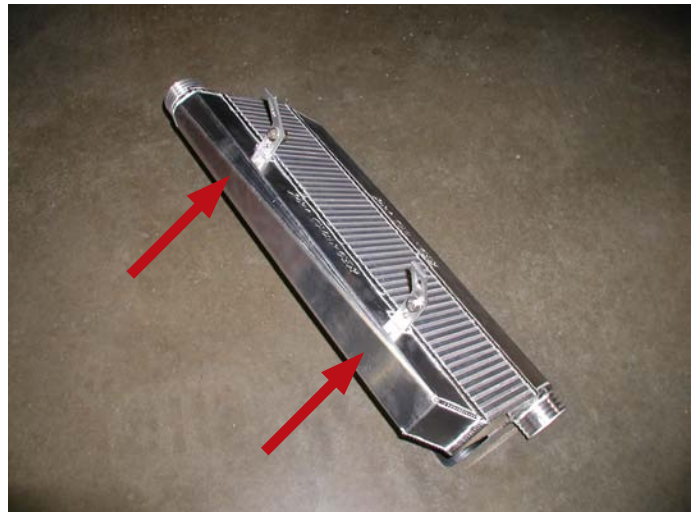
Front Intercooler Tabs Installed
