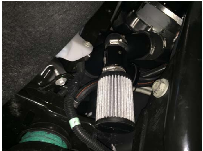
Surge Valve Installed (Vertical Intercooler)
