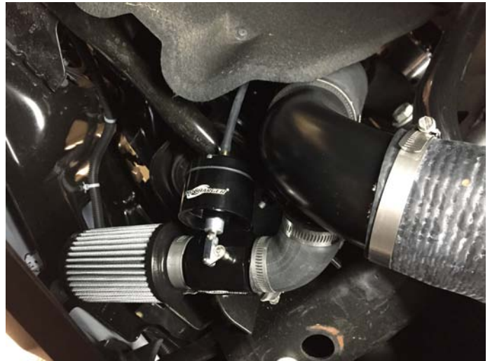
Surge Valve Installed (Horizontal Intercooler)
