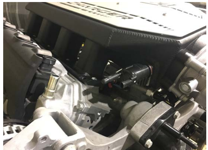
EVAP Cylinder Installed
