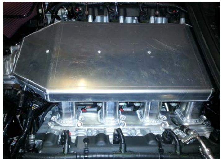
Intake Manifold Installed
