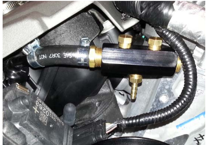
Vacuum Manifold Top Port Installed
