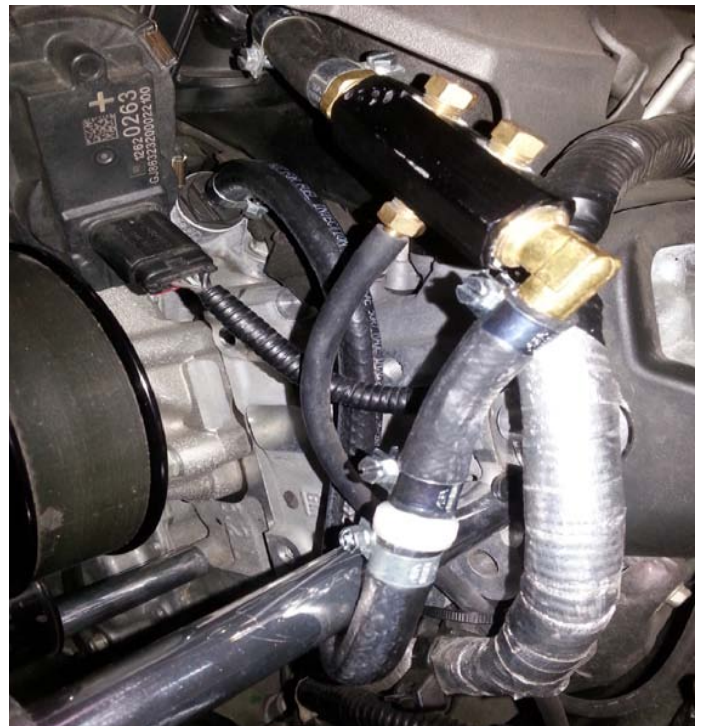
Vacuum Manifold Installed
