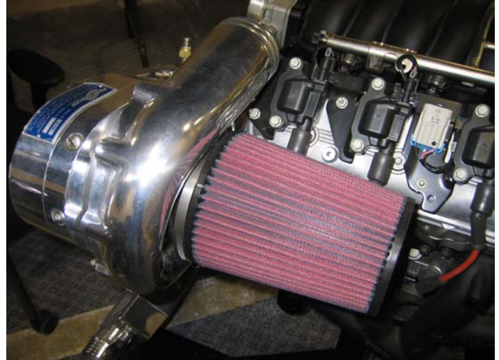
Air Filter Installed
