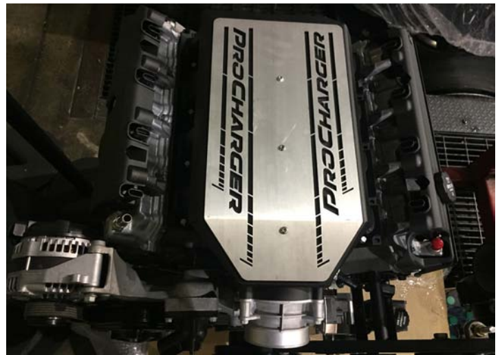
Intake Cover Installed
