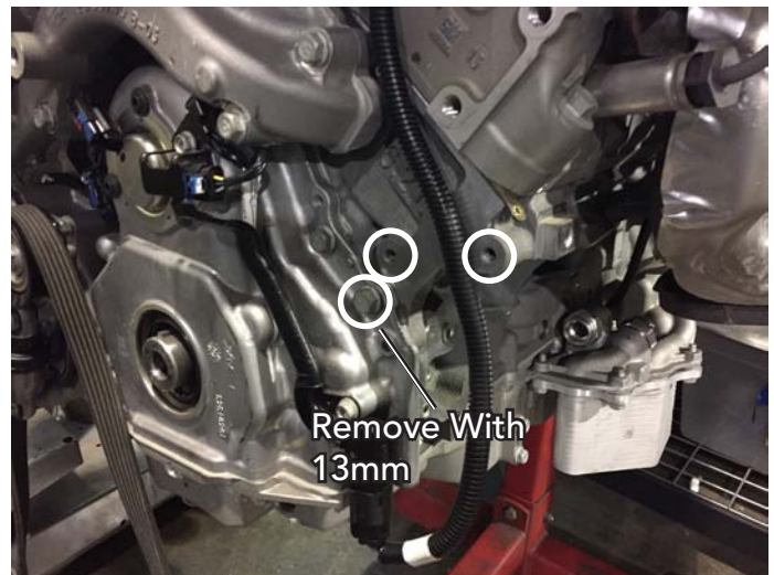
Power Steering Sub-Bracket Mounting Holes
