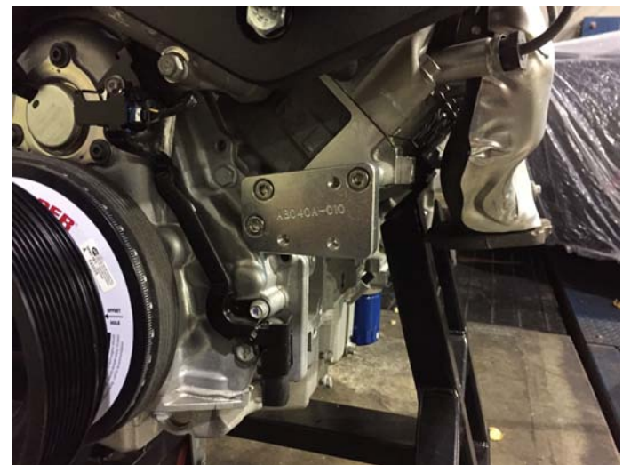
Power Steering Sub-Bracket Mounted
