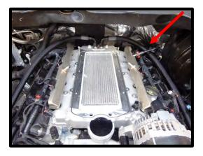
67. Install (2) of the supplied ½" rubber grommets to the LTR bracket. Apply light amount of grease in the ID of grommet. Install the LTR bracket to the factory frame using the (2) 6mm x 20mm HHFCS. Torque to 106 in-lbs.
