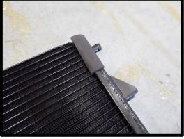
70. Carefully slide the LTR down in between the condenser and core support. LTR pins will sit in rubber grommets. Driver side fitting is down, passenger side is up at the top.
