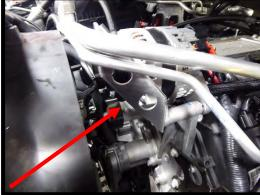
46. Reconnect power wire and electrical connector. Push plastic clip for power wire protection back in place.
