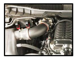
103. (Stock air box) Connect the supplied 3/4" x 11" hose and 3/4" to 5/8" adapter to the pre-routed oil fill barb fitting. Connect hose to factory airbox.
