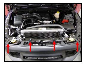
8. (Grill detachment varies per model) Earlier model years will detach (2) metal retaining clips and (2) plastic retaining clips. Later model years will detach (1) center tab and (4) plastic push pins. Detach grill appropriately and remove.
