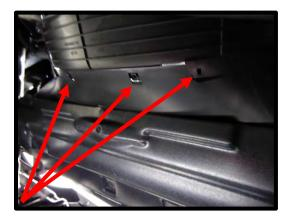
33. Using a panel puller, detach the splash guard from the fan shroud (push pins do not have to be removed).
