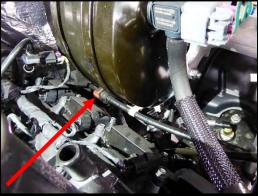
16. (EVAP mounted on intake manifold) Unplug the EVAP connector and disconnect the second EVAP hose from solenoid. Remove the EVAP solenoid from the manifold and set aside as it will be reused later.
