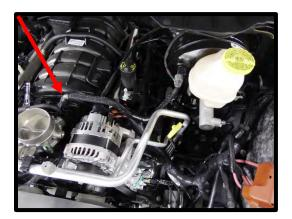
18. Using a small flat head screwdriver, remove the AC support strap from the A/C lines (this will be reused). Unthread this from the bracket.
