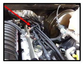
92. Install the supplied (3) 9.89mm to 6an oring fitting to the SC inlet.
