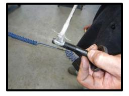
44. (Complete kits) Remove the (8) coil electrical connectors. Remove the coils using a 10mm socket and ratchet (2 bolts per coil). Lift the coil out and use a 5/8" spark plug socket and ratchet to remove the stock spark plugs (16). GAP TO .028". Apply light amount of anti-seize and reinstall. Torque to 13 ft-lbs.
