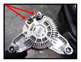
30. Using a 15mm socket, unbolt alternator and remove from engine.
