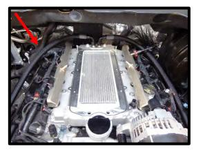
66. Install the 5/8" x 34" intercooler hose to the driver side intercooler fitting. Secure to fitting and route along the driver side valve cover to the driver side of radiator for later installation.
