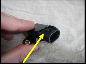
50. Apply generous amount of grease to the supplied 2-BAR MAP sensor oring. Install the supplied MAP sensor to the back of the lower intake manifold by lightly pressing the oring barb through the .590" passage on the back of the lower intake manifold. Use the supplied 5mm x 16mm SHCS (2) bolts to secure sensor to lower manifold. Torque to 50 in/lbs.
