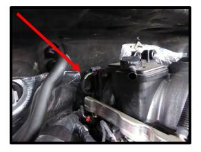
24. Disconnect fuel pressure sensor where applicable (not all models have this).
