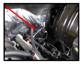
25. **WARNING!!** Disconnect factory fuel feed line from fuel rail. Early model years, remove the fuel safety clip from the fuel feed line then disconnect the fuel feed line from the fuel rail using a 3/8" fuel line removal tool. Later model years need to lift up the red locking tab and then depress the red locking tab from both sides to remove fuel line. Cap the fuel rail to avoid excess fuel spillage.
