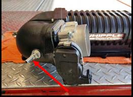
93. (Stock fuel rails) Connect other end of fuel line to the passenger side fuel rail barb. Apply grease or silicone to hose ends for easier installation. You may also use a heat gun on the hose prior to installing (away from any fuel vapors) to make the hose more flexible. Secure with safety clamp.
