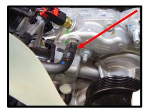
62. Remove the (3) factory fasteners at the water pump assembly using a 13mm and 15mm socket. Install the supplied idler assembly to this location. The idler plate and stand are each marked to their respective position. Use the 8mm x 130mm SHCS on the passenger side bolt hole with the .4525" spacer, 8mm x 140mm SHCS on the center hole with the 1.675" spacer, the 10mm x 55mm SHCS with the .865" spacer. Torque the 8mm bolts to 22 ft-lbs and the 10mm 45 ft-lbs.
