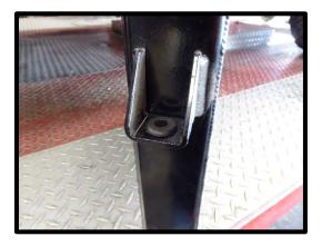
69. Install the supplied (2) 4" long foam strip vertically on the inlet and outlet tank of the LTR, at the top. Cut the 3<sup>rd</sup> 4" foam strip into (2) 2" pieces. Flip the LTR over and install on the top inlet and outlet tank of the LTR. Install the (2) supplied ½" rubber grommets to the LTR mounting brackets. Apply light amount of grease in the ID of grommet.
