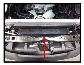
71. Using a 10mm socket, remove the (2) factory hex bolts securing condenser to radiator on driver side. Install the supplied LTR bracket by sliding the locating pin into the LTR grommet. Secure with factory bolts.
