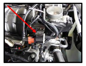
17. Remove brake booster hose from intake manifold. This hose will be reused.
