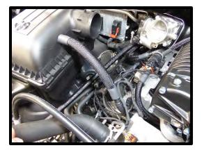
104. (Whipple CAI systems) Using a 1" drill bit, drill a hole in the boss of the air tube. Install the supplied 1" to 3/4" ID rubber grommet. Install the supplied 3/4" to 5/8" barb fitting into air tube. Connect pre-routed hose to air tube.
