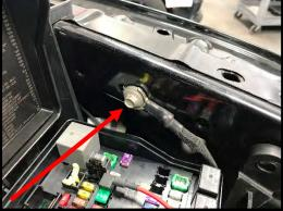
83. Route the turn on wire (orange) through the fuse box. In some cases, a notch may be required for the wire to fit through the fuse box (make sure wire cannot not be cut or chaffed). Remove the fuse from location #70 (fuel pump). Install this into the fuse tap. Install the fuse tap (should have the 30amp and 10amp fuses) into location #70. Route the pump 4-way connector to the driver side front fender for connection to the IC pump.
