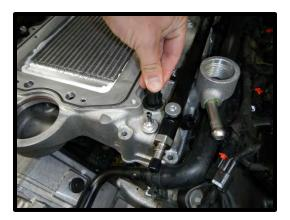
48. Install the supplied PCV valve into the intake manifold, passenger side.
