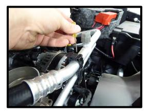
19. Using a panel puller, remove the (2) push pins securing wiring harness to A/C line support bracket and (1) secured to intake manifold.
