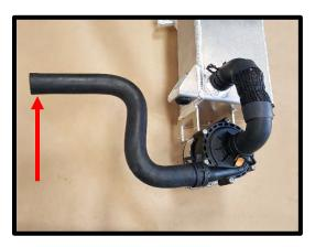
74. Install the IC pump to the IC reservoir by installing the supplied clamp and rubber strip (leave slightly loose to position after hose installation). Once pump is in position, tighten clamp.
