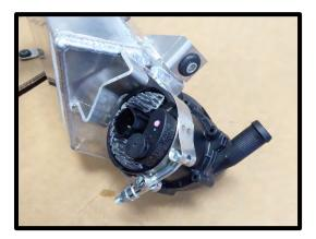
75. Install the supplied (3) rubber grommets into the 3 mounting flanges of the IC coolant reservoir.
