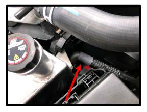
82. Install the IC pump relay harness. Connect the 12V and ground eyelets to the factory positions as shown.
