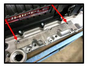
90. (Stock fuel rails) Secure stock fuel rails to fuel rail brackets using the (4) 6mm x 12mm. Torque to 106 in-lbs.
