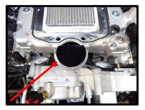
59. Install the factory 1/2" hose 90deg to the oil fill barb. Route hose under the front of the manifold and between water pump housing and block. Leave on passenger side of valve cover for later installation to airbox.
