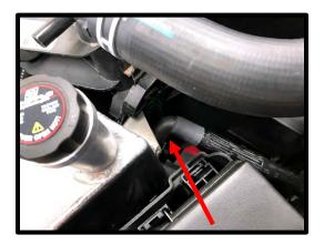
80. Install the previously installed S bend hose from the LTR driver side barb fitting to the IC pump outlet fitting. Secure both ends with pinch clamps (image shown off vehicle for better view).
