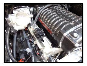
98. Install the supplied brake booster 3/8" 90deg quick connect fitting to the end of the factory brake booster hose. Connect hose to the front driver side 9.89mm fitting.
