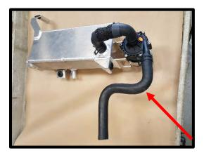
81. Secure pre-routed passenger side IC fitting to passenger side LTR fitting. Secure with pinch clamp. Ensure that hose cannot bind while routed through condenser lines.
