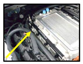
49. Modify the supplied 2-bar MAP sensor (PN# 1-05033224AB) by carefully removing the factory tang. It's best to use a box cutter/razor or a Dremel tool.
