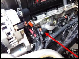
60. Using a razor blade, carefully cut the factory EVAP quick connect fittings from the factory hose. Install these into the supplied ½" x 39 ½" hose. Route this hose with the straight fitting going to the passenger side of vehicle between the front of the manifold and water pump/alternator assembly for later installation.
