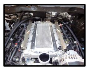
91. (Stock fuel rails) Reconnect factory fuel feed line to fuel rail.
