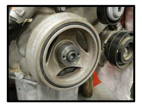
41. Use the supplied 1/4" drill bit (it has a stop at roughly 2.875" from drill bit tip), drill 2 holes into the crankshaft thru the (2) holes in the pin adapter. Blow off debris when done drilling. Remove the pin adapter using an adjustable wrench.
