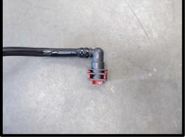
61. (When applicable) Rotate the hose clamp for the thermostat vent line away from center so it doesn't interfere with the idler pulley.
