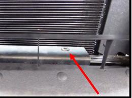
68. Install the supplied (2) rubber grommets into the LTR brackets. Apply light amount of grease to ID for easy installation.
