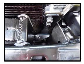
72. Using a phillips screw driver, remove the (2) factory hex bolts securing condenser to radiator on passenger side. Install the supplied LTR bracket by sliding the locating pin into the LTR grommet. Secure with factory bolts using a phillips screw driver.
