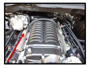
94. The supercharger must be filled with oil prior to use. This supercharger is shipped without oil inside. The oil is in a separate bottle supplied with your kit. The bottle is pre-filled to the exact amount required (5.8 fl/oz.).
