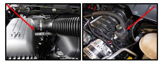
13. Remove the passenger side PCV hose from barb under throttle body and barb at back of intake manifold.
